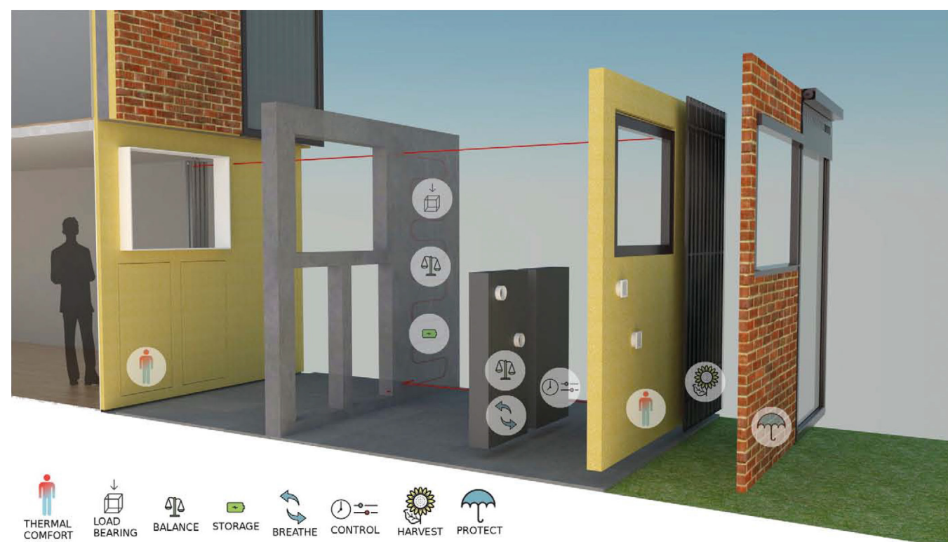
Figure 28: Overview of the ADAPTIWALL project and arrangement of layers Source: www.adaptiwall.eu
