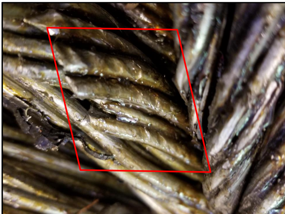
Figure 4.23 - Local contact deformations on outside strand wires of 77 mm 6x36WS-IWRC sling after bending test.
