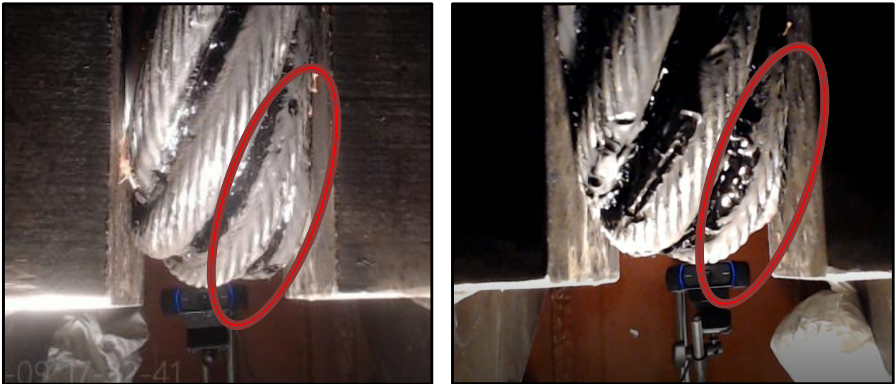
Figure 4.22 – West (left) and east (right) elevation views of the rope bending around the pin.
