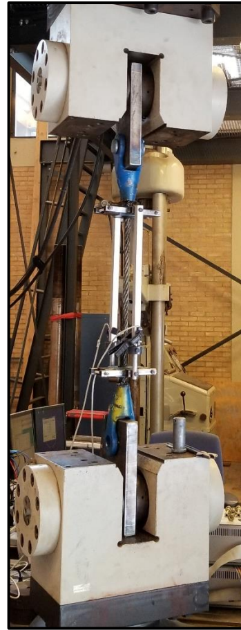
Figure 4.2 – Proof load test setup for small-scale experiment.
