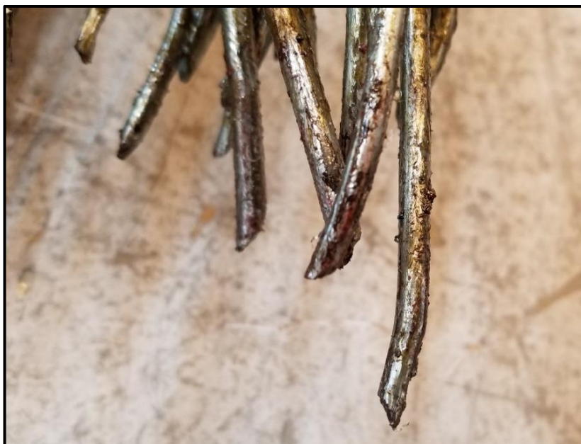
Figure 4.21 - Typical shear failure mode of wires after full-scale bending test.
