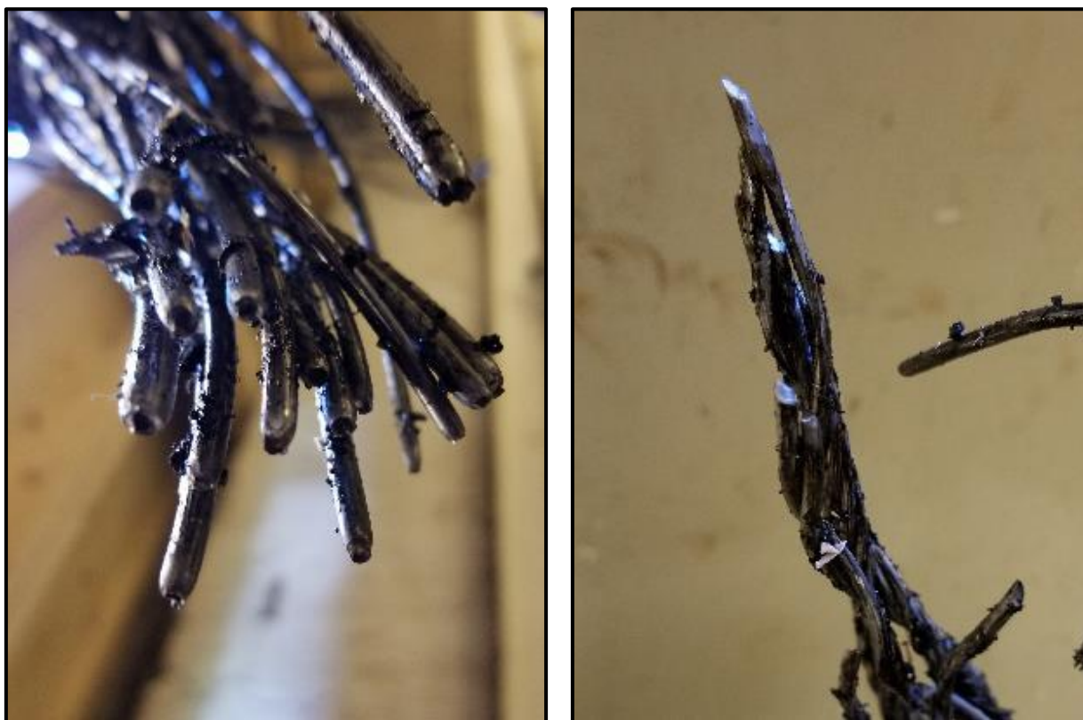
Figure 4.14 - Typical failure mode of outer strand wires due to necking (a) and core wires due to shear (b).
