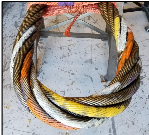
Figure 4.19 - Spray paint technique applied to outer strands near bend of 77 mm 6x36WS-IWRC sling.
