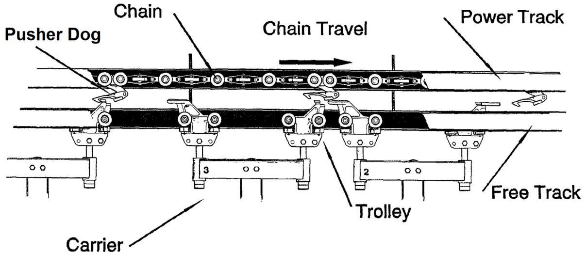
Figure 1.3: Working principle power & free conveyor [15]
