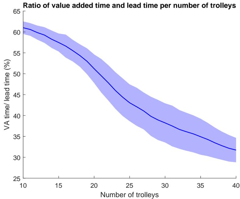
Figure 5.3: Ratio of value added time and lead time per number of trolleys for the current state scenario
