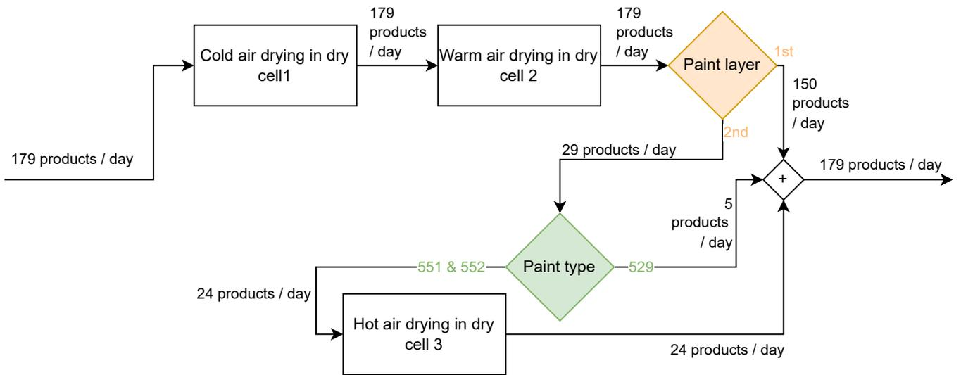
Figure 3.4: The drying tasks performed by 3 dry cells based on latest paint layer and paint type.
