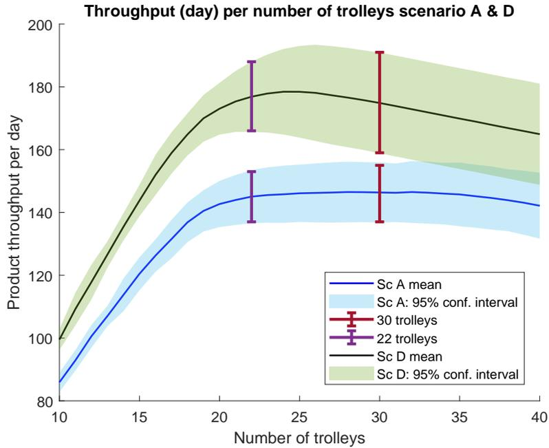
Figure 5.7: Throughput per number of trolleys for scenario A and D
