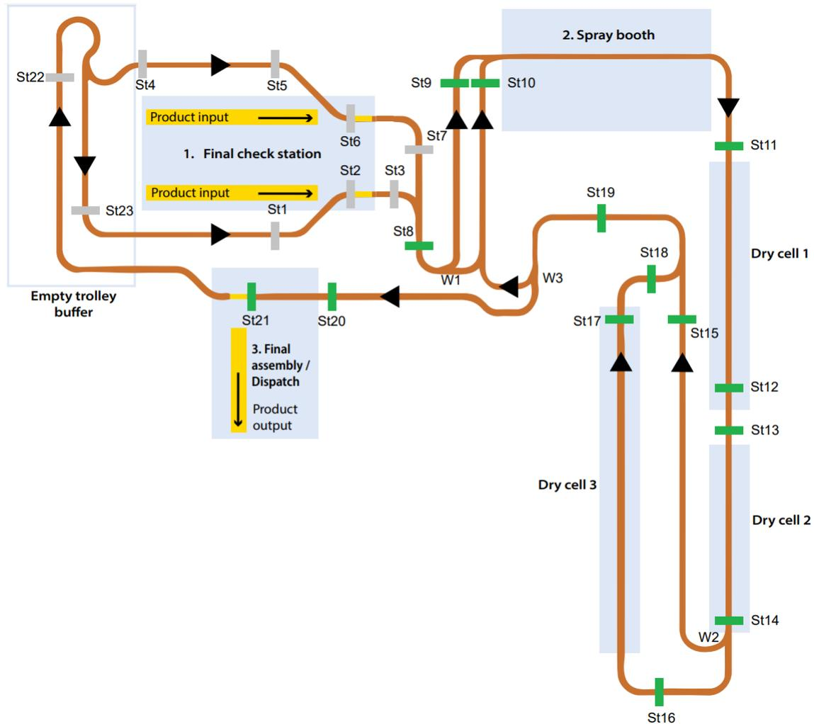
Figure 6.3: Locations of the current sensors at stoppers that record data in green. The same sensor data is required for stoppers marked grey for the development of a digital twin.
