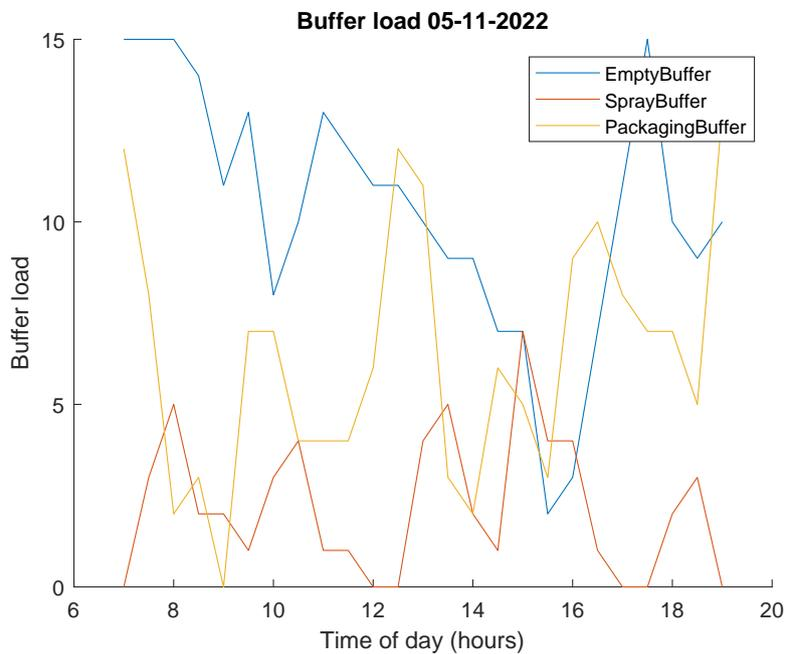
Figure 1.5: Buffer lengths of the P&F system for an arbitrary day in May 2022 with a resolution of 30 minutes. The empty trolley buffer refers to the sum of stopper 22,23,1,4 and 5. Spray buffer to the sum of stopper 9 and 10. Packaging buffer to the sum of stopper 20,19,18 and 15. This figure shows the problem of appearing, disappearing and varying buffer lengths.
