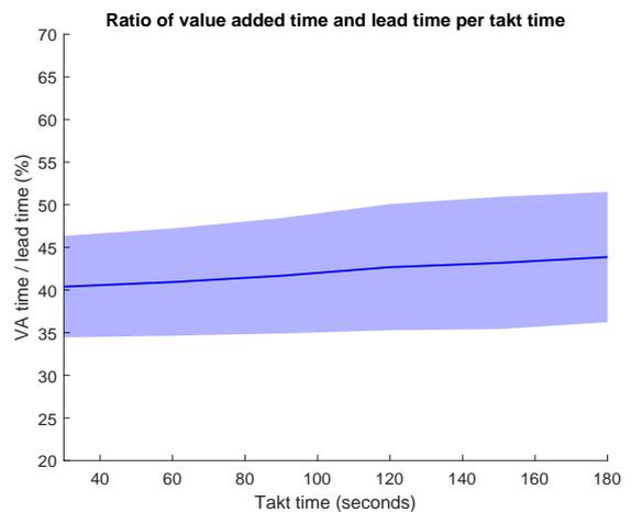
Figure 11: Ratio of value added time and lead time for different takt times
