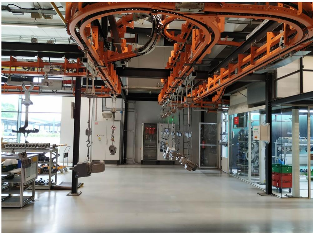
Figure 1.2: Part of the Power and Free conveyor at SEW Eurodrive Rotterdam
