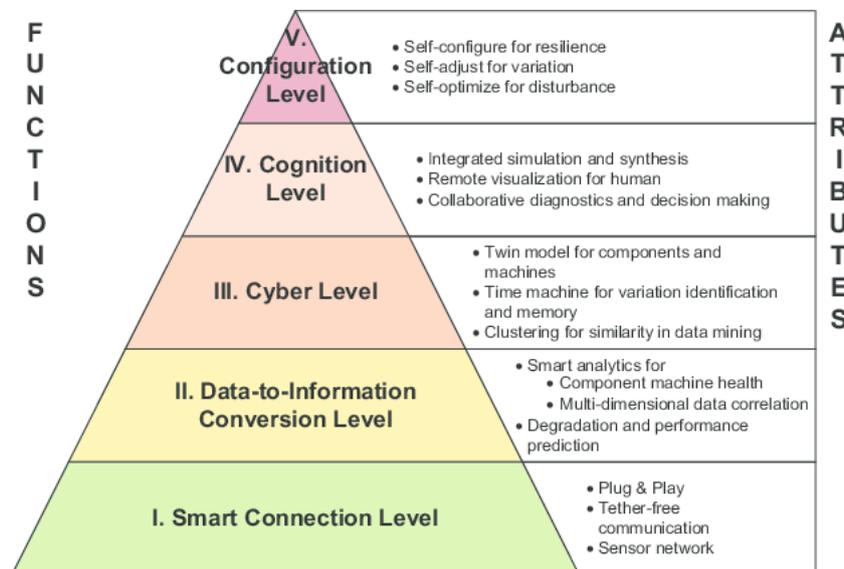
Figure 2.2: Architecture of a cyber-physical production system [51]
