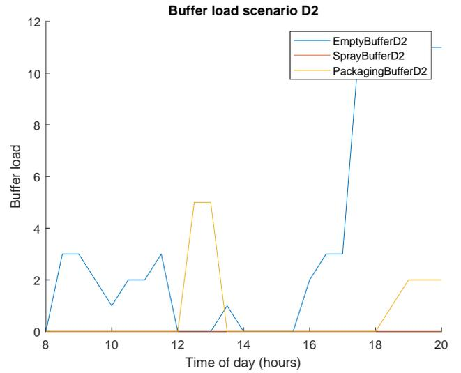
Figure 8.27: Model output buffer load scenario D2
