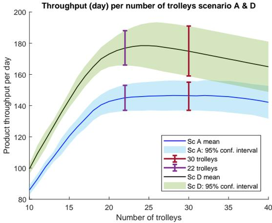
Figure 12: Throughput per number of trolleys for scenario A and D
