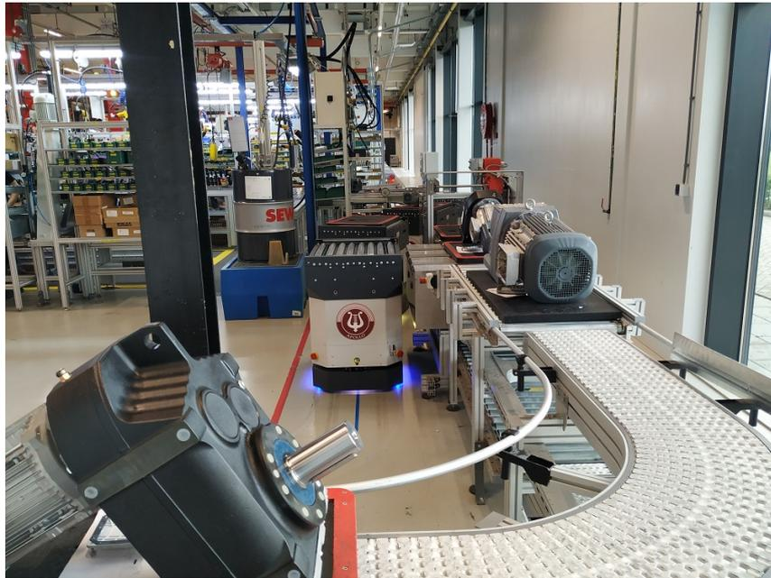
Figure 1.1: Products are transported on dedicated plates in a one-piece flow
