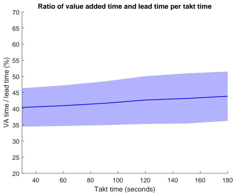
Figure 5.6: Ratio of value added time and lead time for different takt times at the final check station
