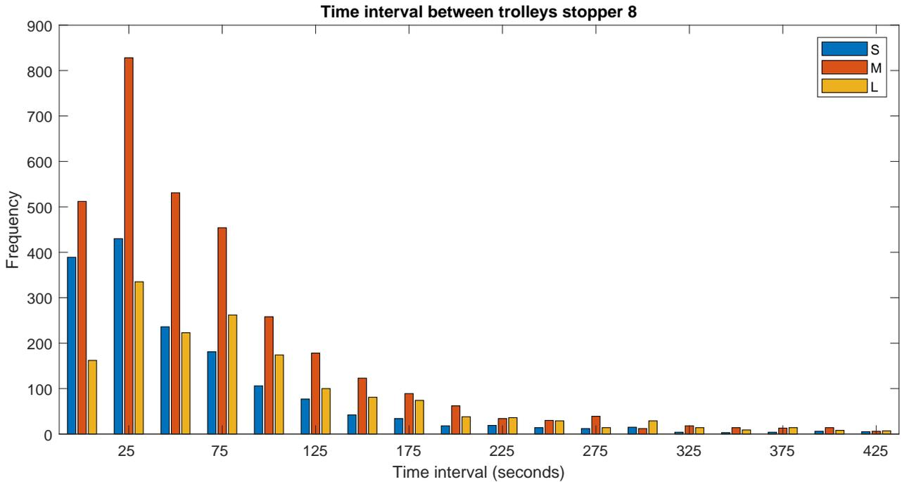
Figure 3.7: Time intervals between trolleys at stopper 8 for different size categories
