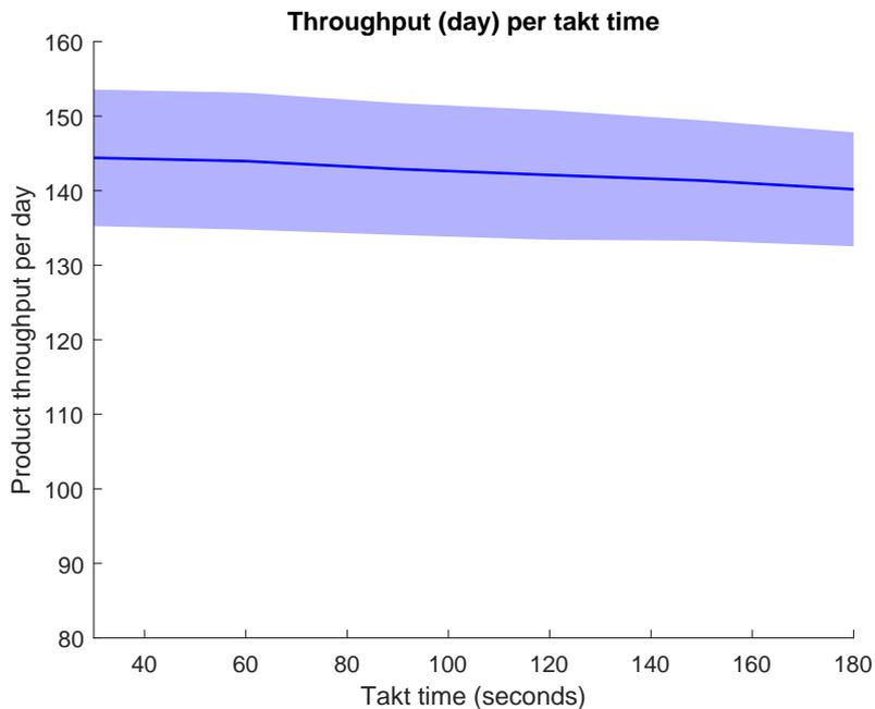
Figure 5.4: Throughput for different takt times at the final check station
