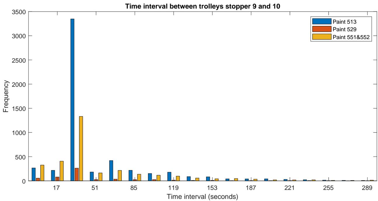
Figure 3.9: Time intervals between trolleys at stopper 9&10 for different paint types
