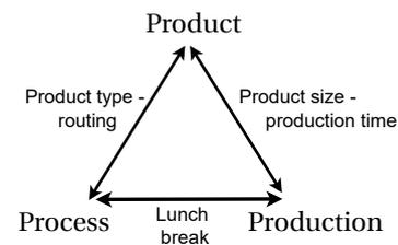
Figure 5: 3P model, three perspectives on a production system, each one influencing the other two [1], in this research used to assess variability.
