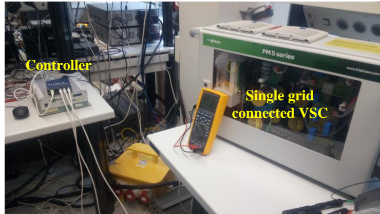
Figure 3.46: Experimental setup showing a single grid connected VSC operating as a STATCOM under distorted voltage.
