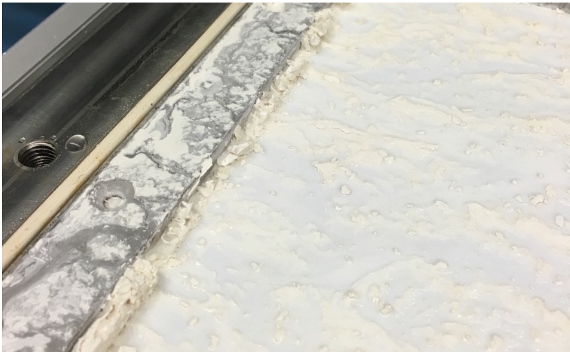
Figure 4.10: Accumulation of CaCO 3 deposits near the inlets of the pressure vessel after conclusion of experiment 4
