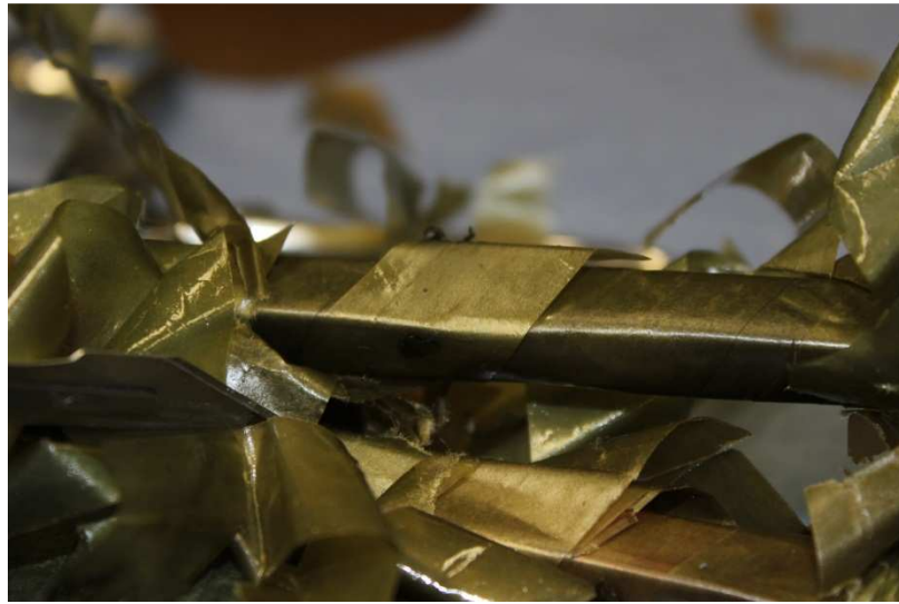
Figure 2.9 Breakdown path example with two breakdown channels.
