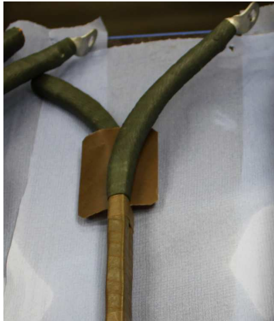
Figure 3.5 CTC winding sample with extra insulation required at the bend of winding samples.
