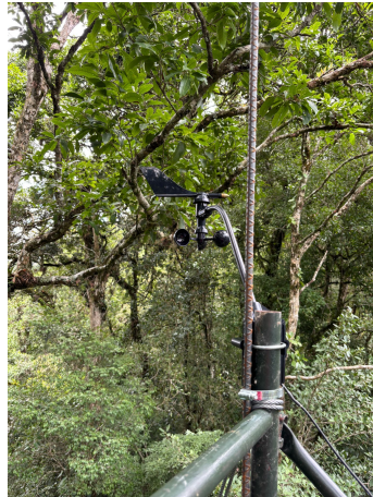
Figure 34: The wind speed and direction sensor, installed at 13.5 meters (only one sensor installed)
