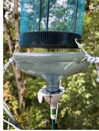
Figure 30: The connection of the fogtrap to the hose leading the collected water to the tipping bucket. A combination of funnels was used
