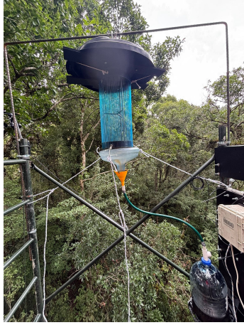
Figure 29: One of the two fogtraps installed at the top of the tower, including the connection to the tipping bucket which is in its turn connected to the data logger
