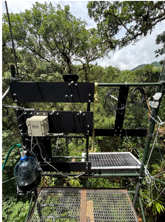
Figure 27: The installation at 13.5 meters, including the data logger (beige box) and solar panel
