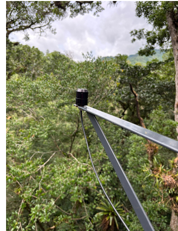
Figure 35: The solar sensor installed at 13.5 meters (2 meter sensor not shown), including attachment arm
