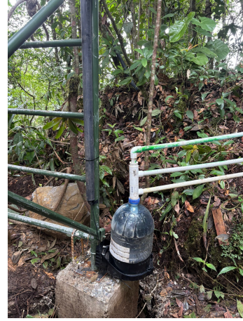
Figure 32: The tipping bucket at the base of the tower, collecting the water from the throughfall set-up
