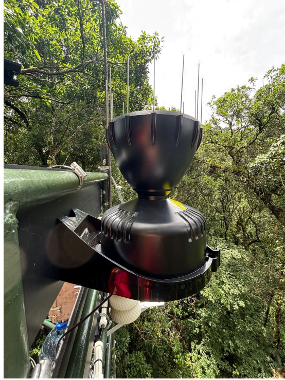
Figure 28: The tipping bucket installed at 13.5 meter height, serving to monitor the vertical precipitation
