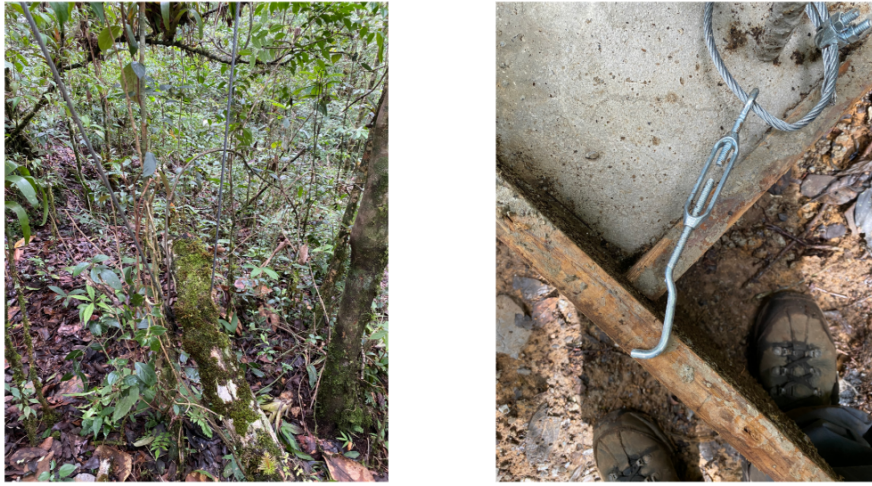
Figure 42: Example of failed tensioner during storm as input for maintenance plan (Cloud Chasers IV, 2025)
