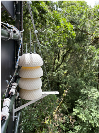
Figure 33: The temperature/relative humidity sensor, installed at 13.5 meters (2 meter sensor not shown)
