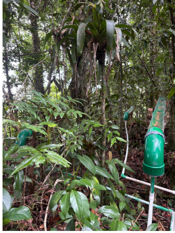
Figure 31: An overview of the three PVC gutters, randomly positioned, used for the throughfall set-up
