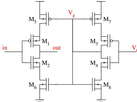
Figure 4.42: Threshold compensated inverter [72]
