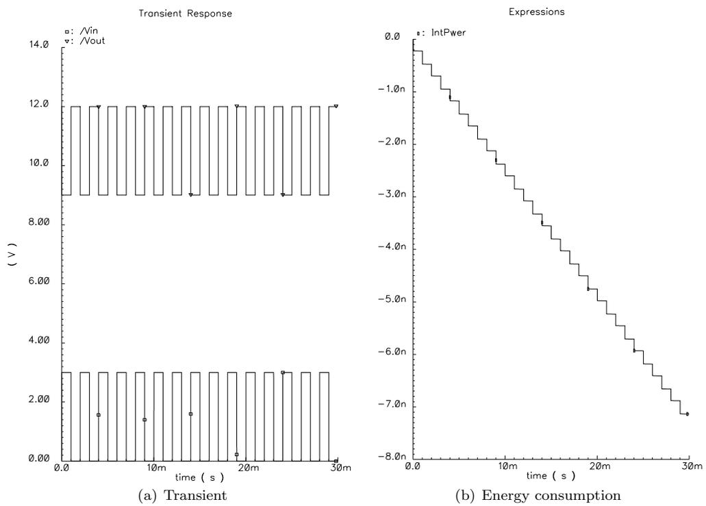
Figure 5.2: Simulation results of the level converter based level shifter
