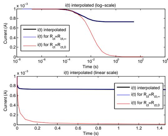
Figure 3.20: Plot of the interpolated step response with denormalized time scale
