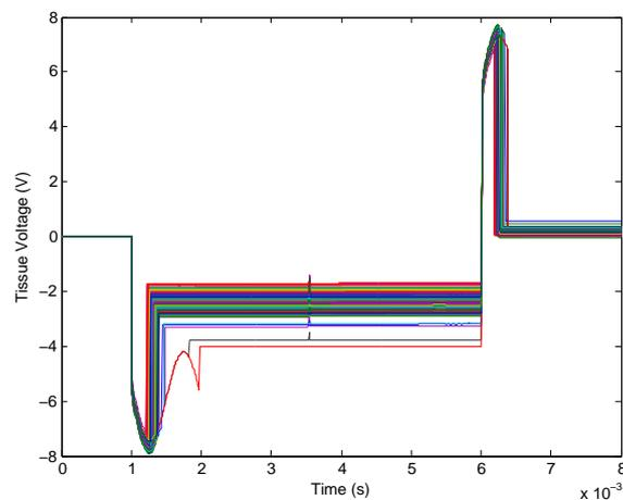
Figure 5.34: 100 run Monte Carlo simulation of the stimulator
