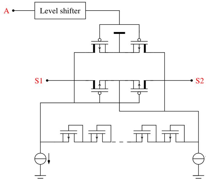
Figure 4.47: Final implementation of the switch
