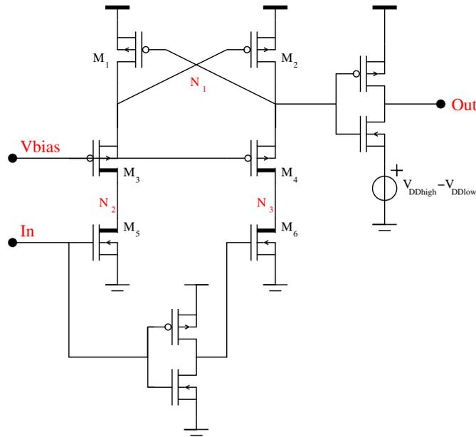
Figure 4.7: Design of a Level Shifter based on a Level Converter
