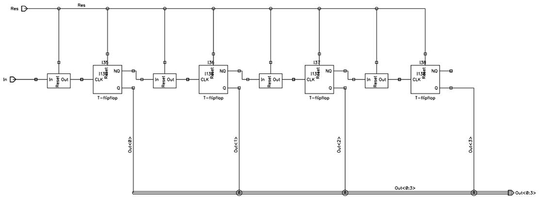
Figure 5.21: Implementation of the counter in the testbench
