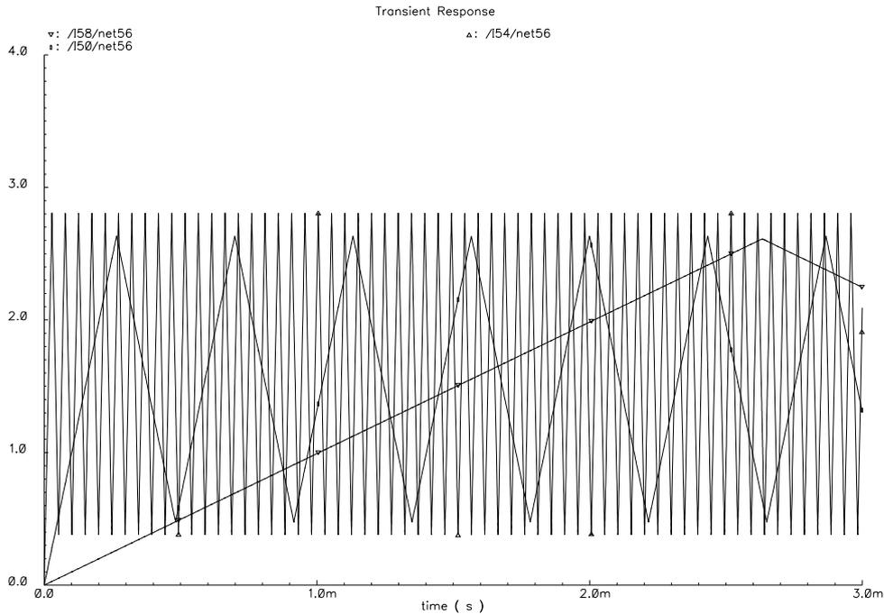
Figure 4.40: Capacitor voltages in the integrator using three DC current inputs
