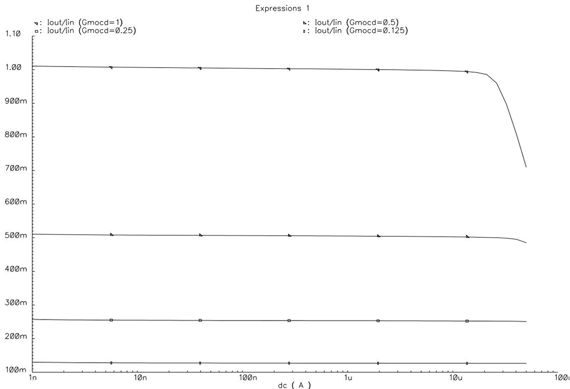
Figure 5.10: MOCD current gain using a buffered output stage with adaptive bias
