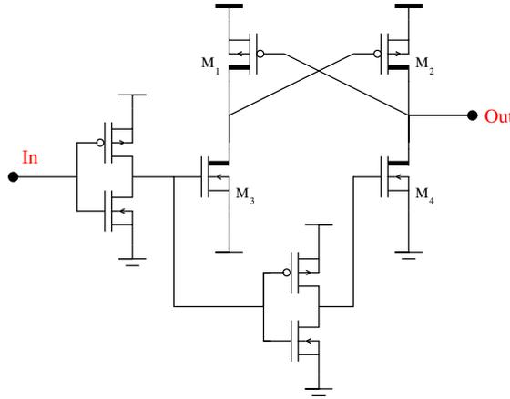
Figure 4.6: A conventional Level Converter circuit
