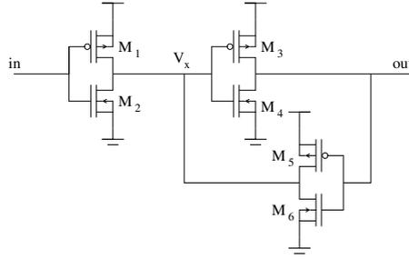
Figure 4.41: Inverter based Schmitt trigger
