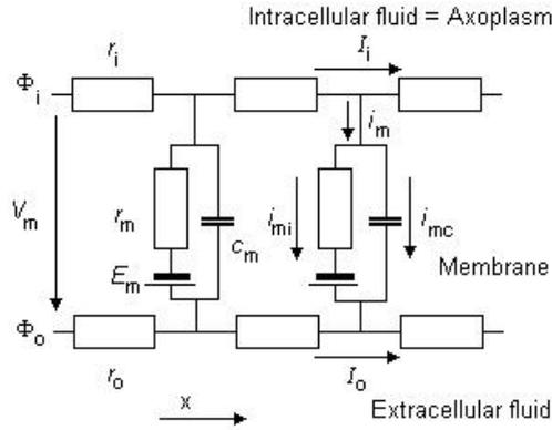
Figure 1.8: Membrane model for subthreshold membrane voltages (from [48])
