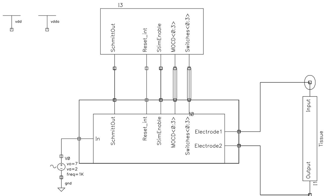
Figure 5.19: Overview of the testbench
