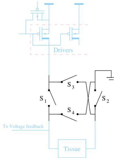
Figure 4.45: Ideal implementation of the switch array
