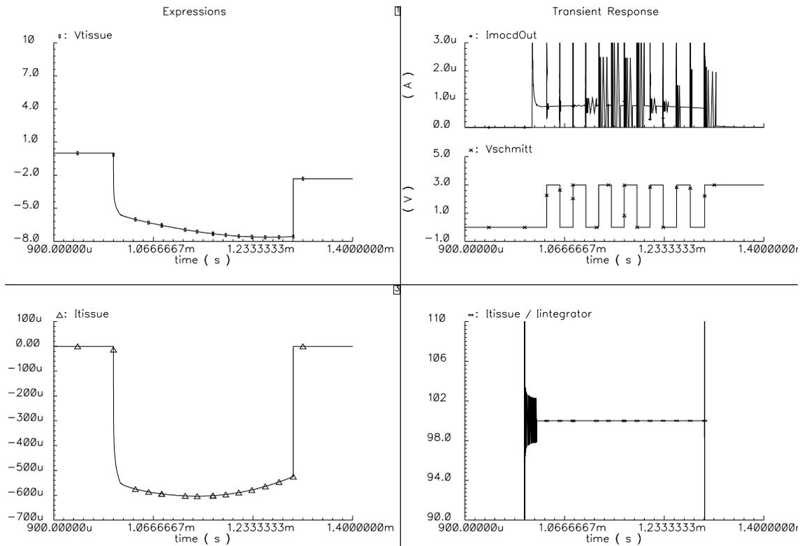
Figure 5.26: Detail of Figure 5.25 for one stimulation pulse (upper left: Tissue voltage, upper right: MOCD output current and Schmitt trigger output, lower left: Tissue current, lower right: Tissue/integrator ratio)
