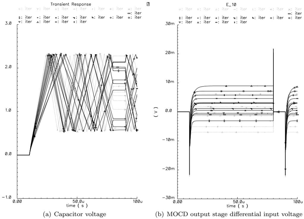
Figure 5.37: 25 run Monte Carlo mismatch simulation for the integrator
