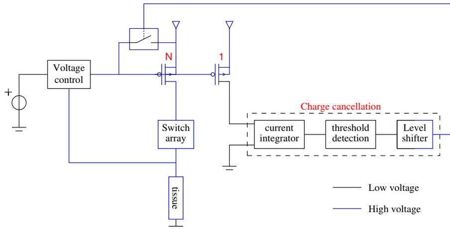
Figure 3.12: Block scheme of the output stage
