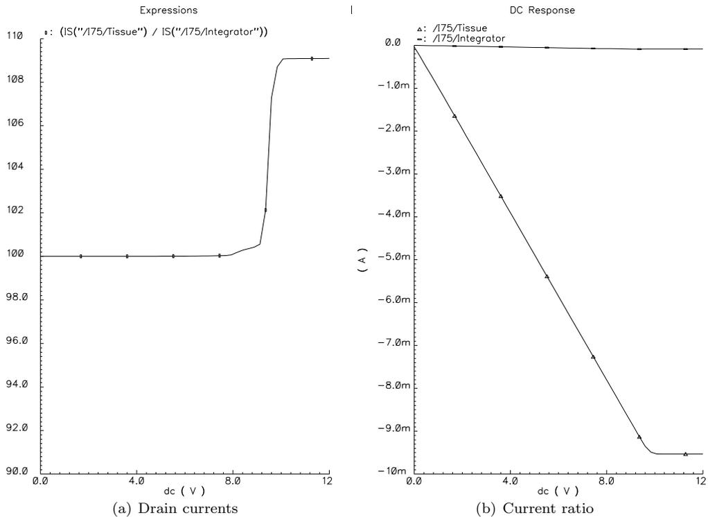
Figure 4.17: Current response using a low voltage cascode stage for CLM
