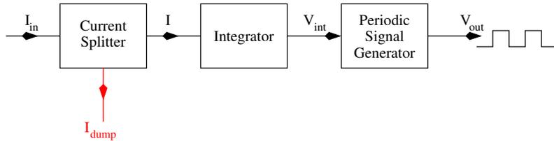
Figure 4.26: integrator system architecture
