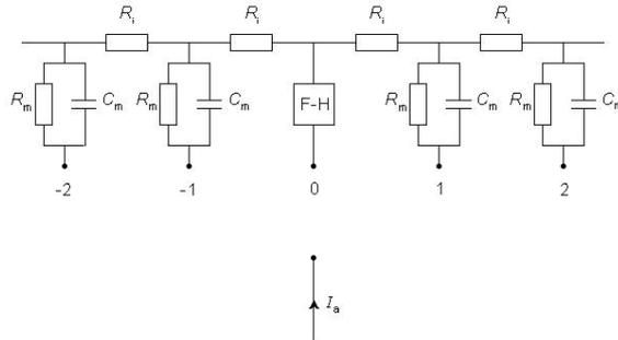
Figure 1.14: Model of the axon using the Hodgkin-Huxley equation for the central node (from [48])
