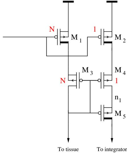
Figure 4.16: Channel Length cancellation using a low voltage cascode stage
