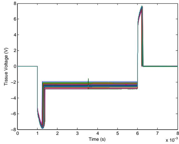
Figure 5.38: 64 run Monte Carlo simulation of the stimulator with ideal current splitter
