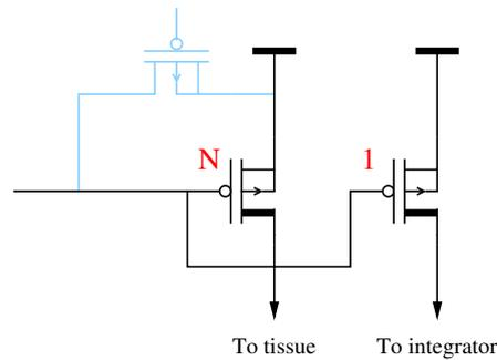
Figure 4.8: Basic design of the Driver transistors
