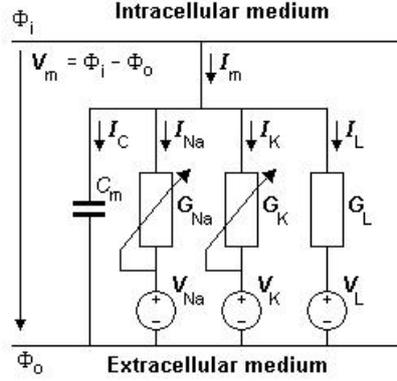
Figure 1.5: Advanced model for the membrane (from [48])
