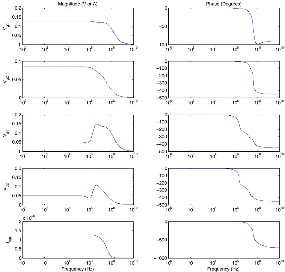
Figure 5.14: AC simulations of the MOCD output stage without stabilization network
