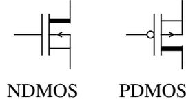
Figure 2.5: Circuit symbols for the High Voltage DMOS transistors
