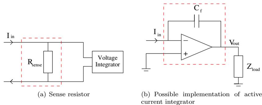
Figure 3.5: Implementation of direct current feedback systems
