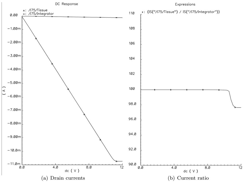
Figure 4.15: Current response using a cascode stage for CLM cancellation
