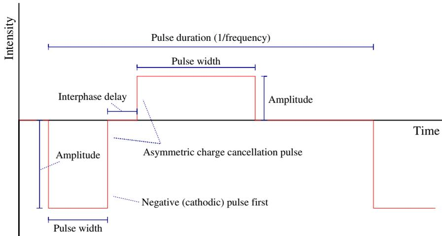
Figure 2.3: An example of a stimulation pulse with some pulse parameters denoted
