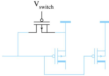
Figure 4.1: Single transistor implementation of the Stimulation enable switch
