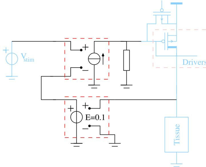
Figure 4.21: Ideal voltage feedback network
