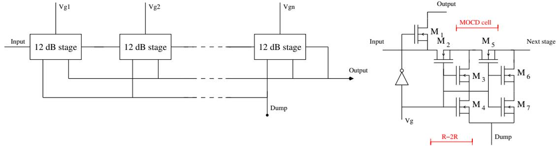
Figure 4.28: Implementation of a binary coded MOCD (block scheme left and implementation of a single block right)
