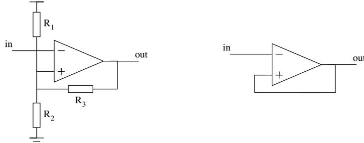
Figure 4.36: Opamp based Schmitt trigger implementation with tunable threshold voltages (left) and fixed (right)
