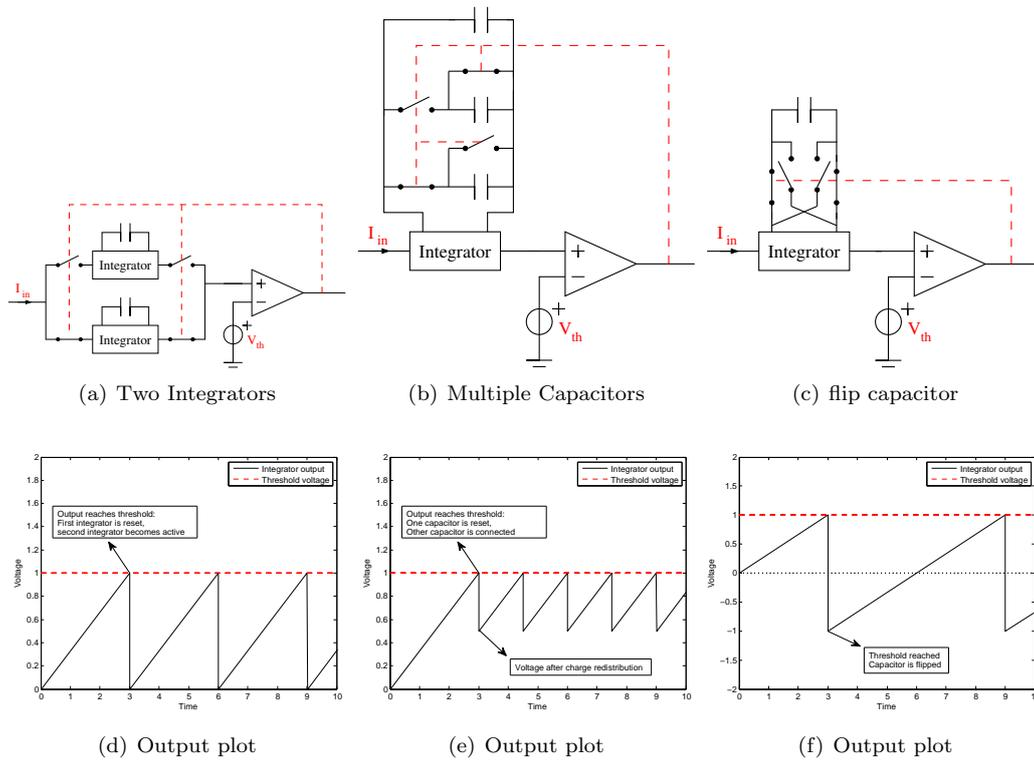
Figure 4.32: Three different integrator implementations using a single threshold level
