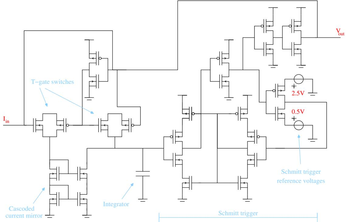
Figure 5.16: Block scheme of the integrator and comparator combination
