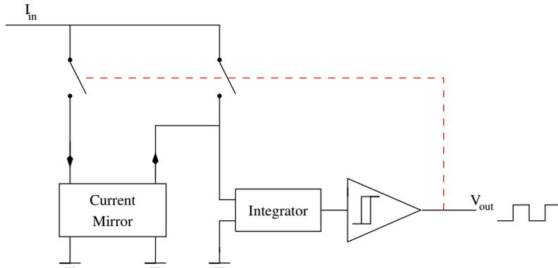
Figure 4.33: Block scheme of the integrator and comparator combination
