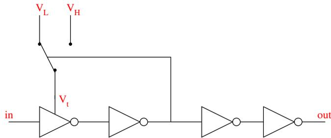
Figure 4.43: Threshold compensated inverter based Schmitt trigger
