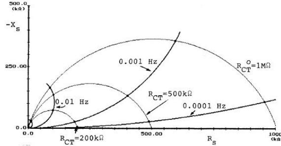
Figure 1.22: Plot of the interface impedance
