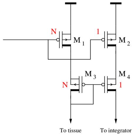
Figure 4.14: Channel Length cancellation using a cascode stage
