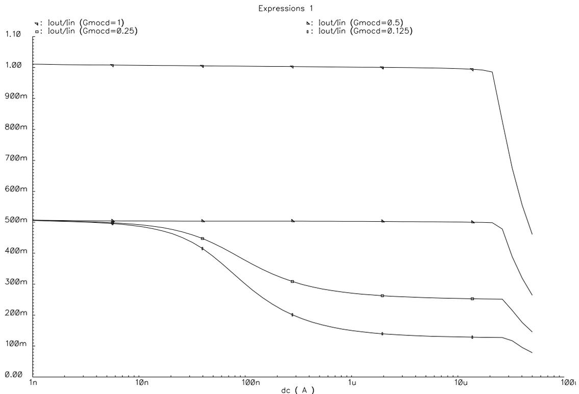
Figure 5.11: MOCD current gain using an output stage with adaptive bias
