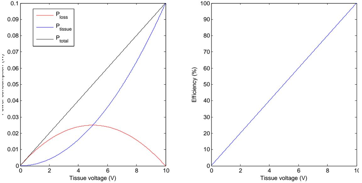
Figure 5.28: Power consumption of the tissue compared to the driver as a function of  $V_{tissue}$
