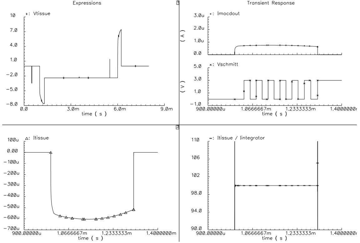
Figure 5.27: Detail of a stimulation pulse using the system with an ideal current divider (upper left: Tissue voltage, upper right: MOCOD output current and Schmitt trigger output, lower left: Tissue current, lower right: Tissue/integrator ratio)
