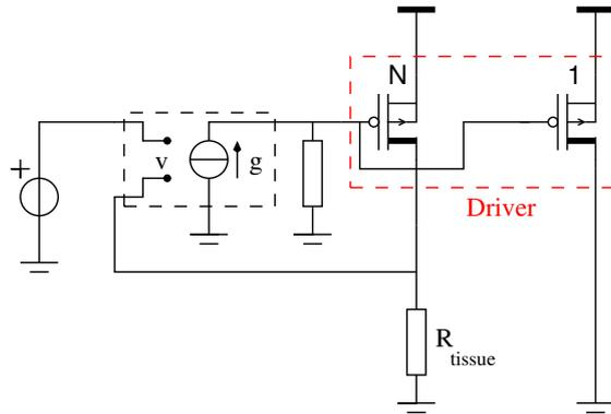
Figure 4.10: Circuit used to simulate the current ratio deviations due to Channel Length Modulation
