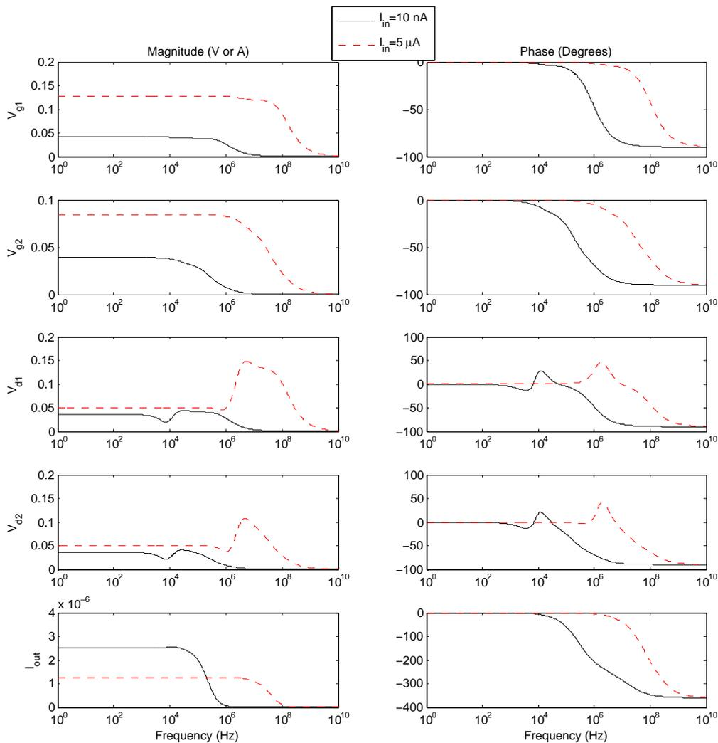
Figure 5.15: AC simulations of the MOCD output stage with two 300 fF pole splitting capacitors
