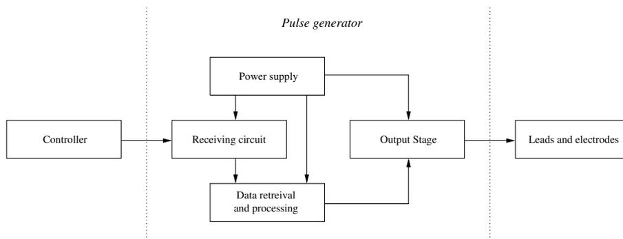
Figure 2.1: System level description of a stimulator
