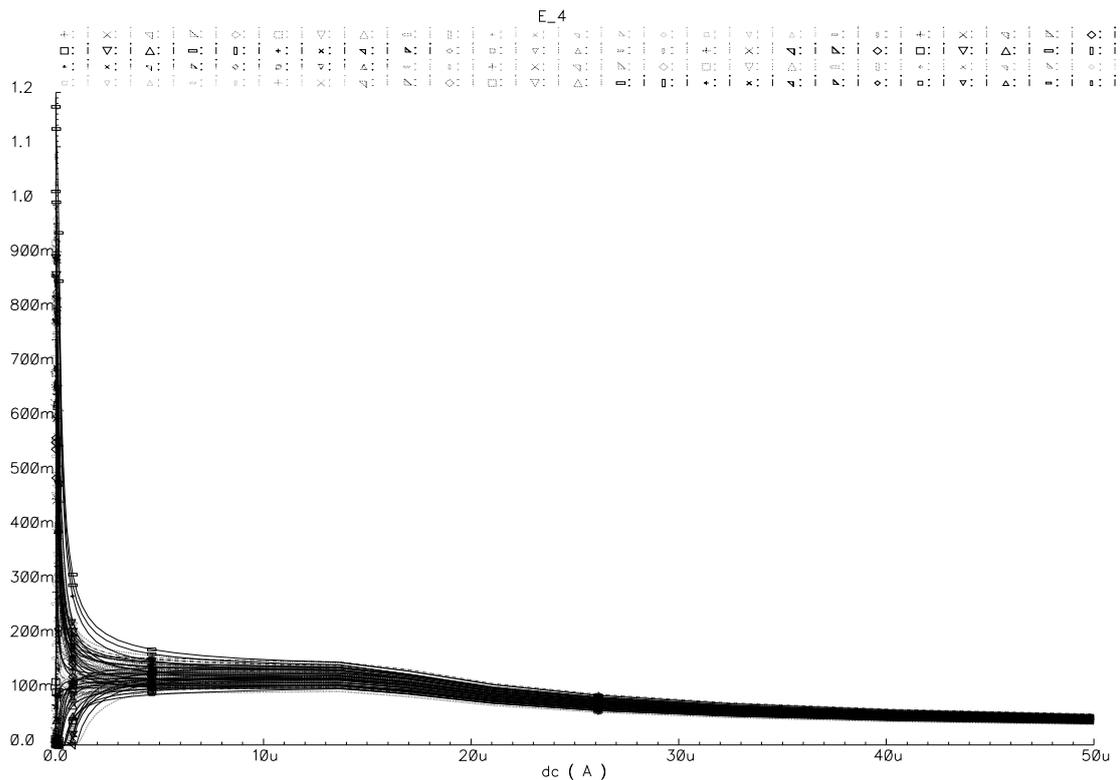
Figure 5.36: 100 run Monte Carlo mismatch simulation for the MOCD current gain
