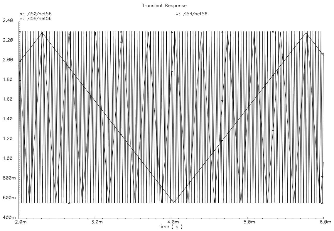
Figure 5.17: Voltage over the capacitor in the integrator for different input currents
