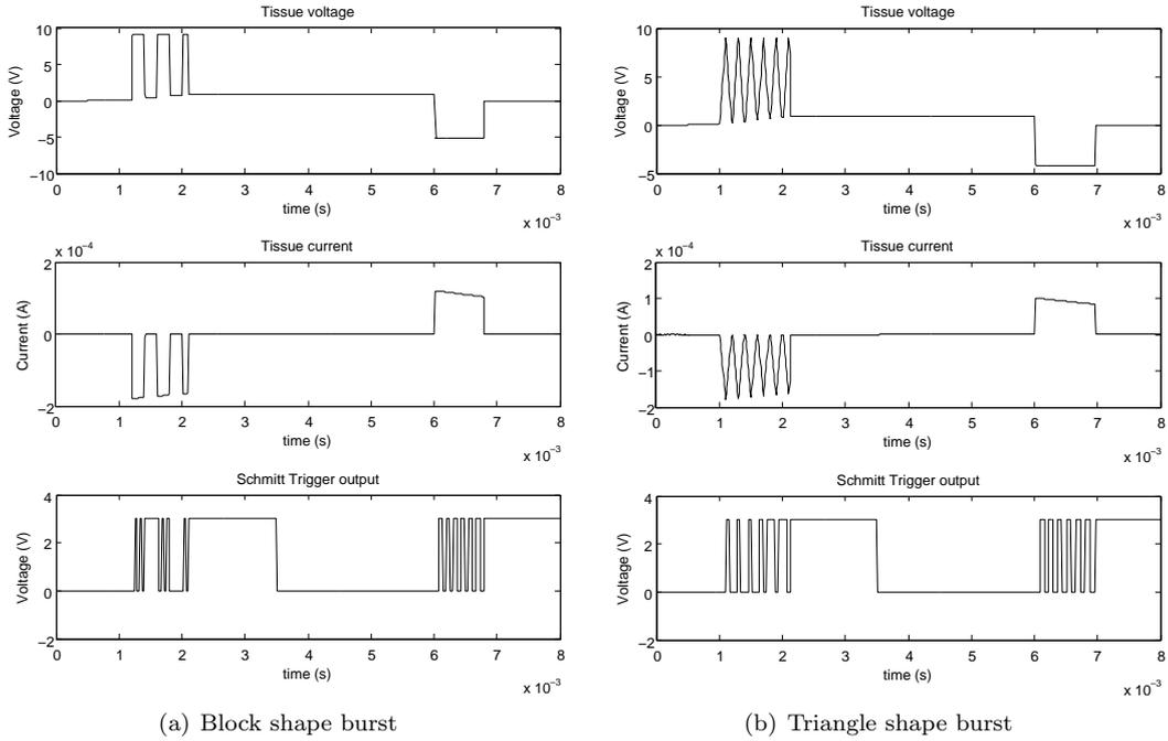
Figure 5.31: System response for a burst (left) and triangular (right) stimulation
