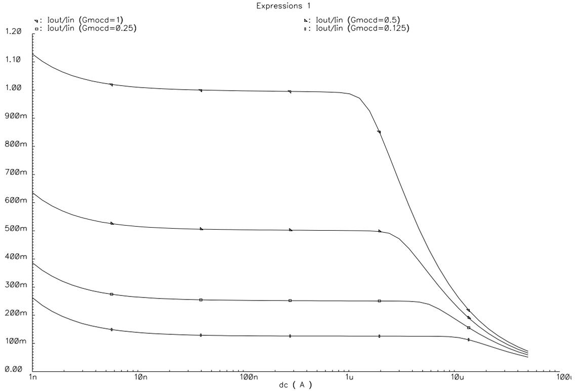
Figure 5.9: MOCD current gain using a buffered output stage with fixed bias (10 nA)
