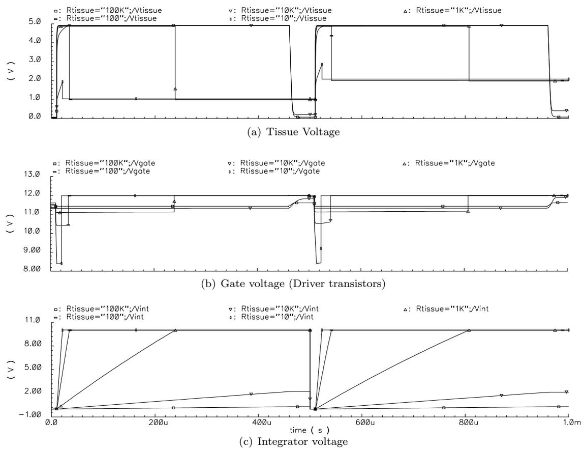
Figure 5.5: Transient simulations for varying tissue resistance
