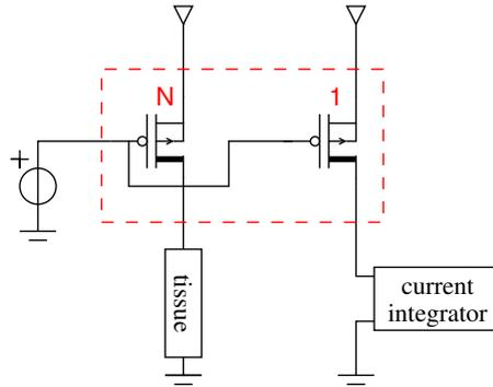
Figure 3.9: Using a current mirror to generate the copy of the current
