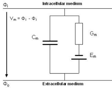
Figure 1.4: Basic electrical model for the cell membrane (from [48])
