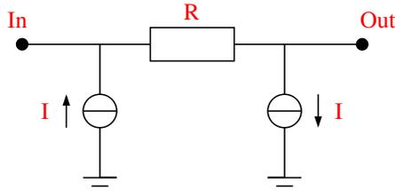
Figure 4.3: Implementation of the level shifter using a resistor and two current sources
