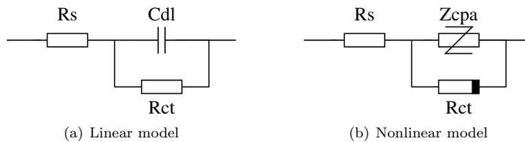
Figure 3.17: Two commonly used interface models (copied from chapter 1.4)
