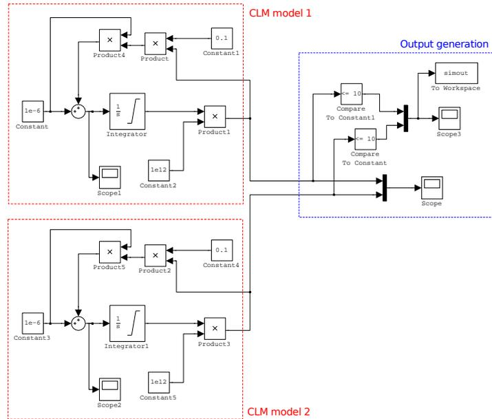
Figure 4.34: Simulink block scheme to compare the effect of channel length modulation for two inputs
