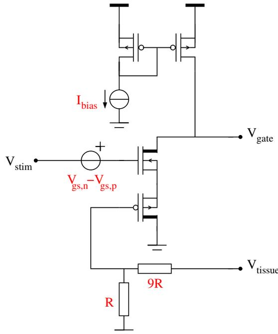
Figure 4.25: Design of the voltage feedback network
