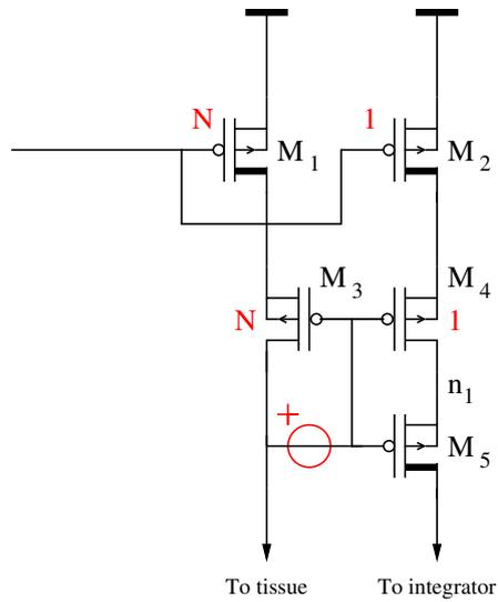
Figure 4.18: Increasing the Tissue voltage swing by boosting the voltage
