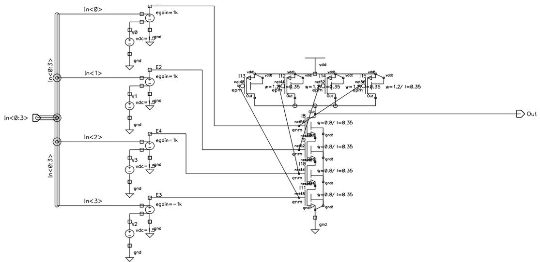
Figure 5.23: Implementation of the charge threshold block in the testbench
