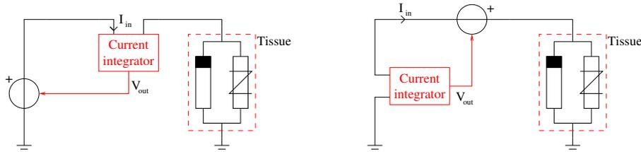
Figure 3.4: Two alternatives for a stimulator with direct current feedback
