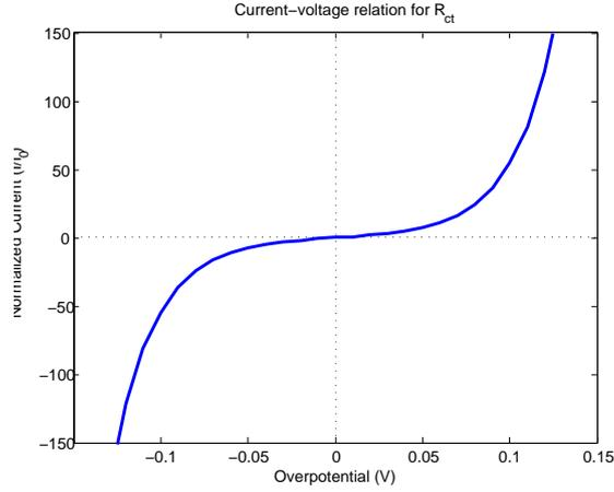
Figure 1.21: Current-voltage relation for the nonlinear charge transfer resistance
