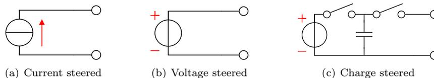
Figure 3.1: Three fundamental output stage types
