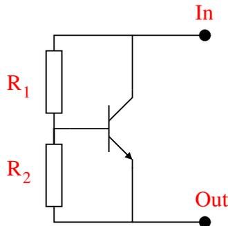
Figure 4.4: Implementation of the level shifter using a  $V_{be}$  multiplier
