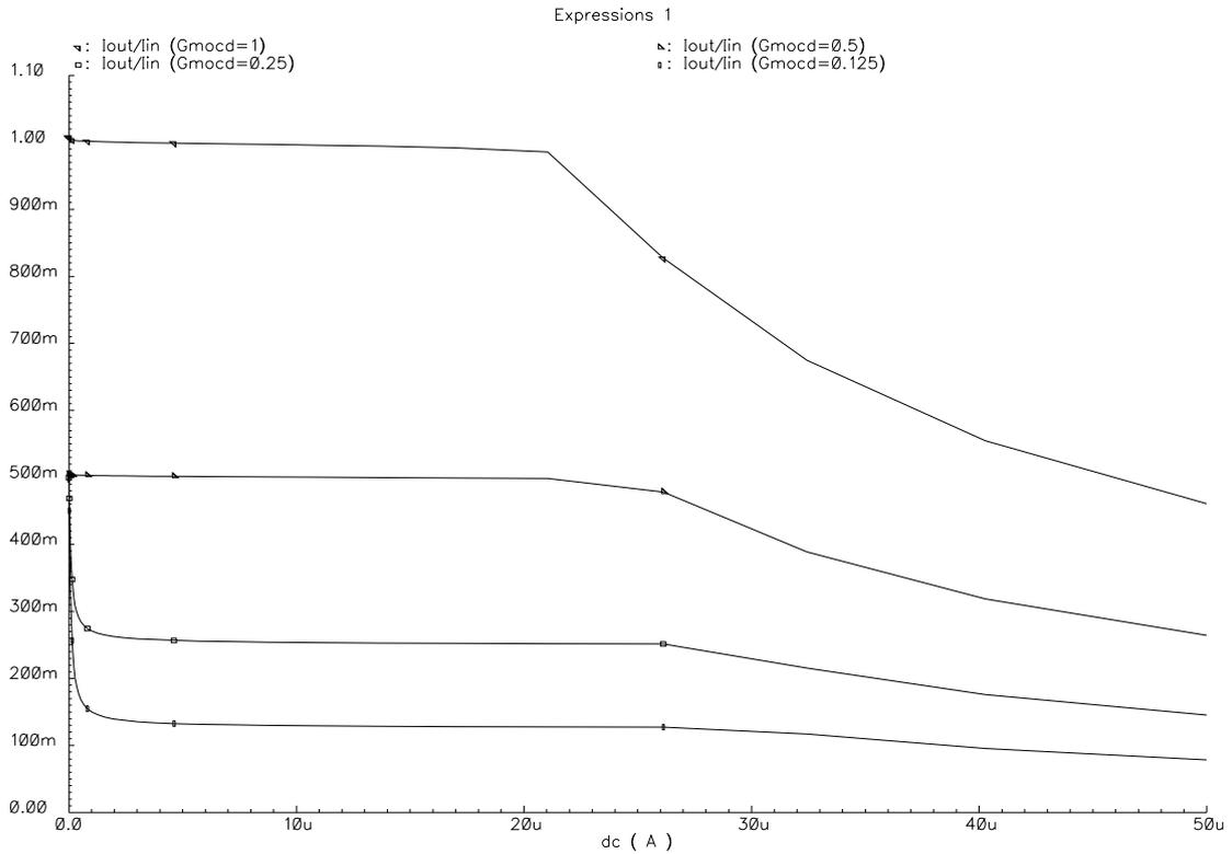
Figure 5.13: MOCD current gain using an output stage with adaptive bias (linear scales)
