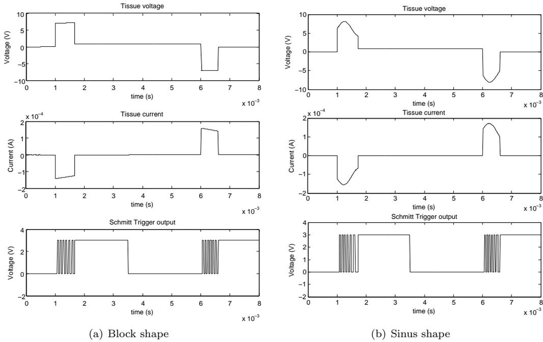
Figure 5.30: System response for a block (left) and shifted sinusoid (right) shaped stimulation
