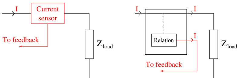
Figure 3.3: Principle of direct (left) and indirect (right) current feedback networks
