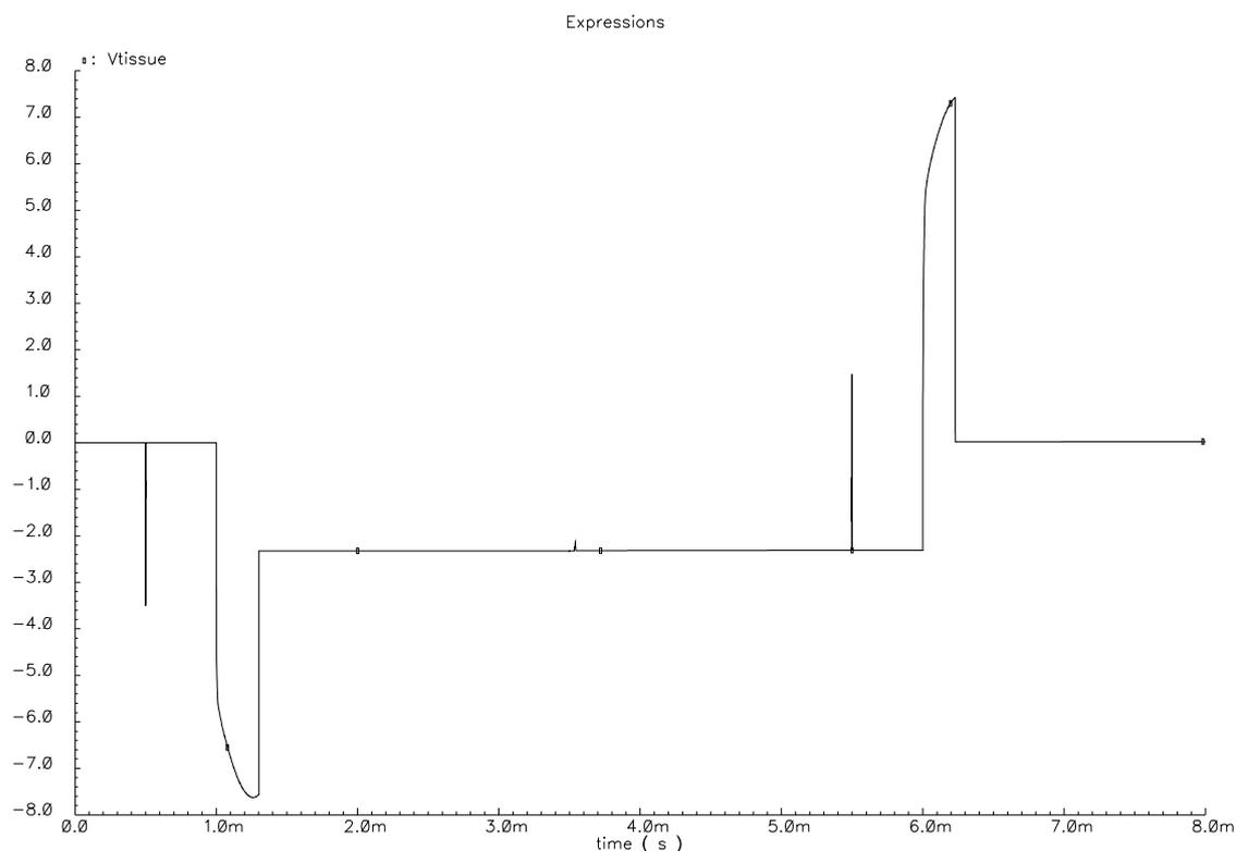
Figure 5.25: Tissue voltage during a complete stimulation cycle
