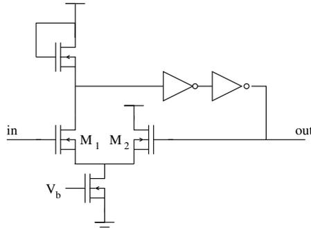
Figure 4.39: Possible implementation of the Schmitt trigger [63]
