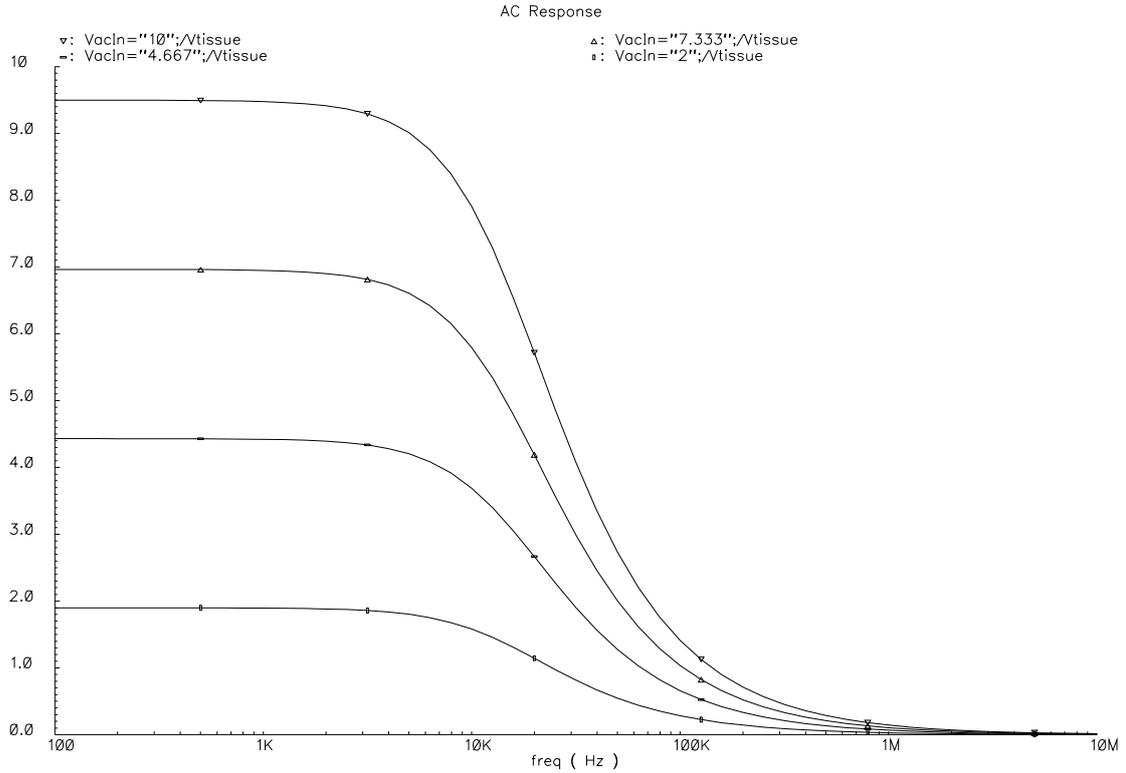
Figure 5.7: AC simulations of the tissue voltage for various input voltages
