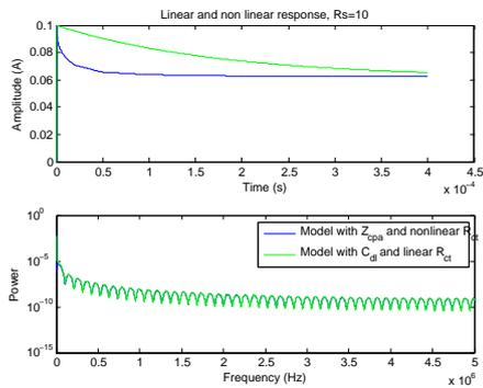
(c)  $\beta = 0.75$ ,  $R_s = 10 \Omega$ ,  $K = 22 \text{ k}\Omega \text{ s}^\beta$
