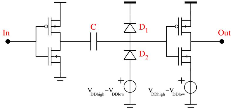
Figure 4.5: Implementation of the level shifter using a capacitor
