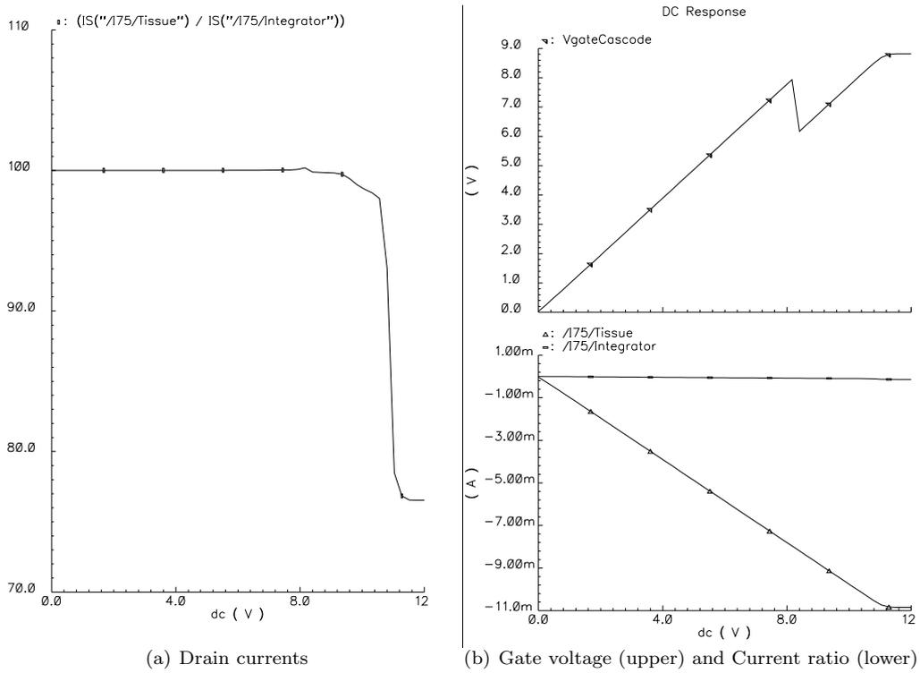
Figure 4.19: Current response using using a low voltage cascode stage with a boosted tissue voltage
