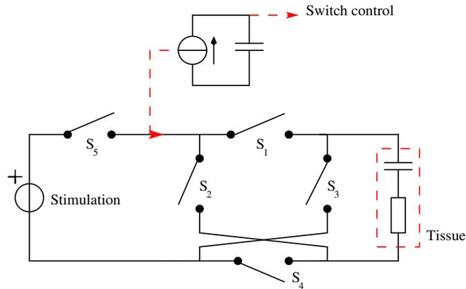
Figure 3.13: Simplified ideal circuit representing voltage based stimulation with charge cancellation
