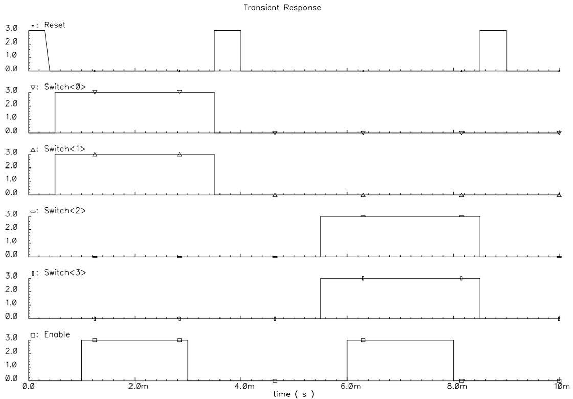
Figure 5.24: Control signals used for a simulation cycle
