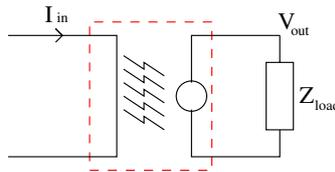
Figure 3.6: Passive indirect feedback: current clamp
