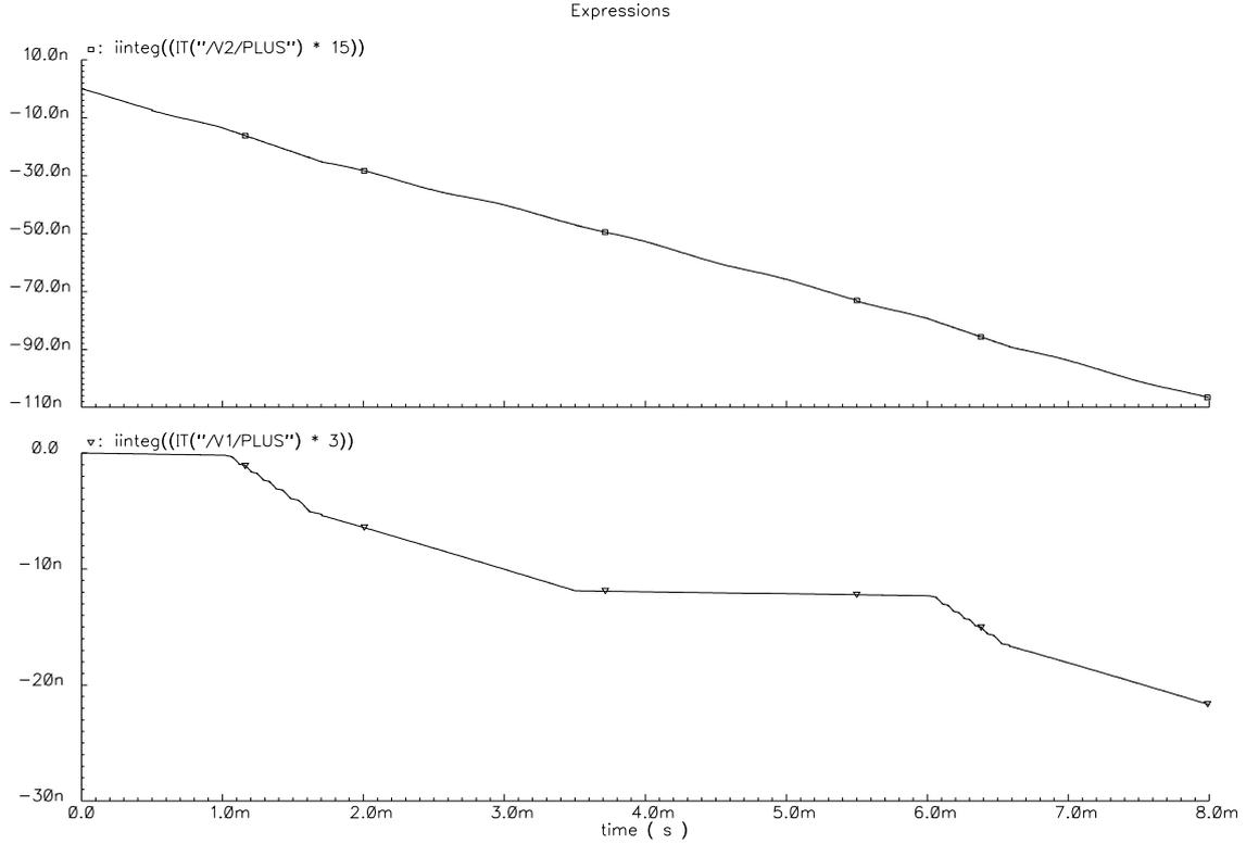
Figure 5.29: Power consumption of  $V_{DDhigh}$  (upper plot, excluding driver and enable switch) and  $V_{DDlow}$  (lower)
