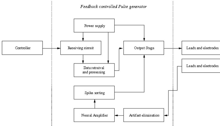
Figure 2.2: System level description of a stimulator with feedback
