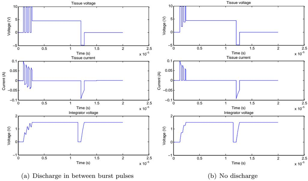
Figure 3.16: Pulsetrain waveform stimulation
