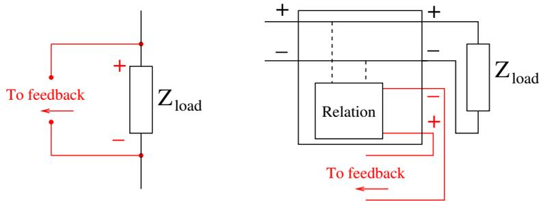
Figure 3.2: Principle of direct (left) and indirect (right) voltage feedback networks
