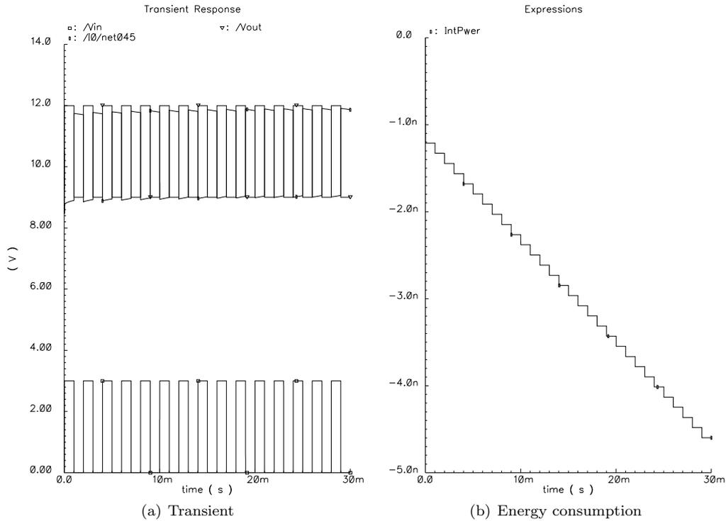
Figure 5.1: Simulation results of the capacitor based level shifter
