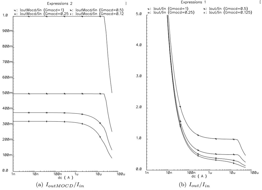
Figure 5.12: MOCD current gain using an output stage with a fixed bias ( $10 \mu\text{A}$ )
