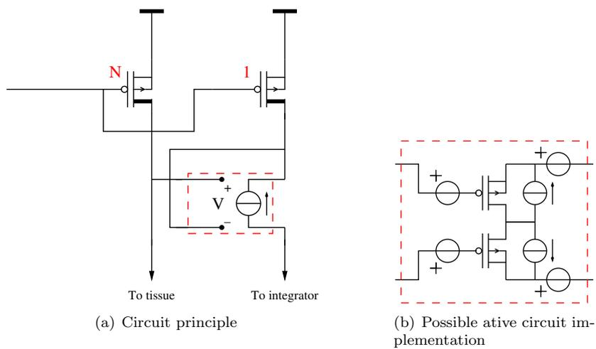
Figure 4.12: Channel Length cancellation using an ideal active circuit
