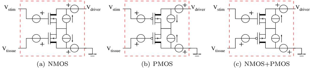
Figure 4.22: Three different biasing schemes for the differential CS stage
