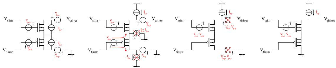
Figure 4.23: Biasing of the CS stage
