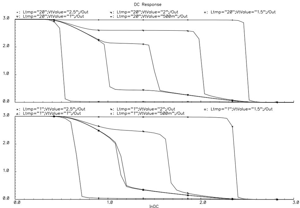
Figure 4.44: DC response of a symmetric (upper plot) and asymmetric (lower plot) threshold compensated inverter
