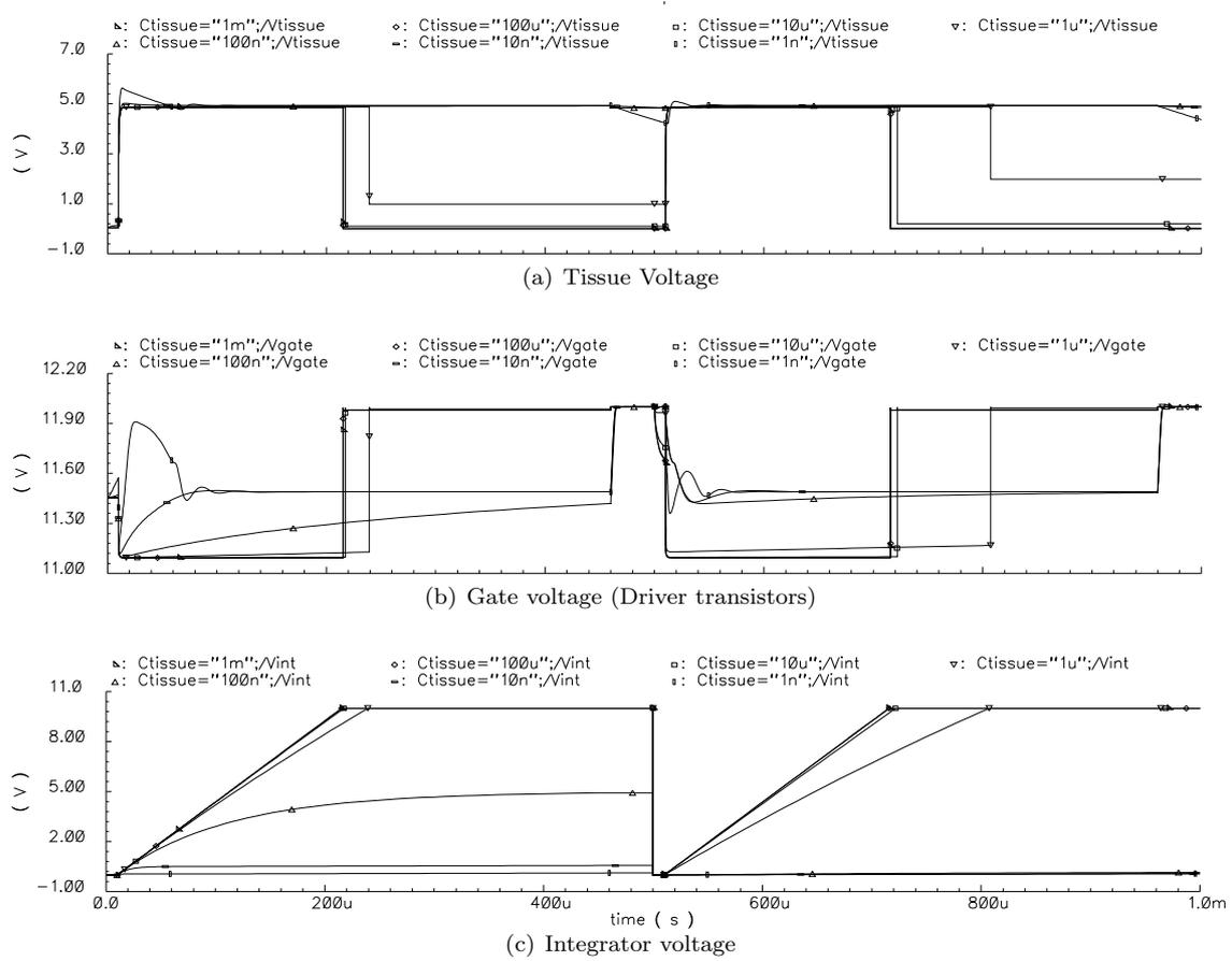
Figure 5.6: Transient simulations for varying tissue capacitance
