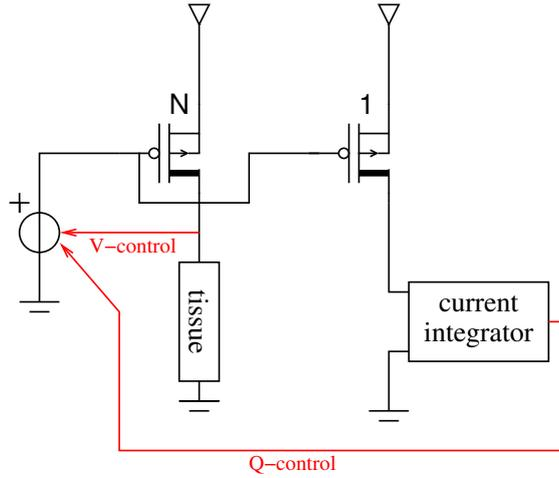
Figure 3.10: High level design of the output stage
