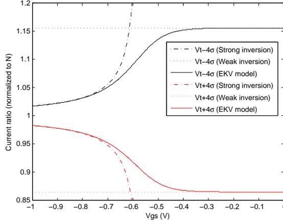
Figure 4.9: Normalized current ratio due to intra die  $V_t$  mismatches
