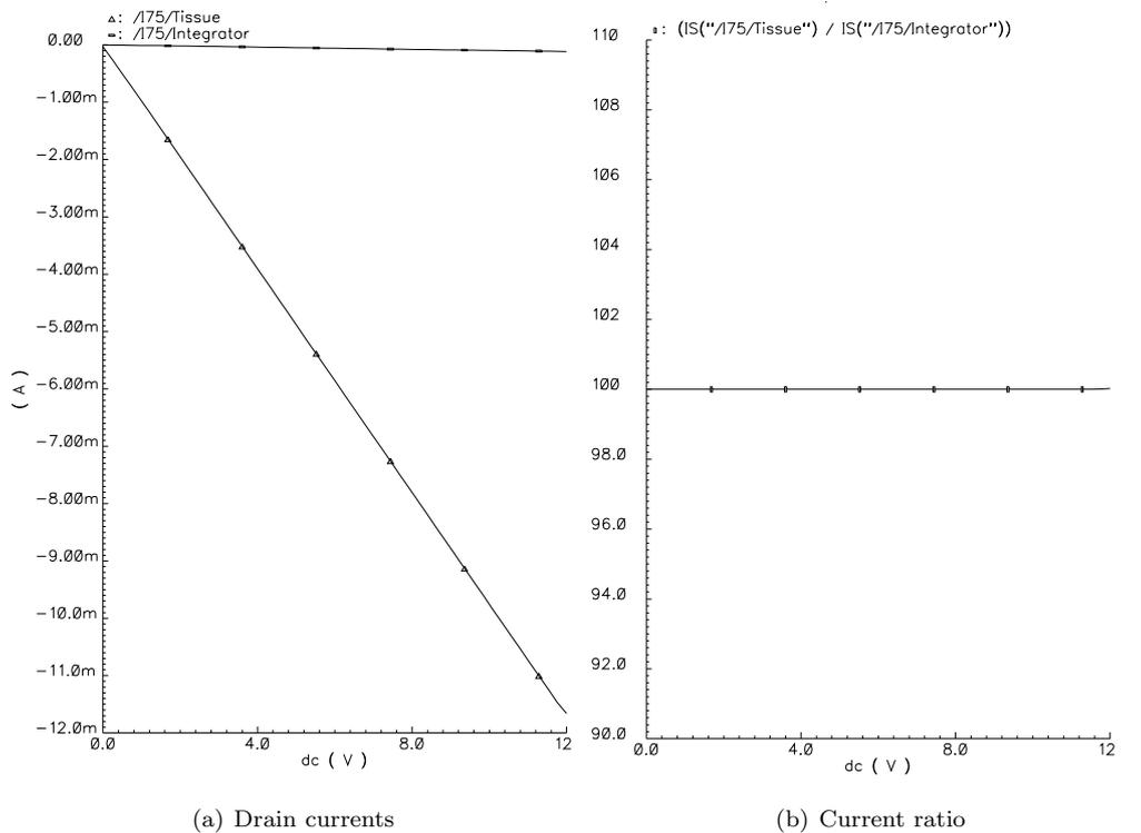
Figure 4.13: Current response using the active circuit for CLM cancellation
