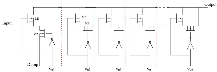
Figure 4.29: Implementation of a thermometer coded MOCD
