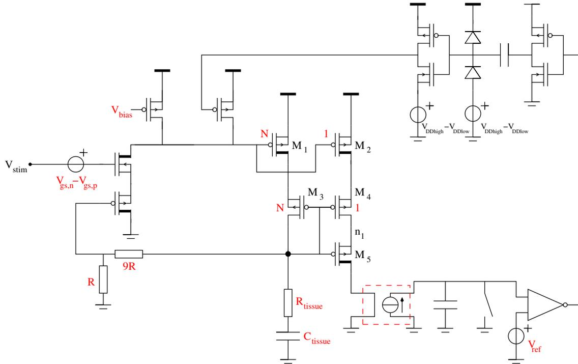
Figure 5.3: Circuit used to simulate the working principle of the stimulation circuit
