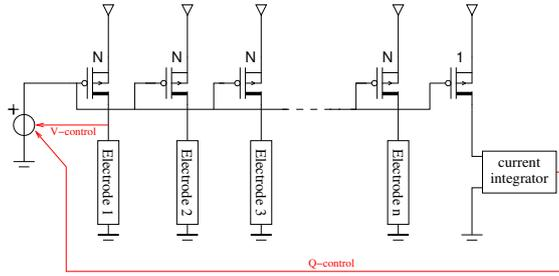
Figure 3.11: System configuration with multiple electrodes
