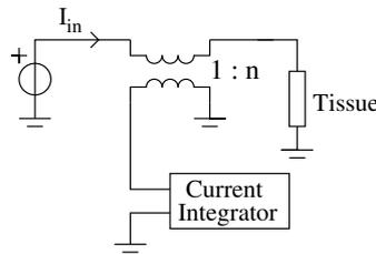
Figure 3.7: Using a transformer to generate the copy of the current
