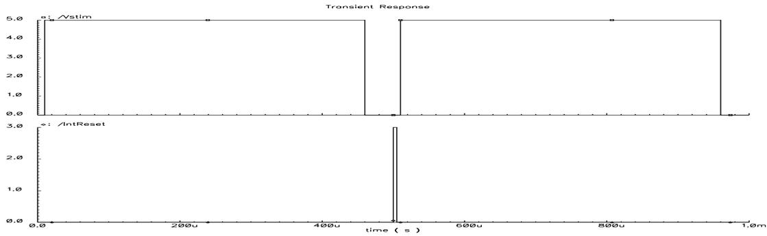
Figure 5.4: Input waveforms used for transient simulations
