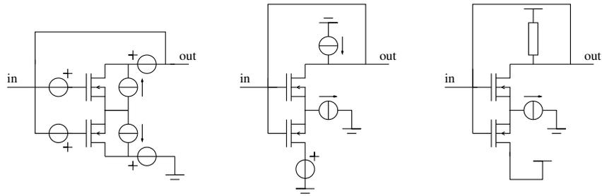
Figure 4.37: 'Biasing' of the differential pair to implement the Schmitt trigger
