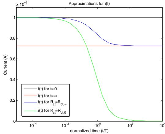
Figure 3.19: Plots of approximations  $i(t)$  for several values of  $R_{ct}$
