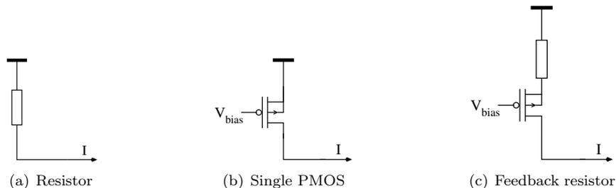
Figure 4.24: Three alternative current source implementations
