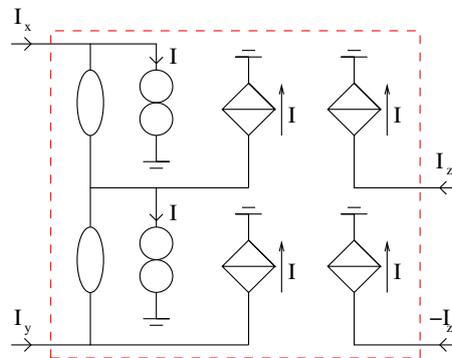
Figure 3.8: The principle of the third generation current conveyors
