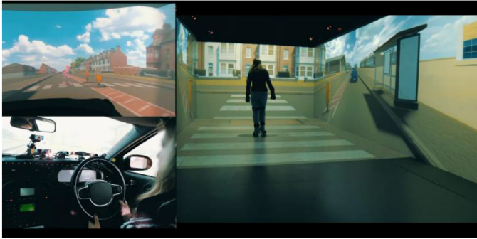
Fig. 1. Experimental scene in the DSS. Top left shows the driver's view of the pedestrian, with the pedestrian represented by pink spheres to the driver. Bottom left displays the driver behind the wheel of the UOLDS. On the right, the pedestrian is seen crossing the zebra in the CAVE-based pedestrian lab [14].
