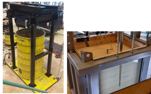
Figure 2: The Deltares calibration chamber (CC) test devices: (left) cylindrical CC and (right) half-CC with glass.
