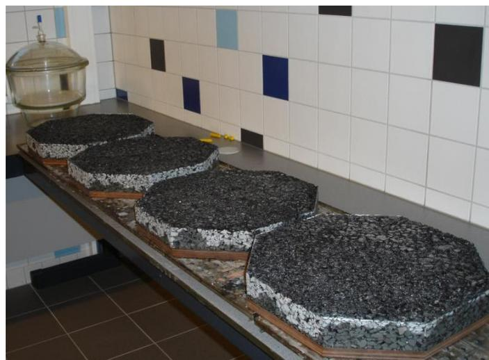
**Figure 7.4:** RSAT slabs with 4% steel wool 00 prepared by Breijn-Heijmans
