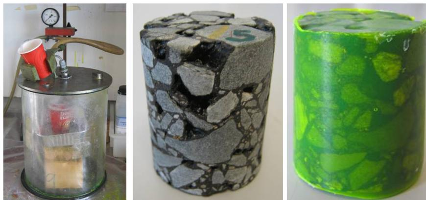
**Figure 5.21:** The set-up of impregnation and the sample before and after impregnation
