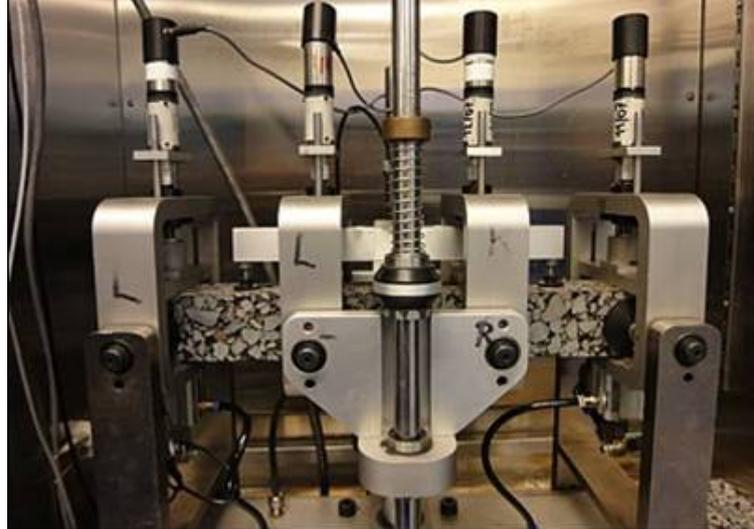
**Figure 6.20:** The set-up of four point bending fatigue test
