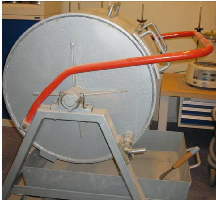
**Figure 5.1:** Los Angeles abrasion machine used in this research
