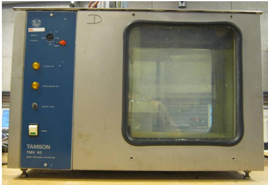
**Figure 5.12:** The water bath used in this research
