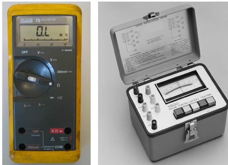
**Figure 4.3:** Fluke digital multimeter (left) and gage installation tester (right)
