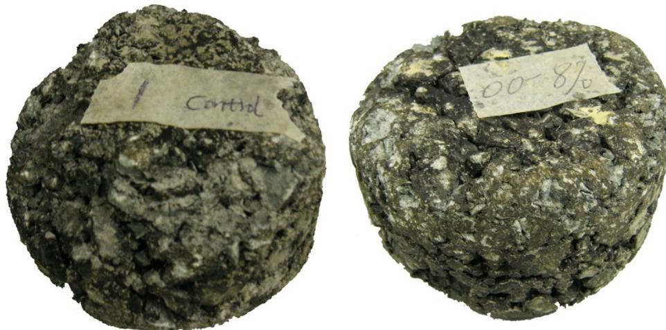
**Figure 5.2:** Porous asphalt concrete samples after particle loss testing
