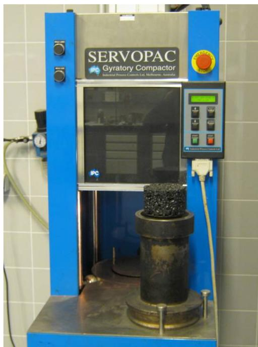
**Figure 3.9** Servopac Gyrotory Compactor used in this research and the sample compacted
