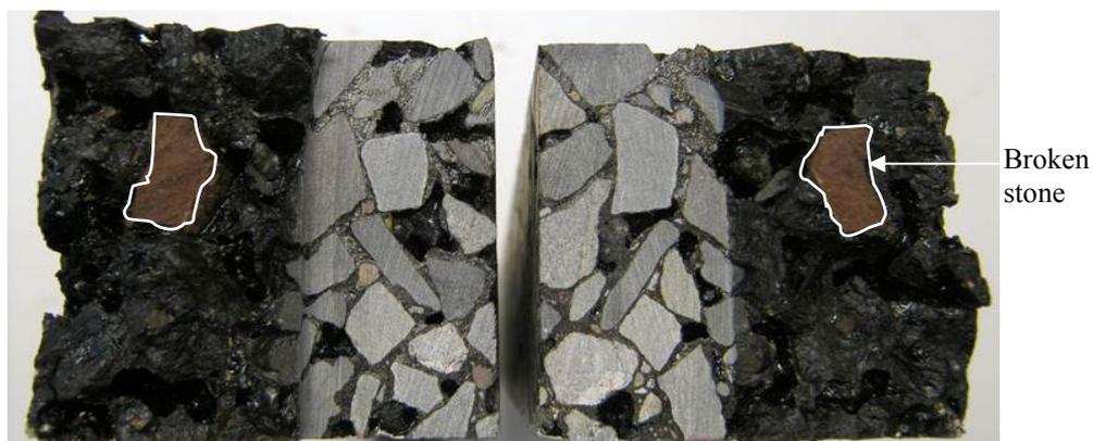
**Figure 6.11:** Fractured beam (with broken stone)
