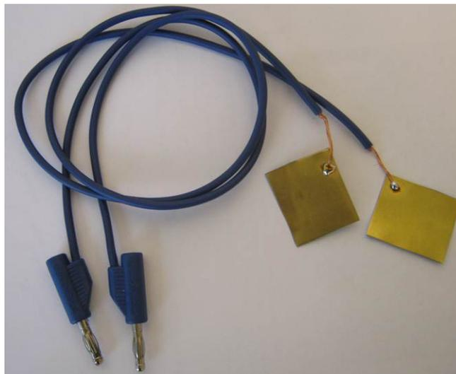
**Figure 4.4:** Self-made electrodes used in measuring the resistance of asphalt mastic beams
