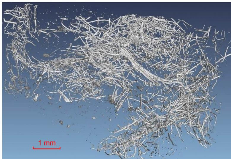
**Figure 7.24:** Steel wool distributions in the sample
