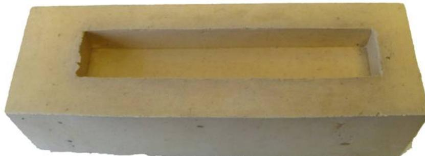
**Figure 3.6** Mould used for preparing mastic beam samples for electrical resistance and heating tests
