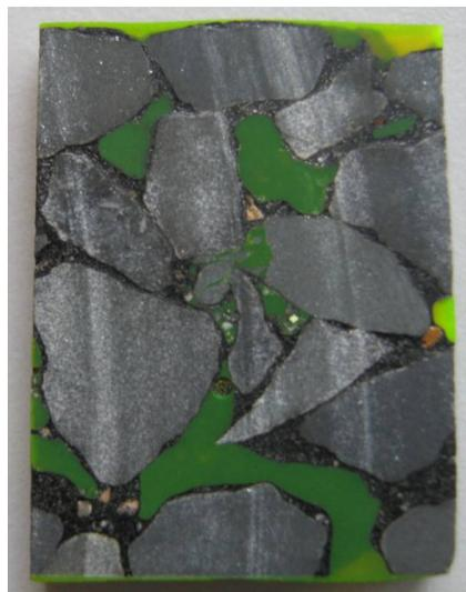
**Figure 5.24:** Sample ready for nano-indentation testing
