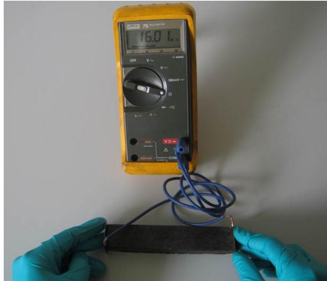
**Figure 4.5:** The testing method of resistance measurement on a asphalt mastic beam
