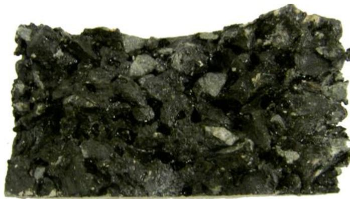
**Figure 5.9:** Appearance of the fracture surface of the sample after ITS test
