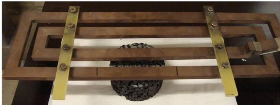
**Figure 4.18:** Induction heating setup
