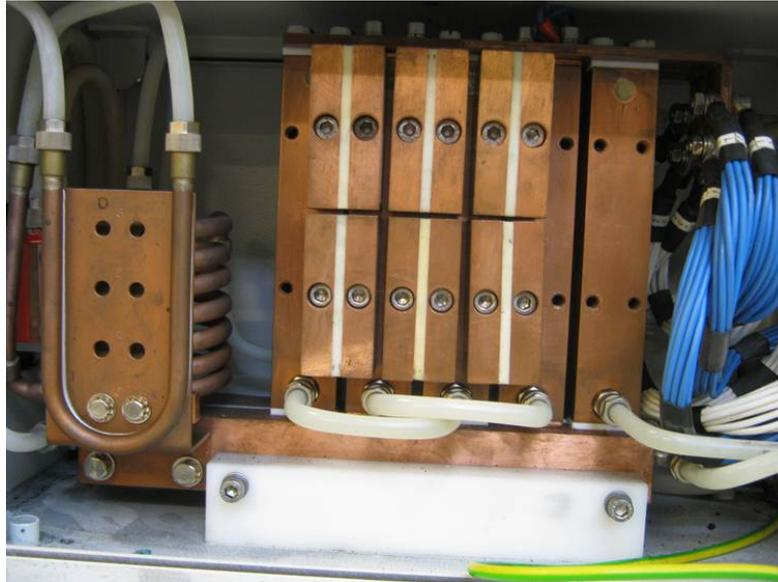
**Figure 4.17:** Configuration of the induction heating generator with 6 capacitors: the number of the capacitors can be varied to change the frequency of the magnetic field
