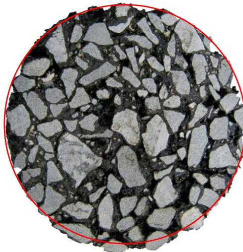
**Figure 4.28:** Swelling appearance of the over-heated sample
