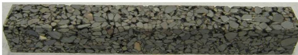
**Figure 3.14** Porous asphalt concrete beam used in this research
