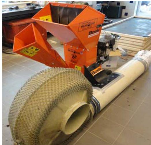
**Figure 7.9:** Wood chipper used to disperse steel wool
