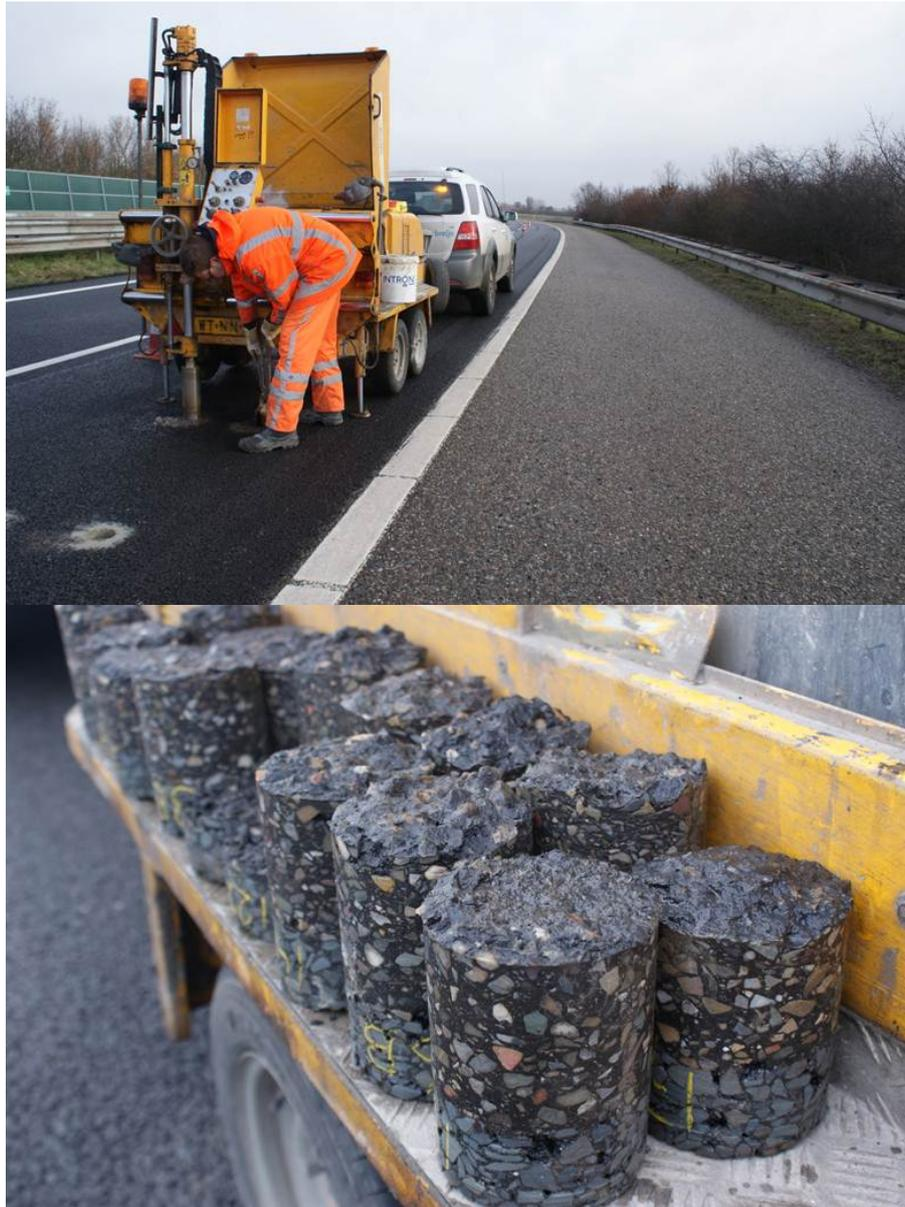
**Figure 7.12:** Drilling cores from the induction heating trial section
