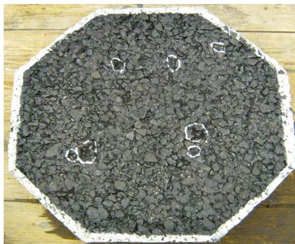
**Figure 7.6:** Sample with stone loss after rotating surface abrasion test
