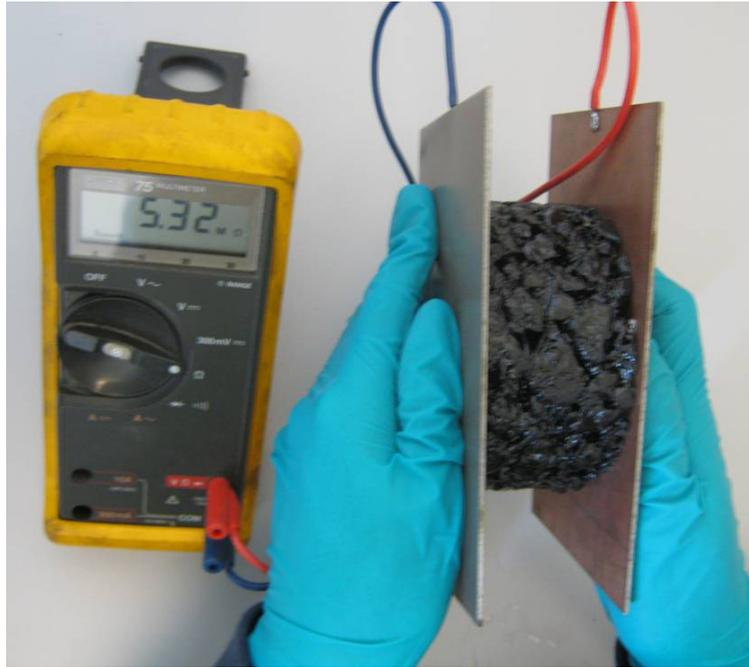
**Figure 4.7:** The testing method of resistance measurement on a porous asphalt concrete cylinder
