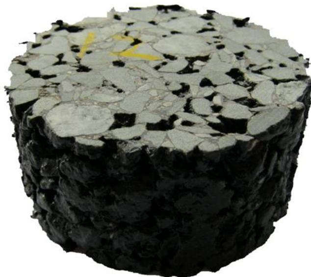
**Figure 4.2:** Porous asphalt concrete cylinder used in resistance testing
