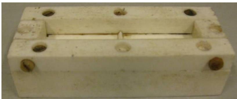
**Figure 3.7** Mould used for preparing notched mastic beam samples for healing test
