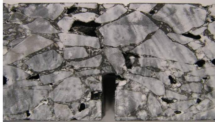
**Figure 6.15:** Fractured beam immediately after induction heating
