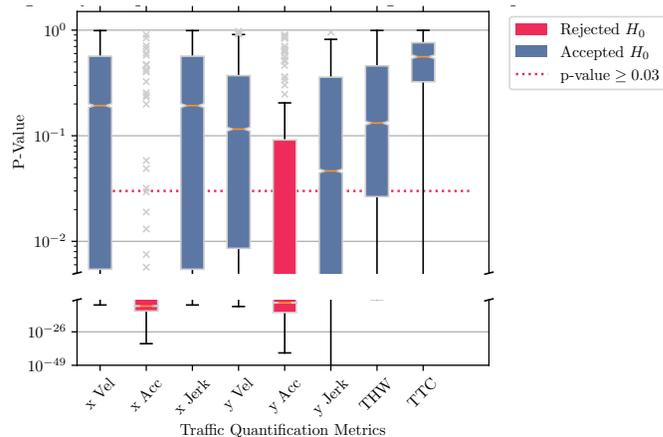
Fig. 4: Homogeneity between  $C_{1,HighD}$  and  $C_{1,openPASS}$ , expressing the quality of the simulation’s recreation of a real-world traffic observation.
