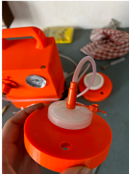
Figure 7.1: Placement of bacterial filter and desired tube to motor
