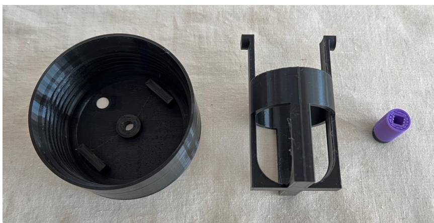
Figure 20: 3D printed parts of the WOCA Canister.
