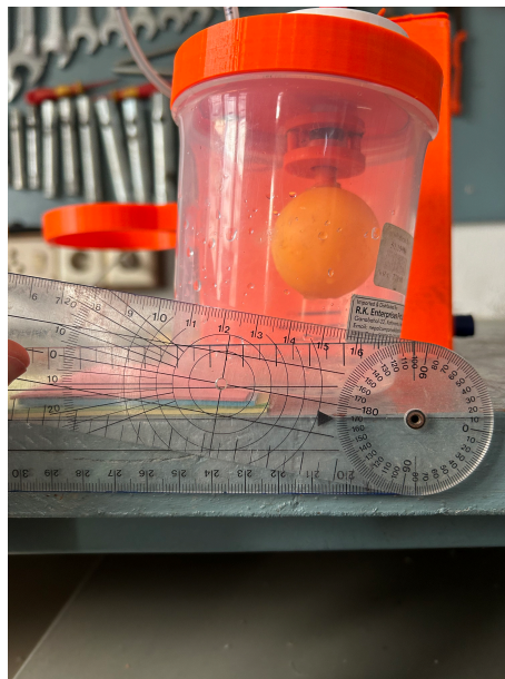
Figure 5.2: Overflowprotection test for ISO-norm criteria 7.1.
