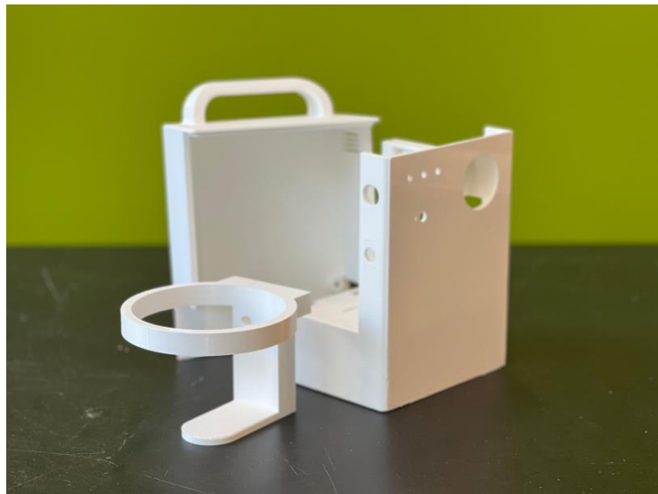
Figure 5: 3D printed parts of the WOCA Vacuum Pump.
