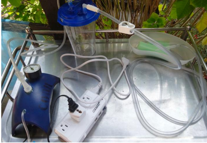
Figure 1: Setup of the converted aquarium pump (AquaVAC) used in Green Pastures Hospital.
