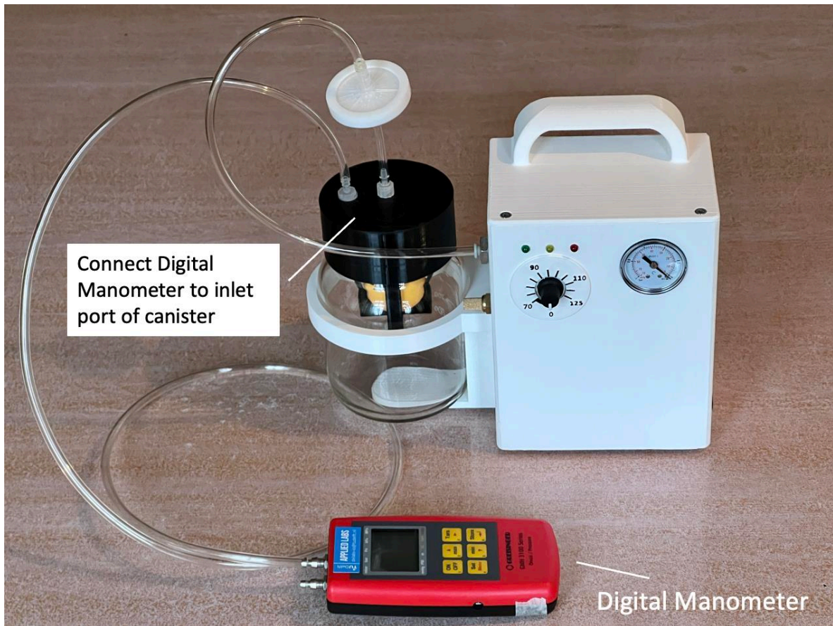
Figure 26: Setup for leakage test of the WOCA Pump
