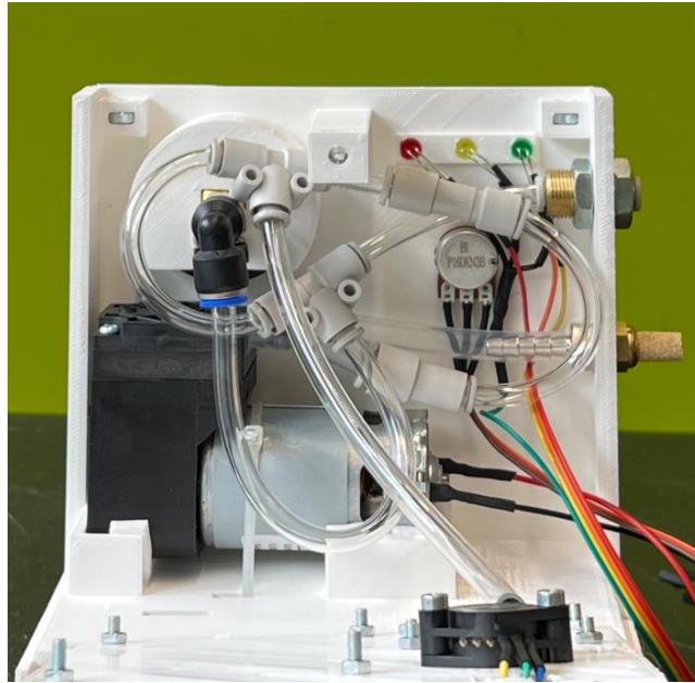
Figure 14: Components in the WOCA vacuum pump with all the tubing connected.
