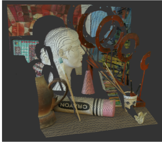
Figure 2.7: Pointcloud resulting from stereo matching of Middlebury dataset example stereo pair and disparity map
