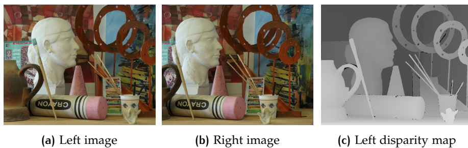
Figure 2.5: Rectified stereo pair and disparity from Middlebury dataset [Scharstein and Pal, 2007]
