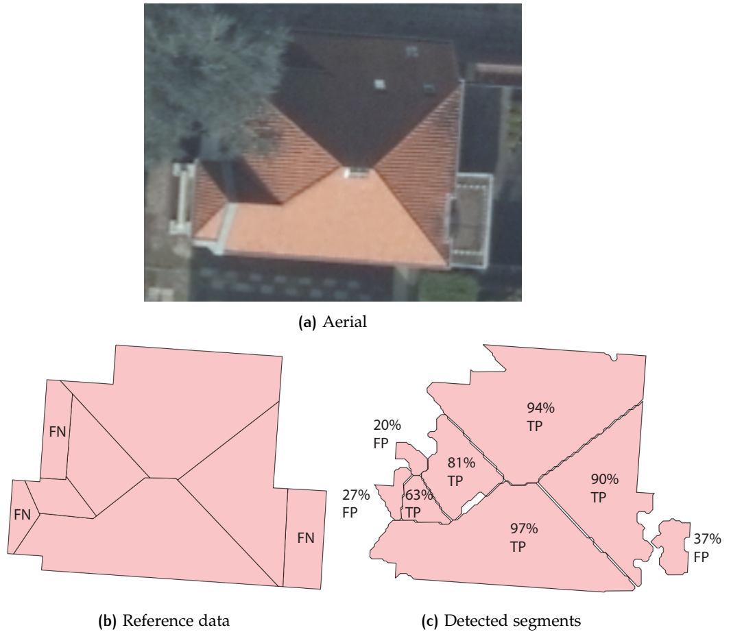
Figure 5.3: Example of how percentage of overlap determines whether a segment is a TP or FP , and segments that are not detected ( FN )
