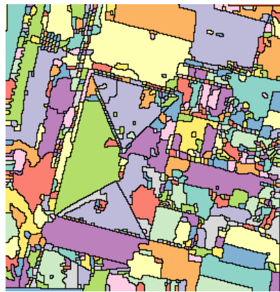
Figure 4.7: Similar color segments retrieved with watershed segmentation of the gradient magnitude
