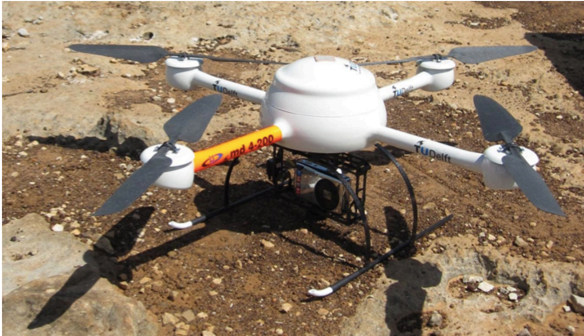
Figure 2.1: A UAV with its movable digital camera underneath. The UAV has a diameter of 540 mm and a height of 230 mm. This drone has been used in outcrops images acquisition for most of the outcrops images used in this thesis. Source: van Eijk (2014)
