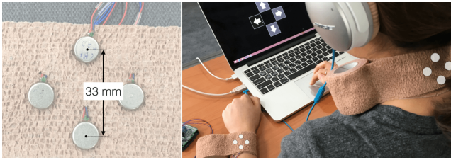
Fig. 13: Airflow-based indentation tactile interface by Lee and Lee [55]. On the left is a closer look at the prototype's 4 air pumps, on the right is the device strapped around the back of the neck and wrist.
