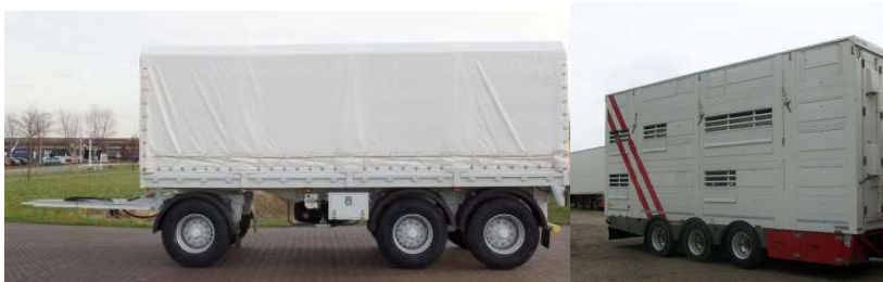
Figure 12 - Pictures of different trailer types which can be carried by full trucks. Left: ADFT. Right: CCT. 11
