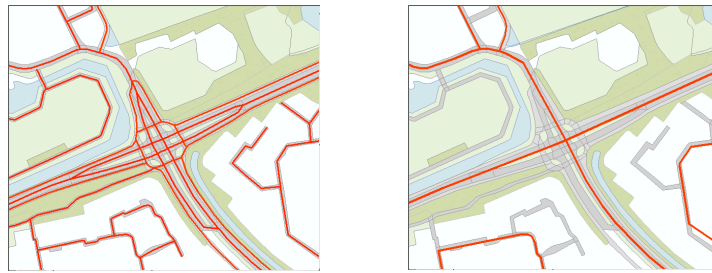
Figure 1 Centrelines in TOP10NL (left) and TOP50 (right), both projected on TOP10NL polygons
