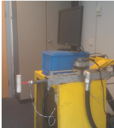
FIGURE A-1: THE PROPRIO MANIPULATOR ON WHERE THE EXPERIMENTS ARE EXECUTED. SUBJECTS USED THE WHITE HANDLE TO CONTROL THE SLOW DYNAMIC SYSTEM WHICH IS VISUALIZED ON THE SCREEN.
