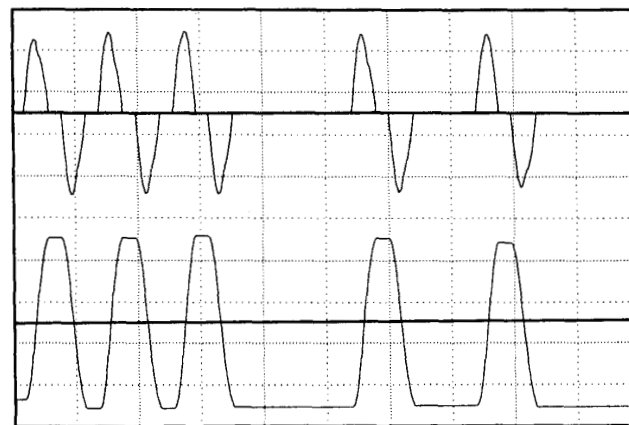
Fig. 9. Results of computer simulation [time 1 ms]: Upper trace: resonant current i , [50 A/div]. Lower trace: resonant capacitor voltage u_{Cr} , [150 V/div].
