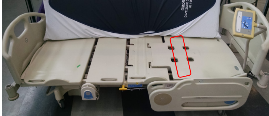
Figure 3.2: Standardized hospital bed produced by Hill-Rom which is used in the experiments, with the sensor system location indicated by the red rectangle.
