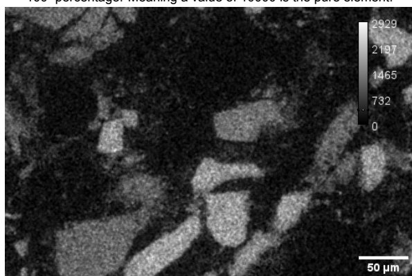
(e) Magnesium content in the M1 structure in sample 13. The colour scale indicates the elemental percentage of Mg atoms. The value is given as 100×percentage. Meaning a value of 10000 is the pure element.
