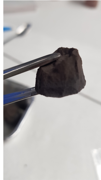
(b) An example of an hourglass failure shape after compressive testing. This is the bottom part.
