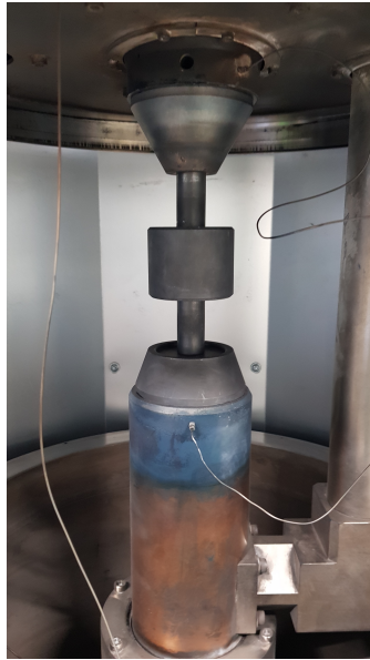
(a) The punch and die assembly within the opened SPS chamber. The material residues within.
