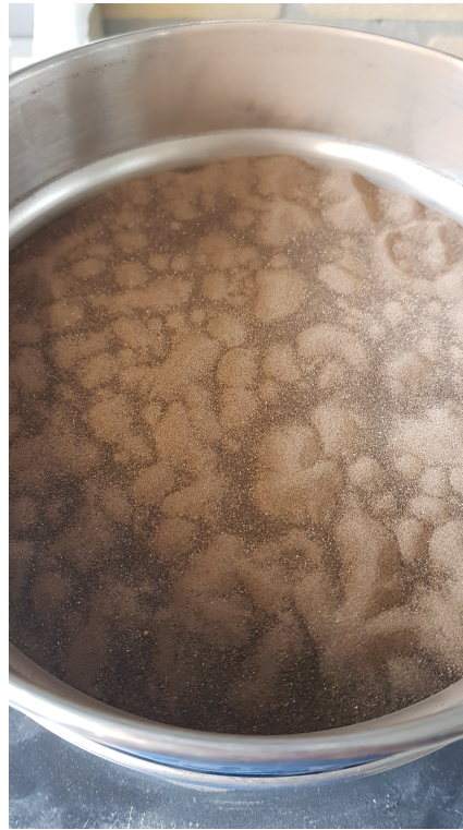
Figure 3.5: Example of material aggregation on a large sieve size. The humps of lighter material are of a smaller particle size than the sieve, but do not pass through easily. Aggravation was necessary to redistribute the cohesive material over the sieve and to sieve again.
