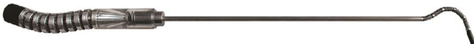
Figure 6.3 Cable-ring mechanism-based Multi-Flex prototype [7, 23, 25] featuring a fully actuated ten DOF tip (excluding tip function), developed within the BITE-group of BioMechanical Engineering Dept., TU Delft.
