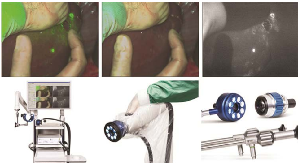
Figure 1.3 Top – Image overlay of the surgical field viewed under visible light and the tumours highlighted by the fluorescent dye and visible under near-infrared light. Bottom – Multispectral medical camera Artemis by Quest for open and minimally invasive surgical applications [25].
