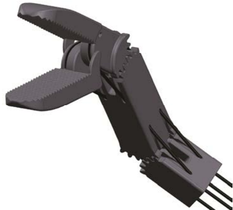
Figure 6.11 Three DOF grasper design showing the jaw flaps and the looped driving cables.
