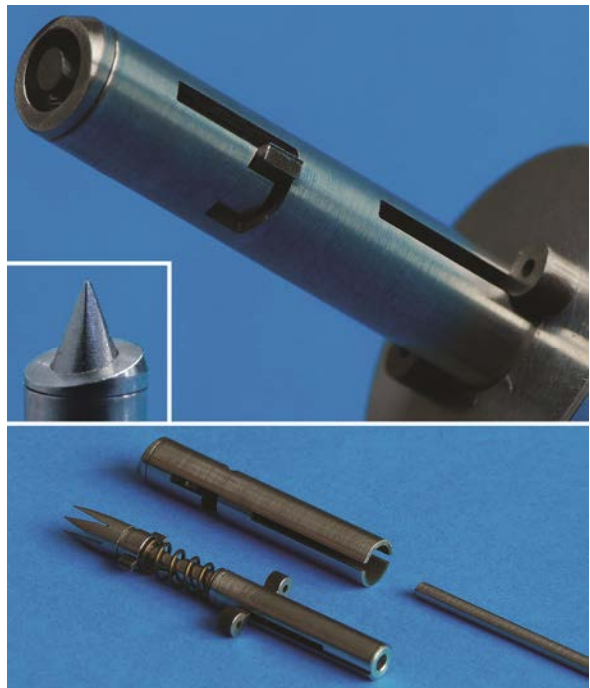
Figure 3.7 Assembled biopsy harvester prototype manufactured nearly at real-scale, \varnothing 6mm, (top) also showing a fully closed crown-cutter (inset). Intermediate assembly (bottom) shows the outer shell, the assembled inner working mechanism and the glass-fibre dummy.
