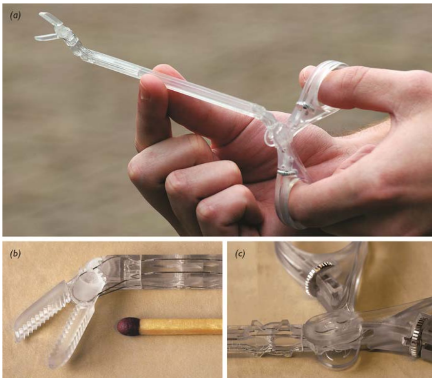
Figure 8.6 (a) New real-scale 5mm wide DragonFlex prototype featuring (b) the optimised rolling joint curvature, no cable-tensioning spring and (c) a smart and simple bolt-and-wheel mechanism for cable clamping and easy tensioning.
