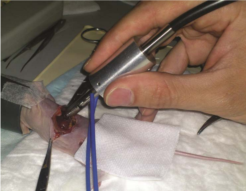
Figure 9.6 In vivo trials on a mouse liver with the experimental biopsy harvester prototype housing a DPS fibre optic cable, showing its potential as a validation device for other optical biopsy technologies.
