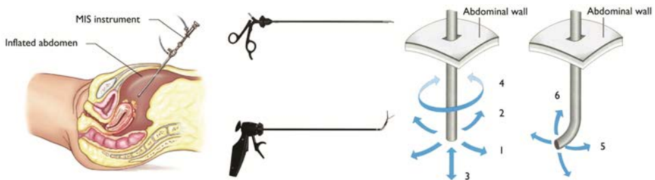
Figure 1.1 Left – Schematic view of laparoscopy [6]. Middle – Rigid [7] & steerable [8] minimally invasive surgical instruments. Right – Rigid instrument DOF [9] and additional steerable tip DOF.
