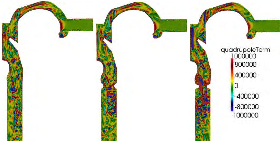
Figure 7.7: Snapshot of the quadrupole source term for the original (left), 50 % constriction (middle) and 75 % constriction (right) SUAM
