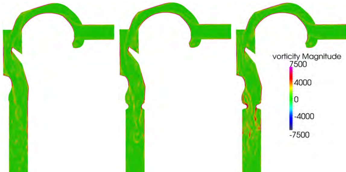
Figure 7.5: Snapshot of the vorticity modulus \|\omega\| for the original (left), 50 % constriction (middle) and 75 % constriction (right) SUAM
