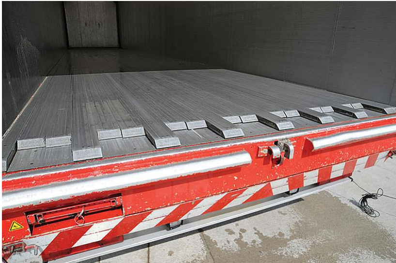
Figure 3.5: Walking floor reclaimer (Image courtesy of Stobart Group Limited)
