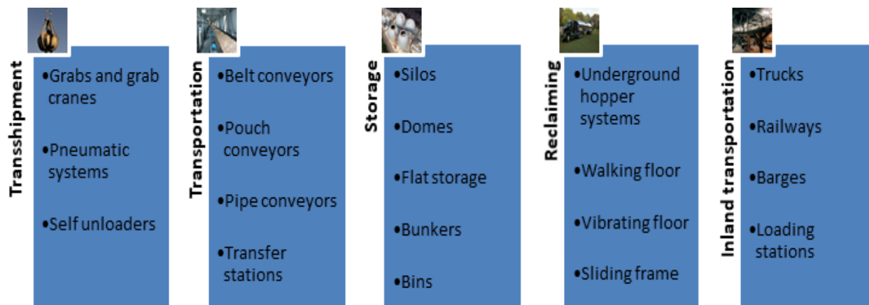
Figure 4.2: Example of solid biomass handling equipment [3]
