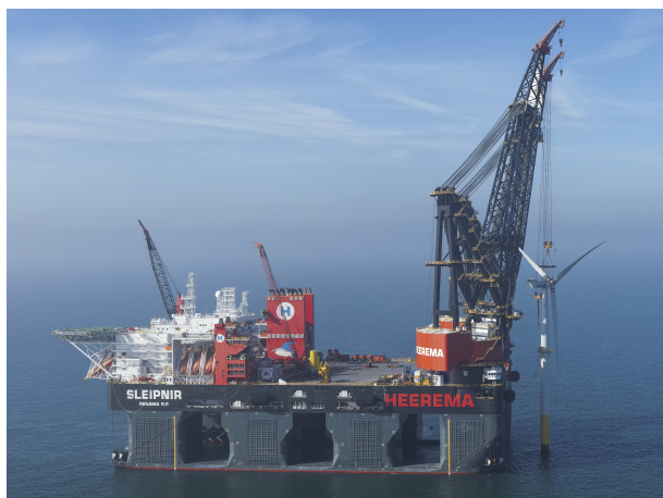
Figure 3.1: Semi-submersible crane vessel Sleipnir of Heerema Marine Contractors performing a floating offshore installation of an OWT [39].
