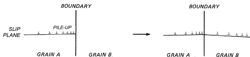
Figure 12.14. Spreading of slip from one grain to another.
