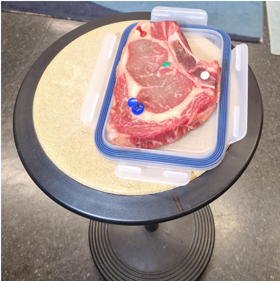
Figure A.8: Anatomical markers tested for visibility in 3D scans, including shiny coloured caps and white plastic caps.
