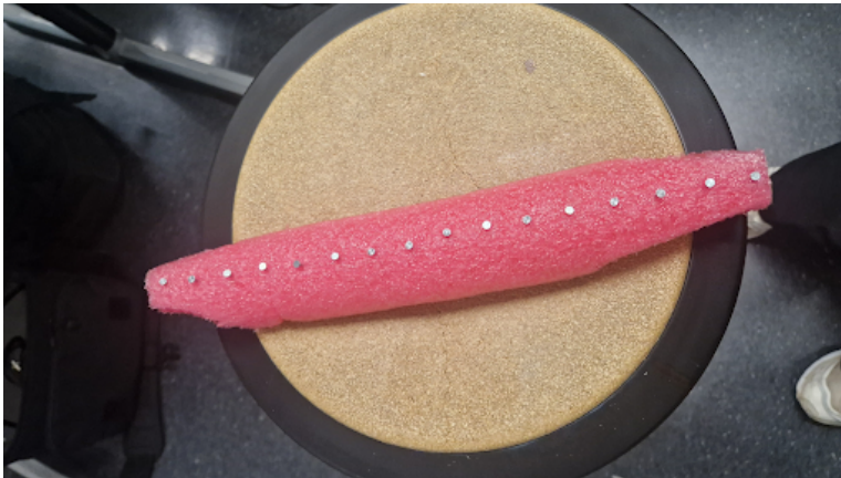
Figure A.5: Pink foam mock-up muscle attached to a skeleton. The shiny surface was intended to mimic the reflective effect of wet muscle tissue. Nails were inserted to simulate fibre length measurements.
