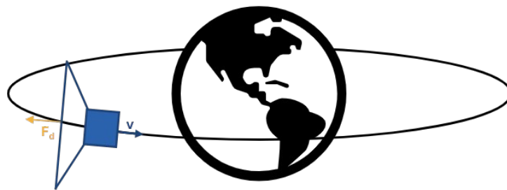
Figure 1.2: Drag sail working principle.
