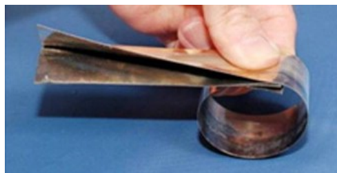
Figure 1.9: Coiled TRAC boom [32].
