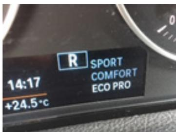
**Figure 5** In some cars, it is possible to adapt it to the preference of the driver by choosing between sport, comfort, and eco.
