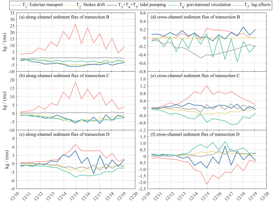
Figure 3.6: Along-channel (left column) and cross-channel (right column) residual sediment flux per unit width of transect B (row 1), C (row 2), and D (row 3). For along-channel flux, positive value indicates seaward transport; for cross-channel flux, positive value indicates transport from the south shoal to the north shoal.
