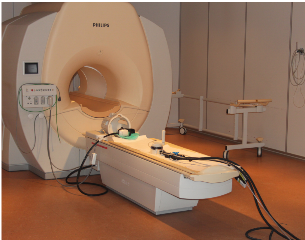
Figure B.13: Photo of the test in an MR-scanner (AMC, Amsterdam). No distortions in the MR-image or distortions in the sensor signal were observed.
