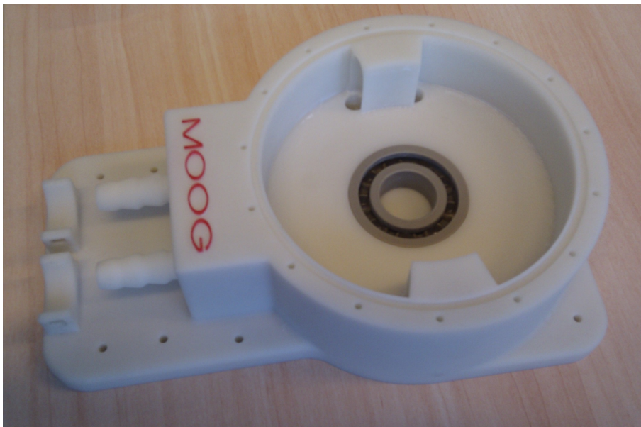
Figure B.6: Photo of the second and last prototype of the vane motor before assembly.
