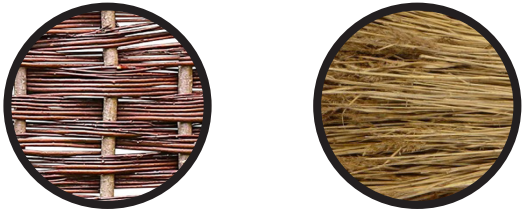
Willow and reed panels south facade sunshading
