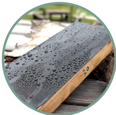
birch bark waterproofing coating
