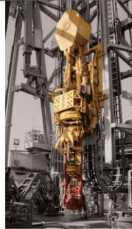
The top drive moves along a set of rails up and down to pick-up the joints from the catwalk shuttle and raise them vertically. After a new joint is connected, the top drive lowers the riser, so that a new joint can be attached. This means the top drive needs to be able to carry the weight of the entire submerged riser.
