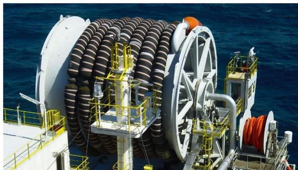
Figure 12: Offloading Reel (Courtesy of Royal IHC)
