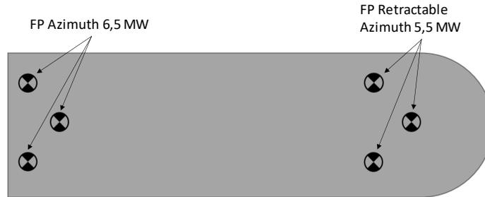
Figure 41: Thruster Arrangement
