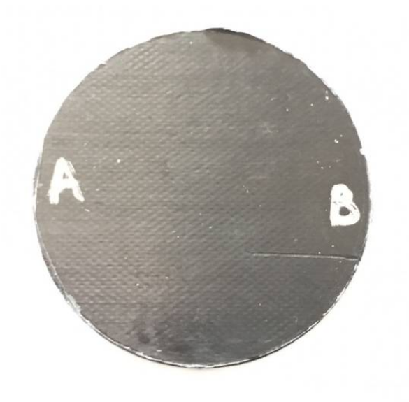
Figure 6.11: Surface quality solid-solid tool panel
