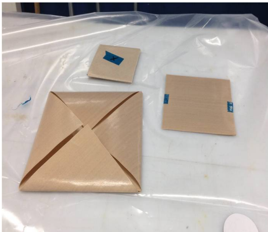
(a) Prepreg stack with teflon covering
