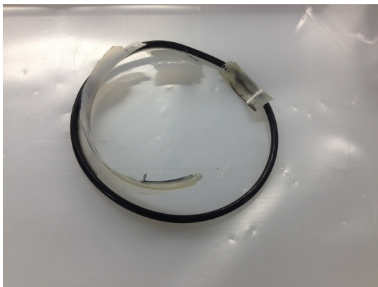
Figure 4.16: Resin leakage during processing in the lower o-ring.
