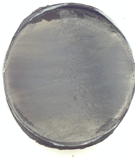
Figure 4.24: Test Panel 4.5: no fiber flow-out
