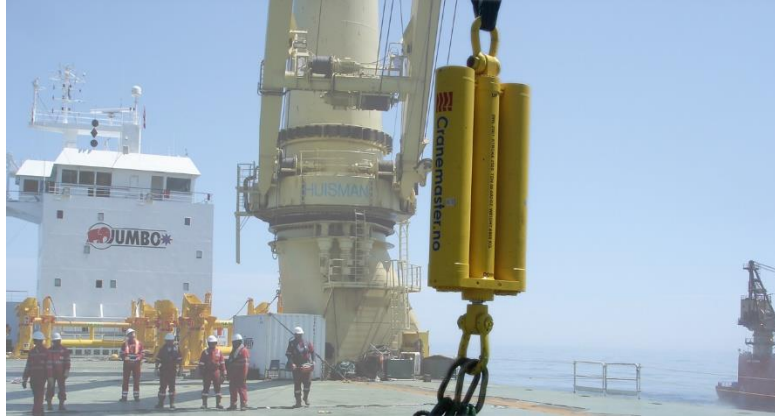
Figure 2.2 One of Jumbo's passive heave compensators during the North Amethyst Project
