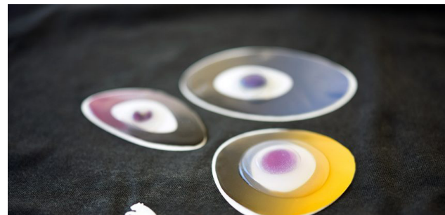
Figure 37. Carbon Eaters contain organisms that change colour in response to changes in air quality (MIT Design Lab, 2018)
