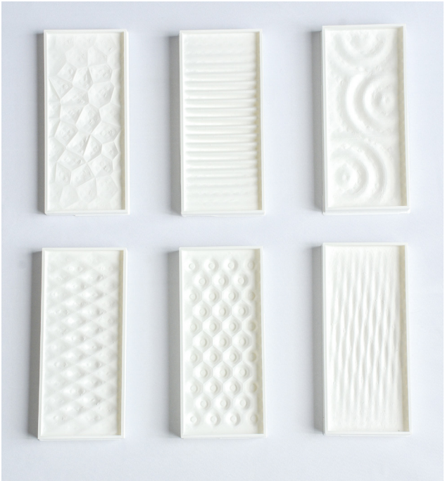
Figure 84. Six 3D print molds.
