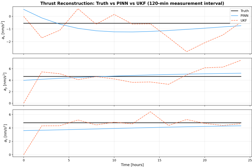
Figure 6.29: Thrust Reconstruction Timeseries Comparing the PINN and the Augmented UKF With 120-Minute Sampling
