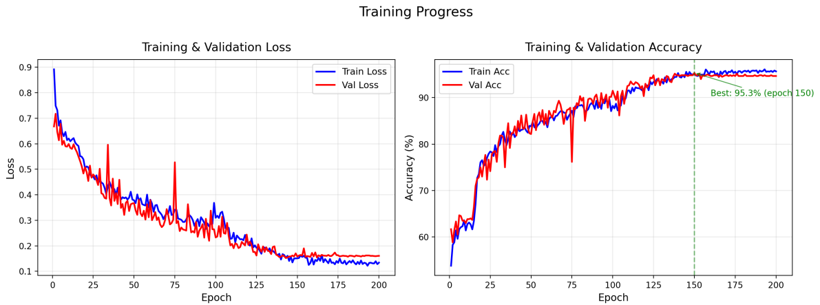
Figure 6.3: Training and Validation Loss (left) and Accuracy (right) Curves for the LSTM Classifier
