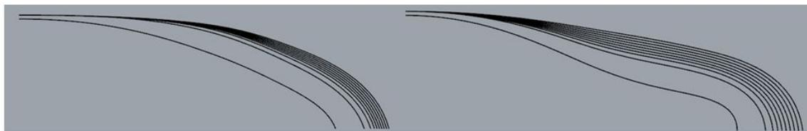
**Figure 5-10:** Waterlines plans of bow 125 (left, good resistance characteristics) and bow 65 (right, poor resistance characteristics)
