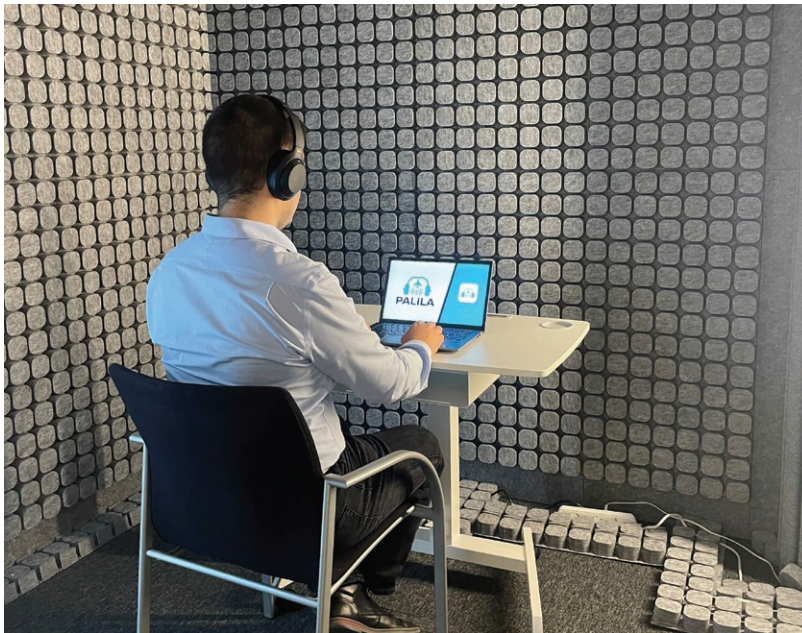
Figure 6.1. Laboratory setup used for the listening experiment on noise annoyance. Source: Roberto Merino-Martínez
