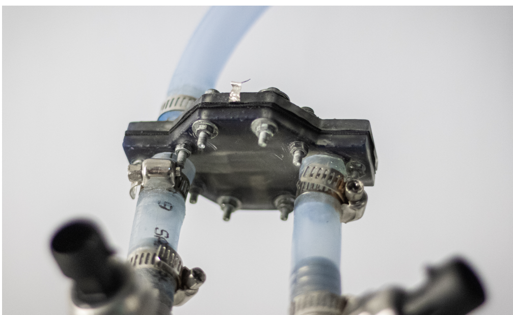
Figure 3.4: Assembled electrolyzer on its side with the silicon tubes connected. The exploded view of this electrolyzer's 3D render is shown in Fig. 3.3
