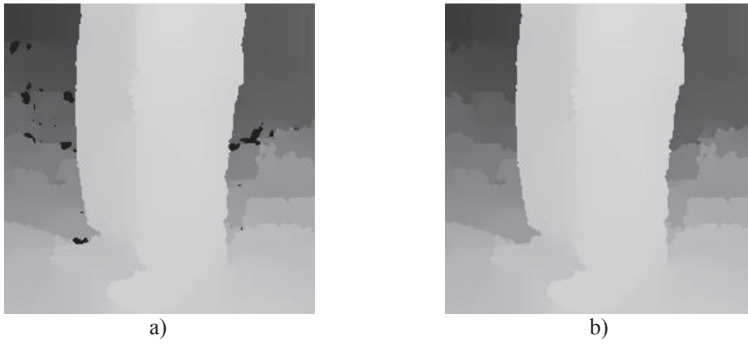
Figure 3.7: Disocclusion inpainting for depth maps : a) Depth after median filtering, b) Depth after filling disocclusions
