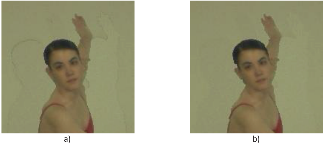
Figure 3.9: Dilation : a) Ghost contours in the absence of dilation, b) Ghost contours erased by dilation
