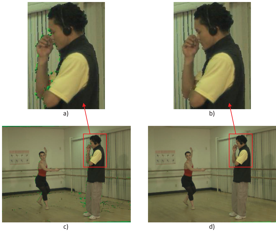
Figure 3.11: Disocclusion inpainting for texture maps : a) Before inpainting (closer look), b) After inpainting (closer look), c) Before inpainting, d) After inpainting - final interpolated view
