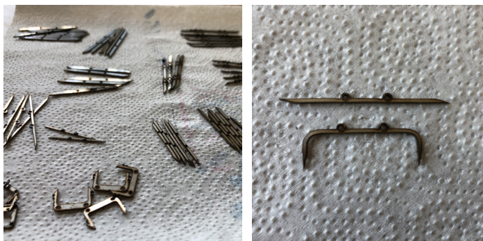
Figure 74: Staples produced on a CO2 laser cutter, 1:10 scale
