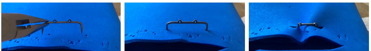
Figure 76: Staple with straight legs squishing the material
