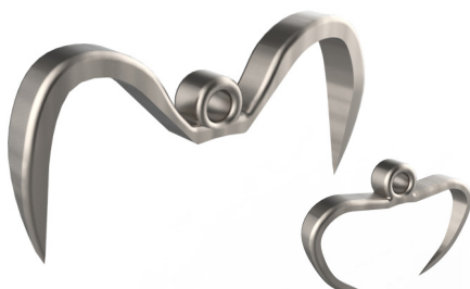
Figure 70: Final staple shape (open and closed)
