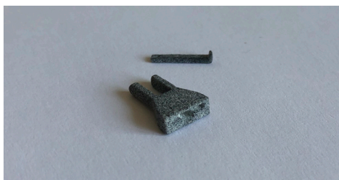
Figure 81: SLS printed parts
