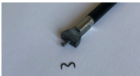
Figure 82: Device with hook, manual insertion of the staple
