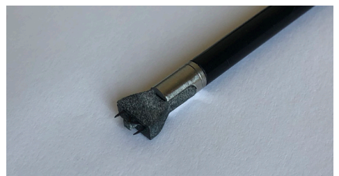
Figure 82: Device with hook, manual insertion of the staple
