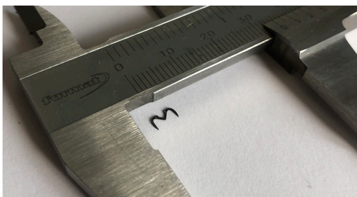
Figure 77: Staples produced on a UV laser (1:1 scale). The suture is 0.3 mm thick and fits through the 0.35 mm holes (right)
