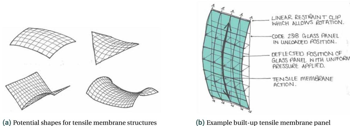
**Figure 2.5:** Possibilities for thin glass tensile membrane panels (Lambert and O'Callaghan, 2013)
