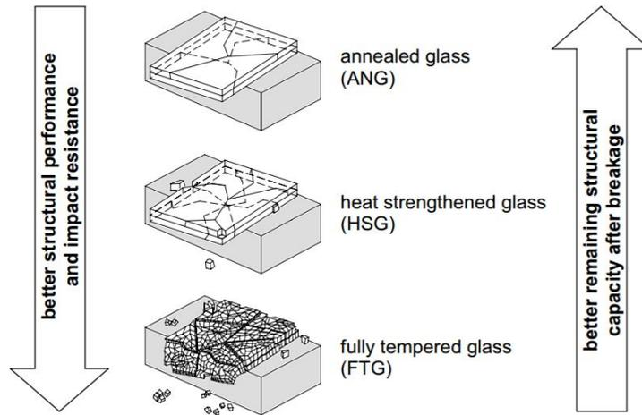
Figure 4.4: Breakage pattern of annealed, heat strengthened and toughened glass (Haldimann et al., 2008)
