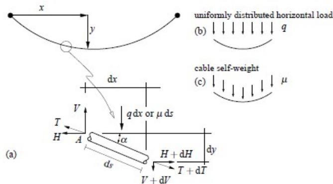
Figure B.8: Forces in parabolic cable and catenary (Simone, 2011)
