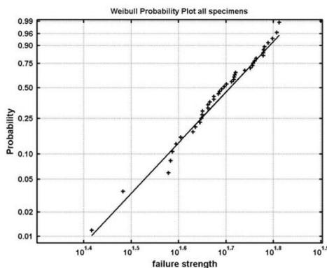
Figure 8.2: Weibull plot of bending tensile strength (Veer et al., 2007)
