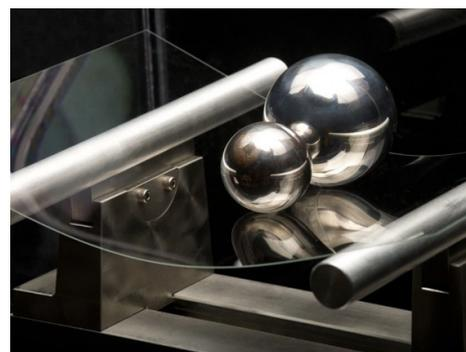
**Figure 2.2:** Demonstration of the flexibility of thin glass [Photography by Corning]
