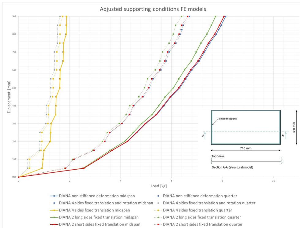
Figure 9.10: Resulting graph of the displacements at midspan and a quarter for the adjusted support models
