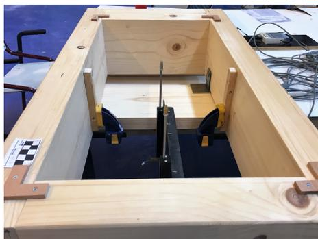
(a) Wooden frame with linear potentiometers
