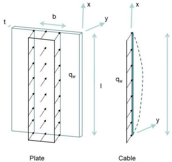
Figure B.9: Simplification of façade structure to cable
