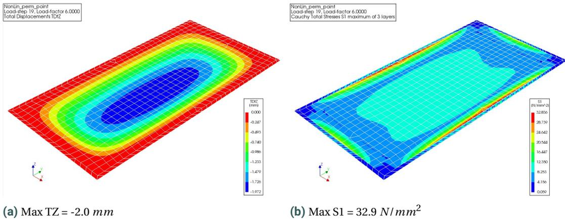
Figure G.2: Contour plot load-step 19 non-linear analysis 4 edges fixed translations
