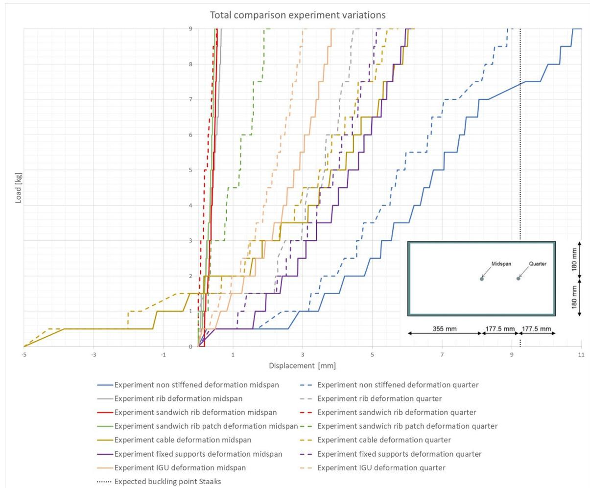
**Figure 9.15:** Resulting graph of the displacements at midspan and a quarter for the executed experiments
