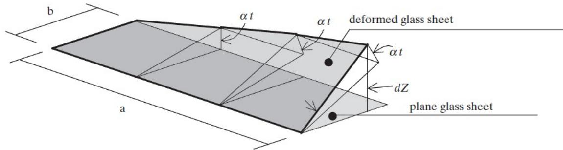
**Figure B.6:** Definition parameters belonging to equation B.5 (Hoogenboom, 2004)
