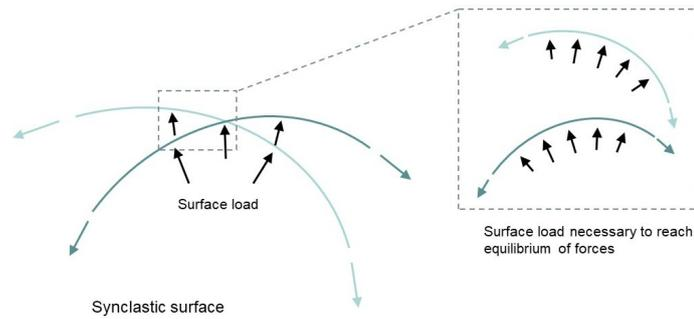
**Figure B.1:** Force distribution in a synclastic membrane
