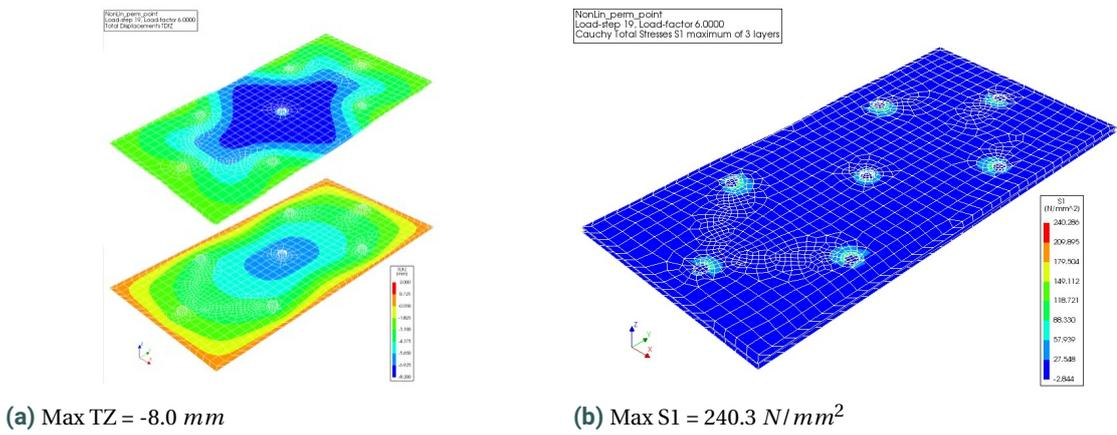
**Figure G.9:** Contour plot load-step 19 non-linear analysis sandwich TSSA variation
