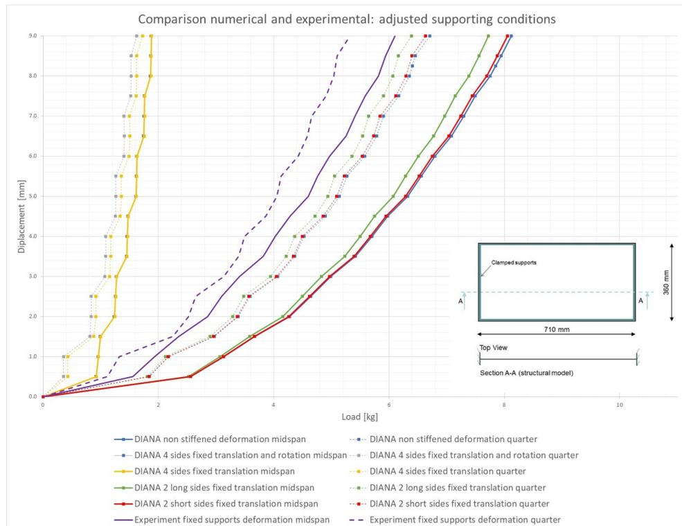
**Figure 9.17:** Resulting graph of the displacements at midspan and a quarter for the executed clamped plate experiment and the related FE models
