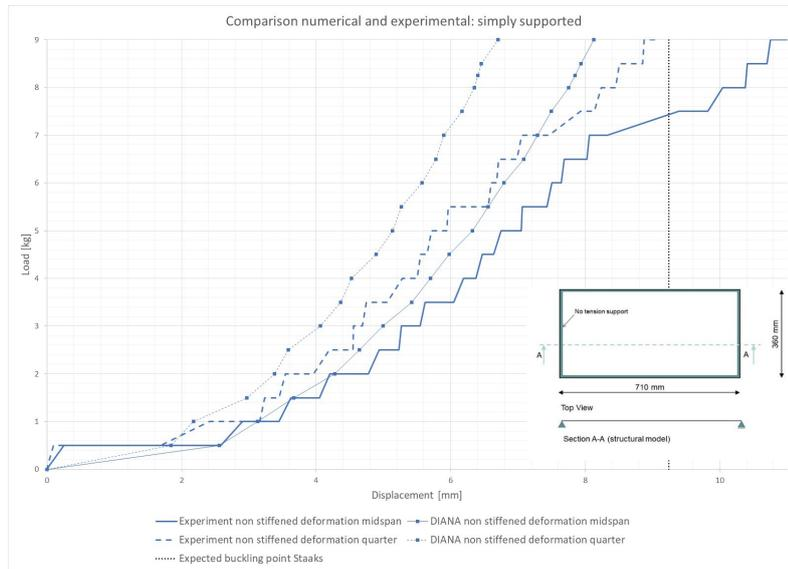
**Figure G.11:** Resulting graph of the displacements at midspan and a quarter for the executed simply supported experiment and the related FE model
