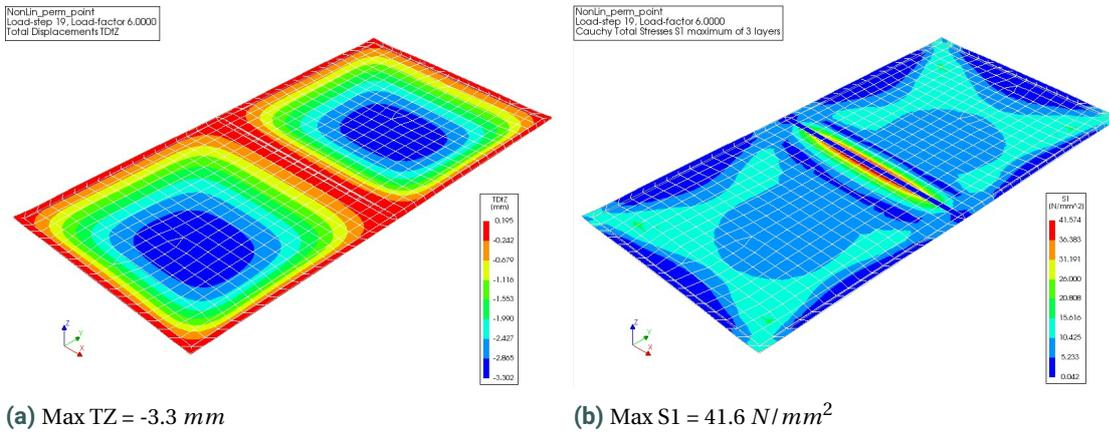
Figure G.5: Contour plot load-step 19 non-linear analysis rib variation
