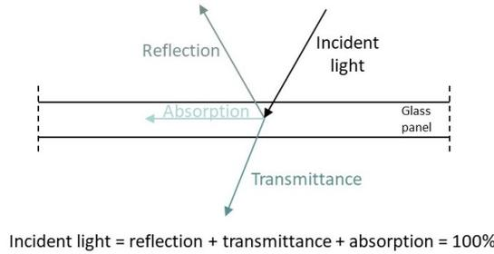
**Figure 7.2:** Illustration of light transmittance glass panel
