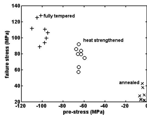
Figure 8.3: Relation between pre-stress and failure stress (Veer et al., 2009)
