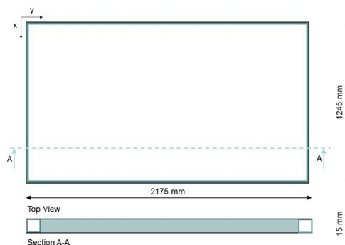
**Figure 11.3:** Geometry of full scale IGU panel
