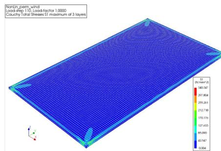
Figure 11.6: Maximum principal stresses S1 in panels = 340.347 N/mm<sup>2</sup>
