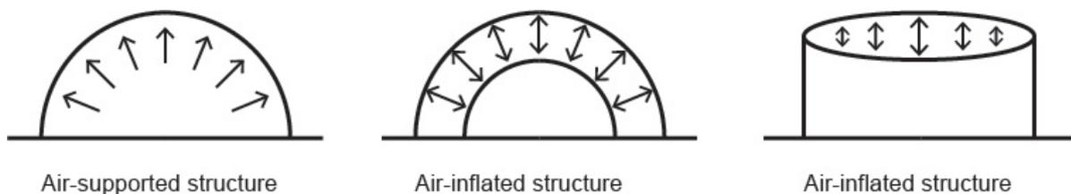
**Figure 2.3:** Difference between an air-supported and air-inflated structure
