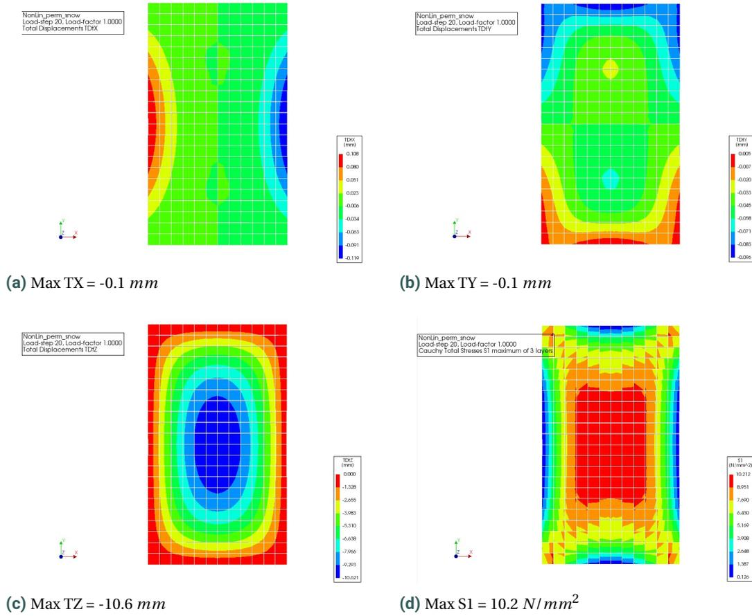
**Figure E.2:** Results non-linear analysis reference model load combination Permanent + Snow
