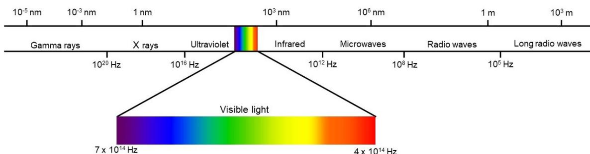
Figure 5.1: Electromagnetic spectrum
