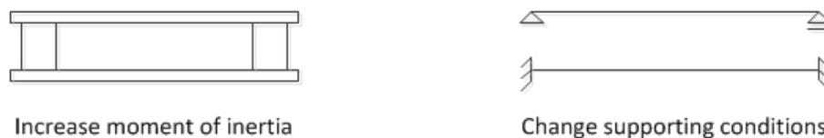
**Figure 2.6:** Stiffening flat plate: left increasing moment of inertia, right change supporting conditions
