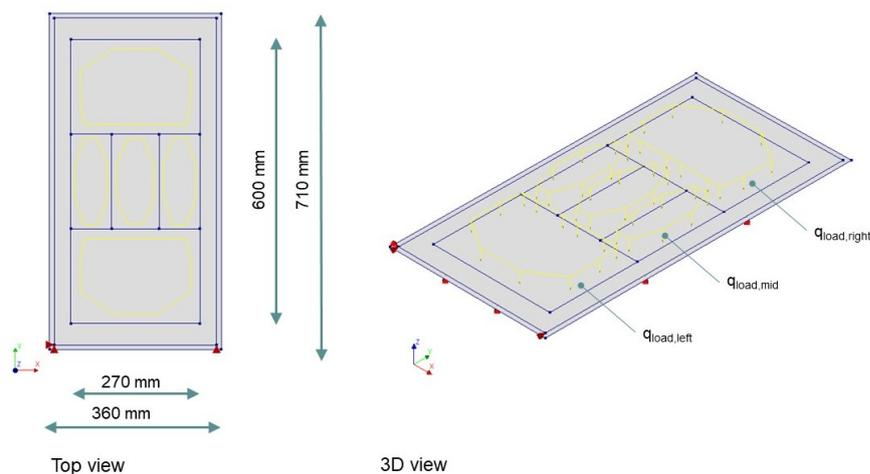
**Figure 9.6:** Overview of the geometry and loads of the variation models
