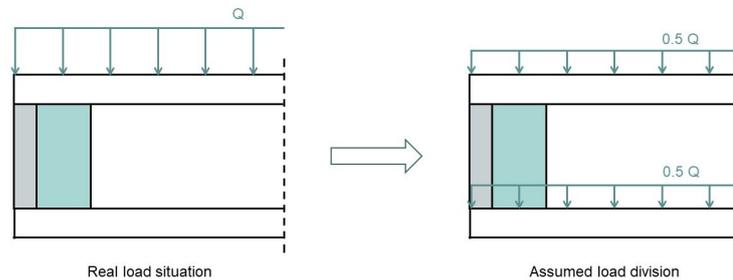
**Figure 11.2:** Left: real load situation of IGU under an external load. Right: assumed load situation of IGU by cooperation panels due to hermetically sealed air layer
