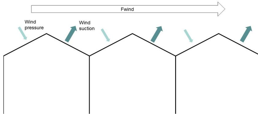
Figure D.1: Wind pressure and suction on a Venlo greenhouse system
