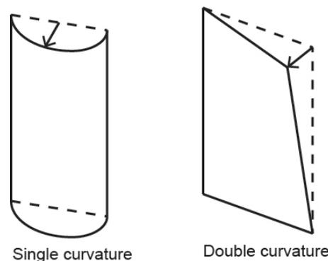
**Figure 2.4:** Single curvature vs. double curvature thin panel
