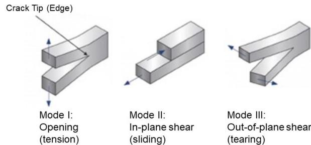
**Figure 8.1:** Visualisation of three possible crack modes, image adjusted from Pepi (2002)
