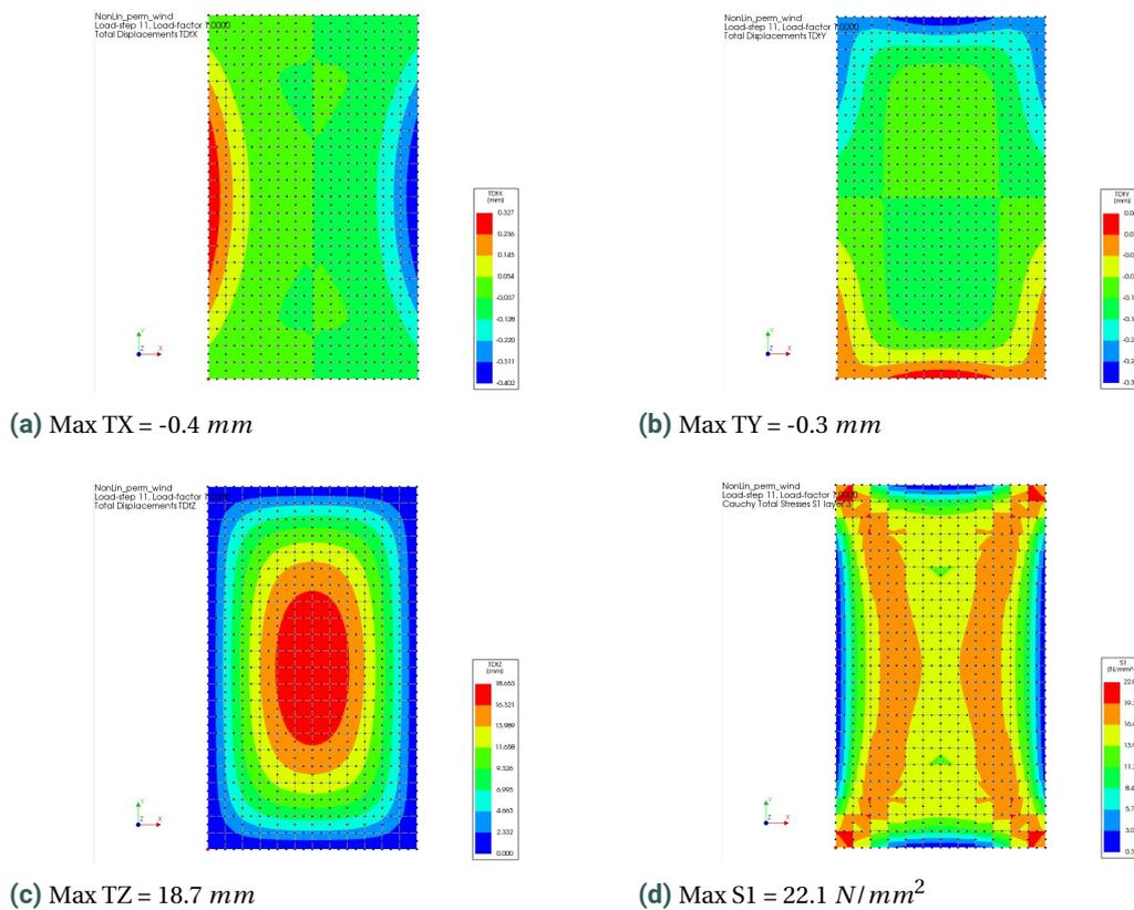
**Figure 9.3:** Results non-linear analysis reference model
