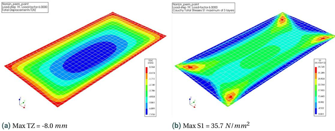
Figure G.3: Contour plot load-step 19 non-linear analysis 2 long edges fixed translations
