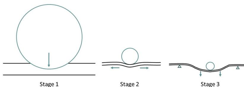
**Figure 8.7:** Visualisation of three stages during hail impact on a sheet
