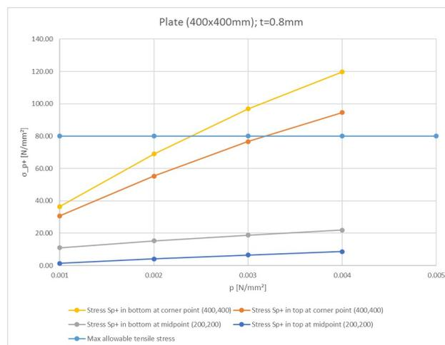
**Figure B.4:** Results stresses Mepla analysis plate 400 x 400 mm and t=0.8 mm
