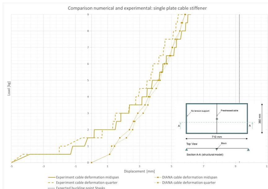
**Figure G.14:** Resulting graph of the displacements at midspan and a quarter for the executed single plate with cable stiffener experiment and the related FE model
