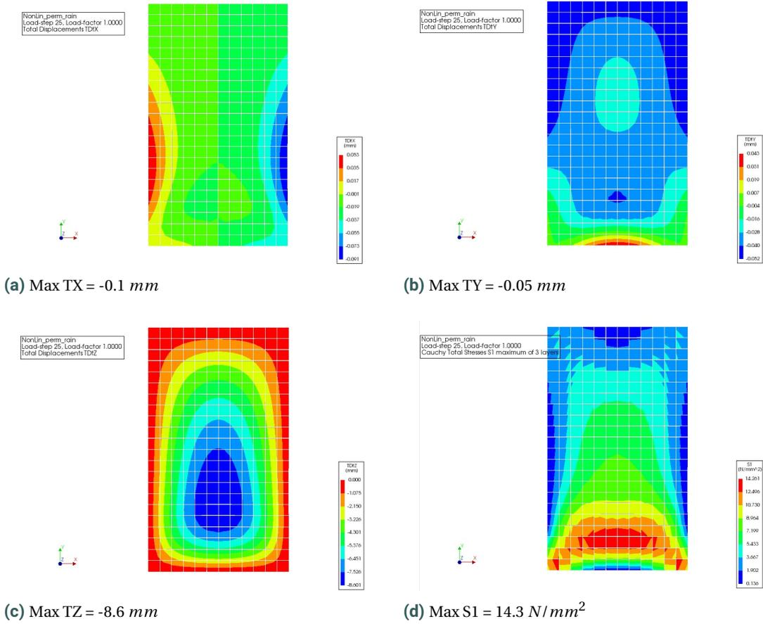
Figure E.3: Results non-linear analysis reference model load combination Permanent + Rain
