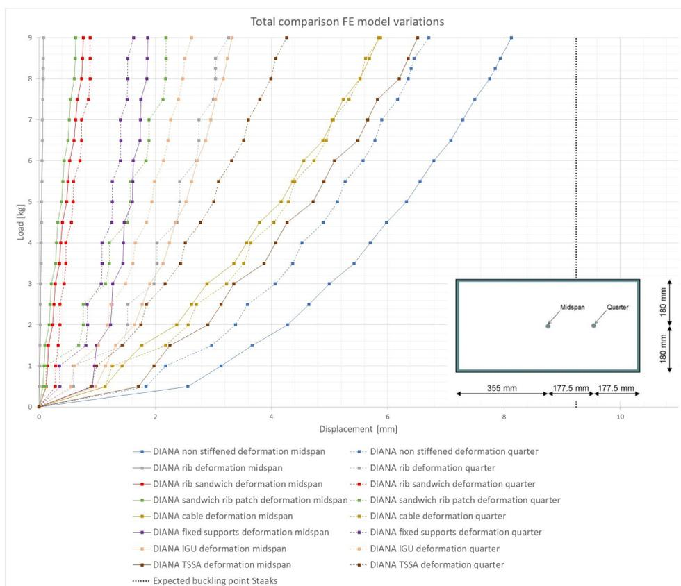
Figure 9.11: Resulting graph of the displacements at midspan and a quarter for the stiffened variation models
