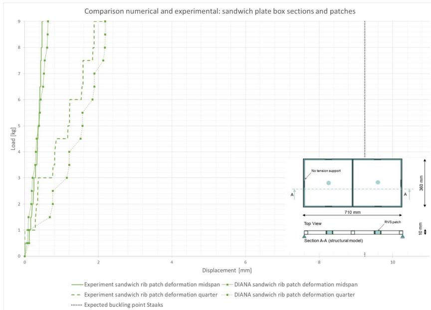
**Figure G.16:** Resulting graph of the displacements at midspan and a quarter for the executed sandwich with rib stiffeners and patches experiment and the related FE model
