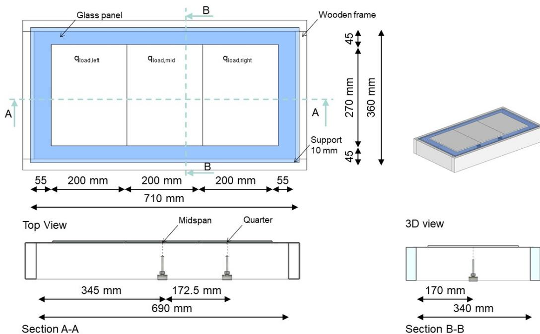
Figure F.1: Drawing of test set-up
