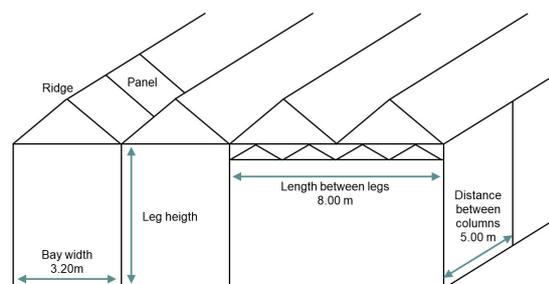
**Figure 5.4:** Typical build up of a Venlo system
