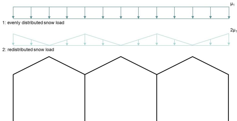
**Figure D.2:** Difference between evenly distributed and redistributed snow load
