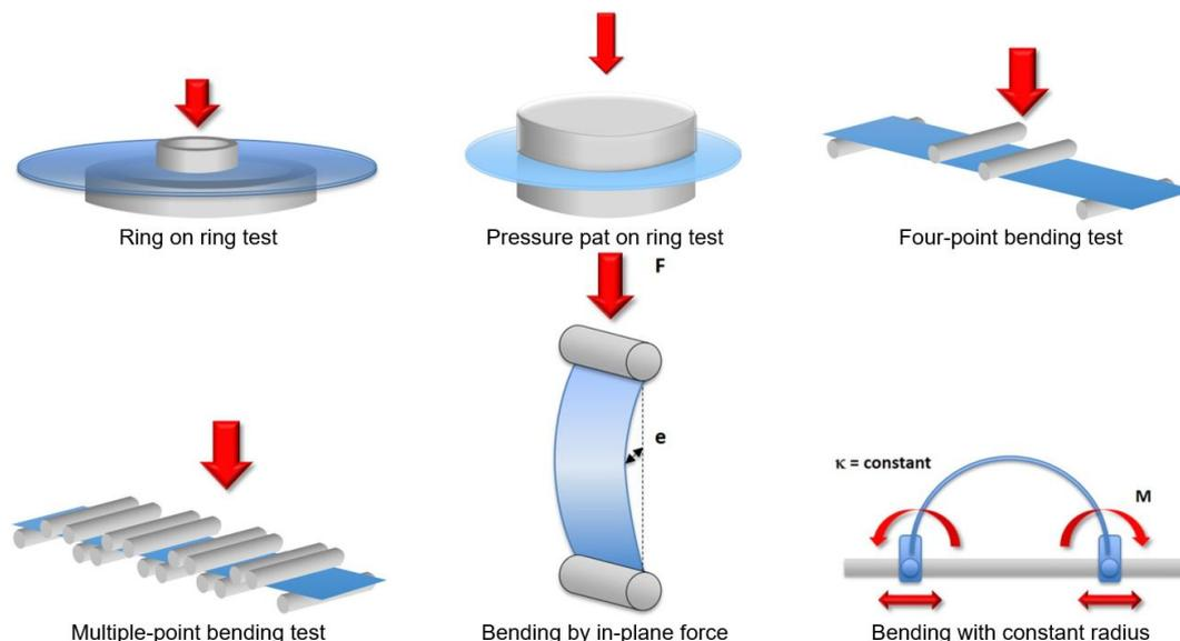
Figure 8.5: Visualisation of possible test configurations, image adjusted from Neugebauer (2016)
