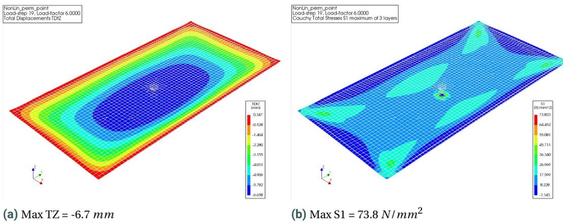
Figure G.6: Contour plot load-step 19 non-linear analysis cable variation
