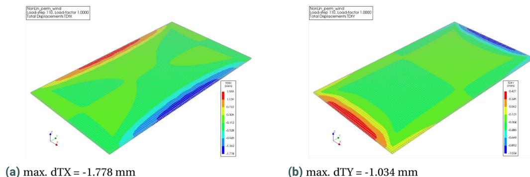
Figure 11.4: In-plane deformation results numerical analysis
