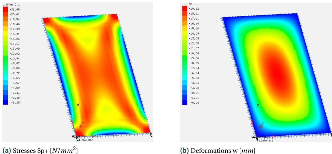
Figure B.12: Results of Mepla analysis for  $t=4$  mm
