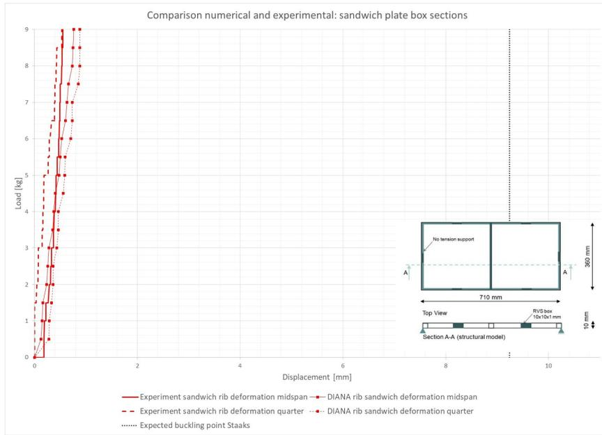
**Figure G.15:** Resulting graph of the displacements at midspan and a quarter for the executed sandwich with rib stiffeners experiment and the related FE model
