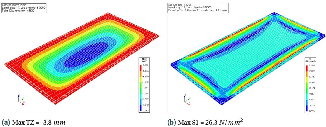
**Figure G.10:** Contour plot load-step 19 non-linear analysis insulated glass panel
