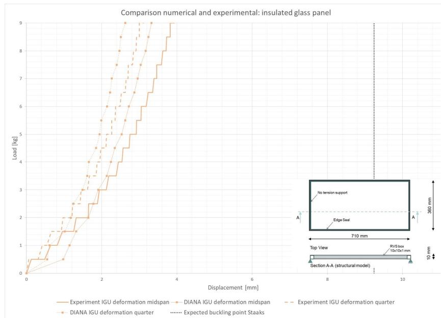
**Figure G.17:** Resulting graph of the displacements at midspan and a quarter for the executed insulated glass unit experiment and the related FE model
