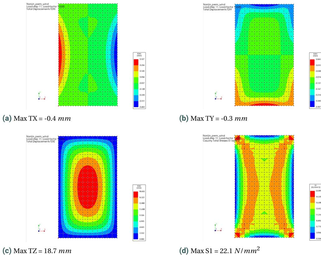
Figure E.1: Results non-linear analysis reference model load combination Permanent + Wind
