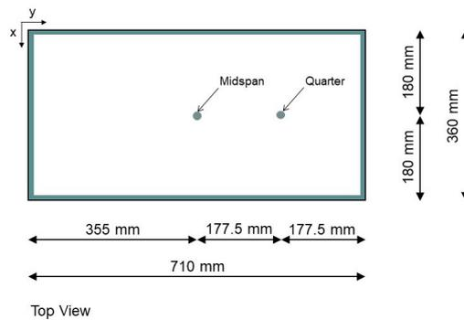
Figure 9.7: Overview of the measurement locations for the variation study
