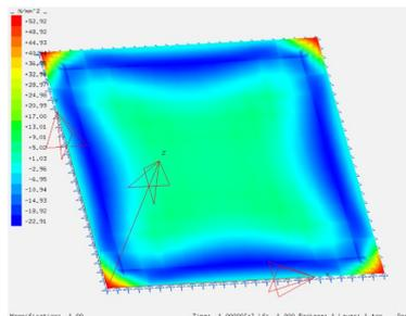
**Figure B.2:** Stresses  $S_{p+}$  [ $N/mm^2$ ]
