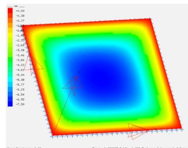
**Figure B.3:** Deformations  $w$  [ $mm$ ]
