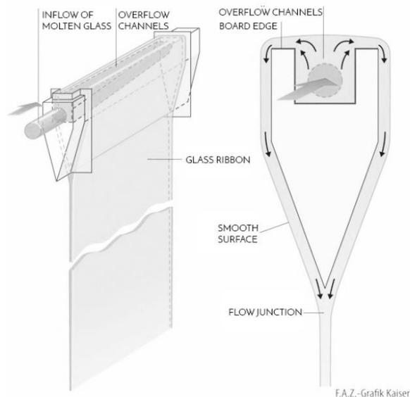
Figure 4.3: Overview of the overflow-fusion process (Silveira, 2016)
