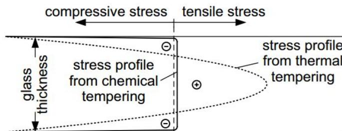
Figure 4.5: Residual stress profiles obtained by thermal and chemical strengthening (Haldimann et al., 2008)
