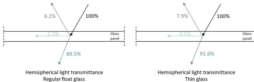
**Figure 7.3:** Visualisation of hemispherical light transmittance regular float glass and thin glass panel
