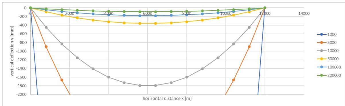
Figure B.10: Deflection of a parabolic cable with horizontal pretension variation from 1,000 N to 200,000 N
