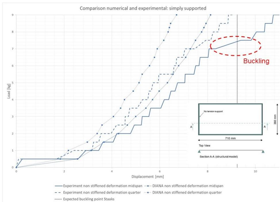
**Figure 9.16:** Resulting graph of the displacements at midspan and a quarter for the executed simply supported experiment and the related FE model
