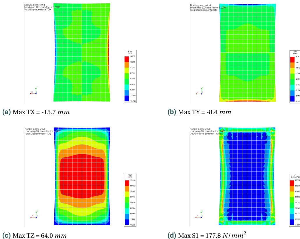
Figure 9.4: Results non-linear analysis thin glass model
