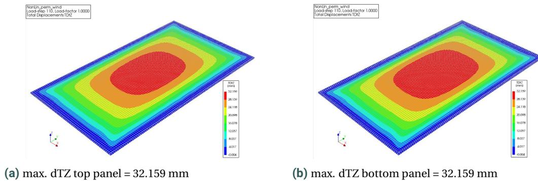
Figure 11.5: Out-of-plane deformation results numerical analysis
