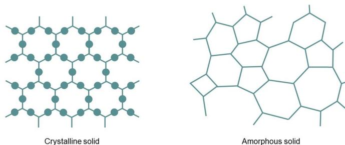
**Figure 4.1:** Structures of a crystalline solid (left) and an amorphous solid (right)
