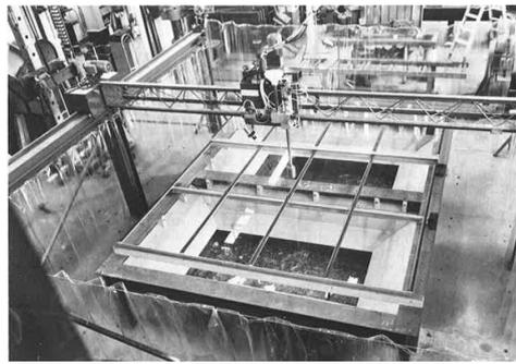
**Figure 8.6:** Measurement set-up used for the hail impact research by TNO (KRI-TNO et al., 1984)
