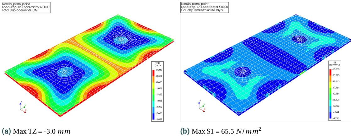
**Figure G.8:** Contour plot load-step 19 non-linear analysis sandwich rib patch variation
