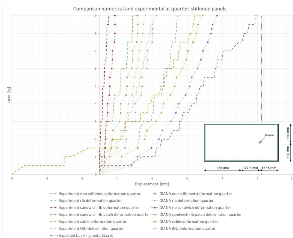
Figure 9.19: Resulting graph of the displacements at quarter for the executed stiffened panels experiments and the related FE models
