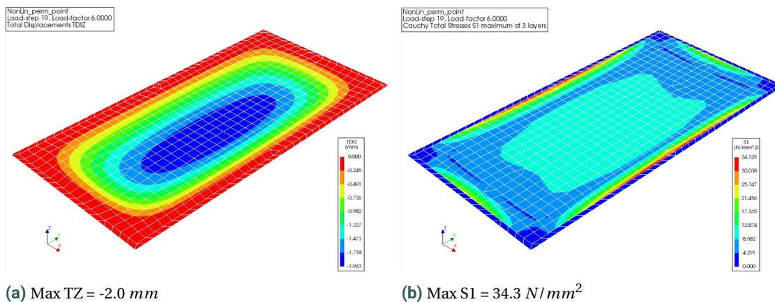
Figure G.1: Contour plot load-step 19 non-linear analysis 4 edges fixed translations and rotations
