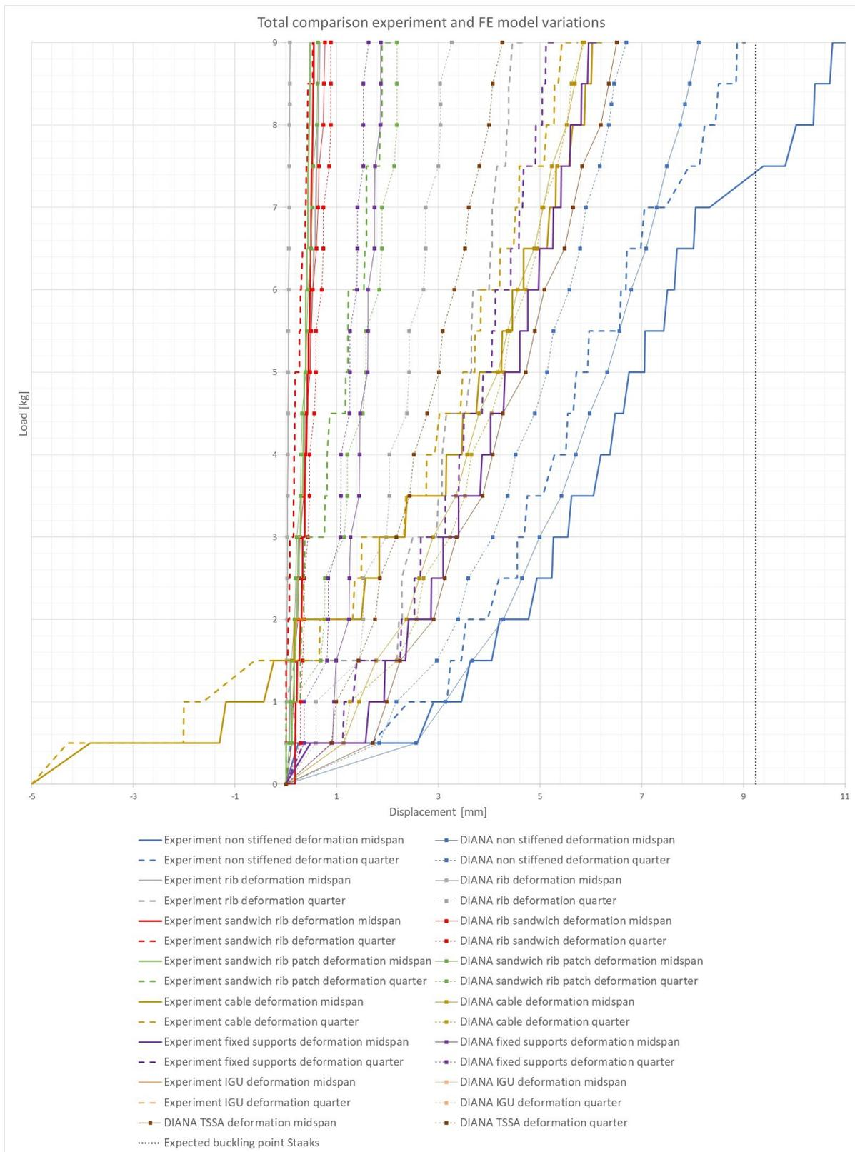
Figure G.18: Resulting graph of the displacements at midspan and a quarter for the all executed experiments and the related FE models
