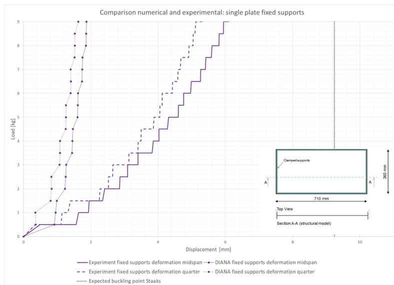
**Figure G.12:** Resulting graph of the displacements at midspan and a quarter for the executed single plate with fixed edges experiment and the related FE model
