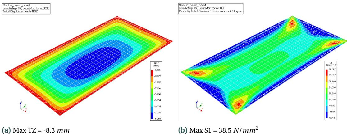
Figure G.4: Contour plot load-step 19 non-linear analysis 2 short edges fixed translations
