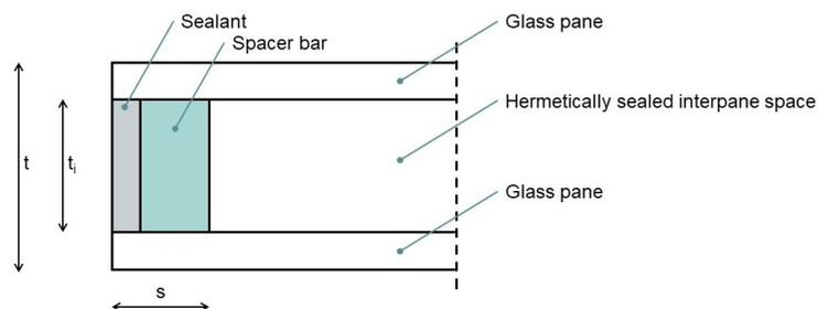
Figure 11.1: Visualisation of typical geometry IGU
