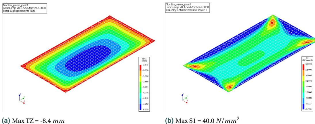
Figure 9.8: Results non-linear analysis simply supported reference model (total load is 9 kg)
