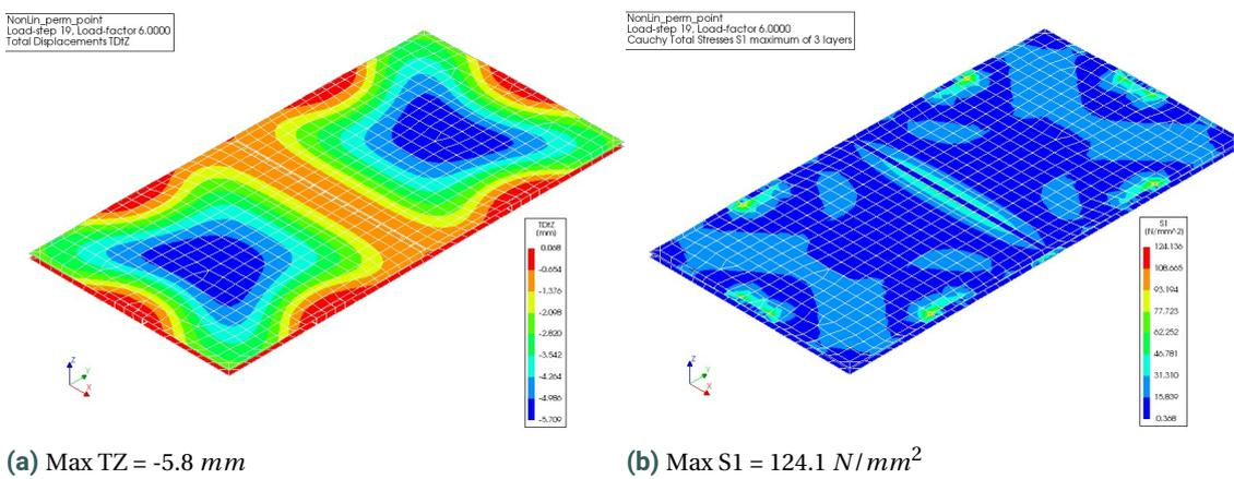
Figure G.7: Contour plot load-step 19 non-linear analysis sandwich rib variation
