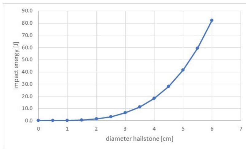
**Figure D.3:** Relation between diameter of hail stone and the impact energy
