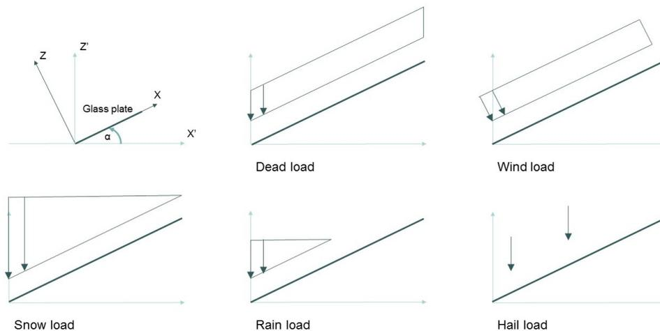
**Figure 9.1:** Visualisation of the directions of the different loads on the glass panel in the reference greenhouse system
