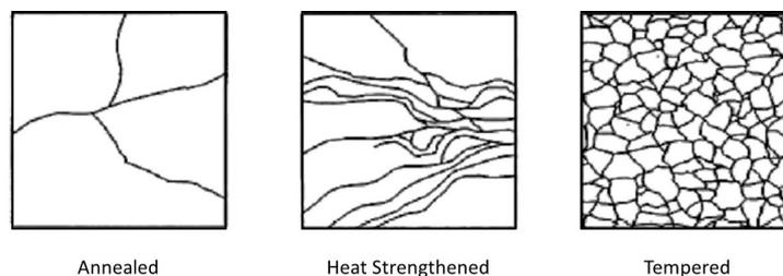
**Figure 8.4:** Breakage pattern of various pre-stressing methods of glass
