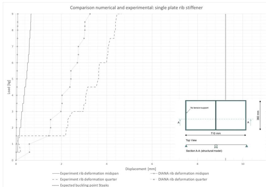
**Figure G.13:** Resulting graph of the displacements at midspan and a quarter for the executed single plate with rib stiffener experiment and the related FE model
