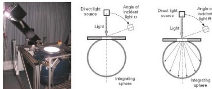
**Figure 7.1:** Schematic overview measurement system for hemispherical and perpendicular light transmittance (Hemming et al., 2014)
