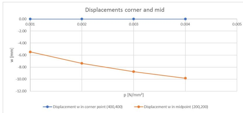
Figure B.5: Results displacements Mepla analysis plate 400 x 400 mm and t=0.8 mm
