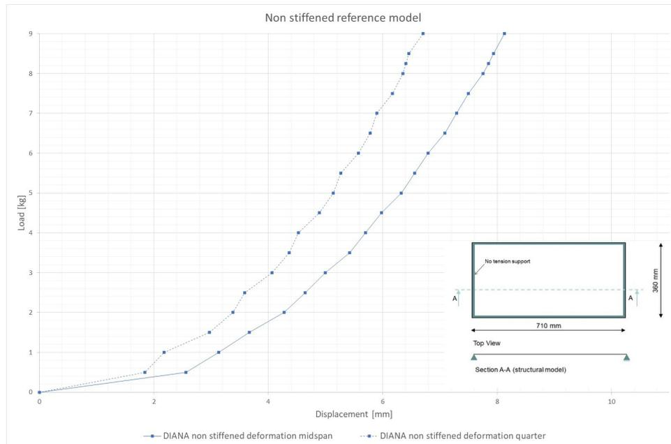
**Figure 9.9:** Resulting graph of the displacements at midspan and a quarter for simply supported reference model
