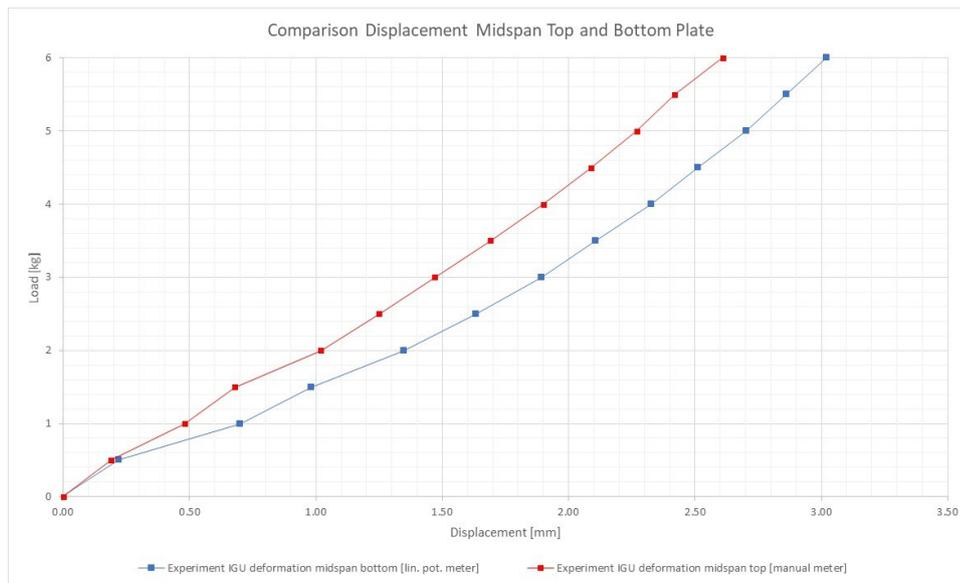
**Figure F.11:** Resulting graph of the displacements at midspan for the executed stiffened panels experiments and the related FE models
