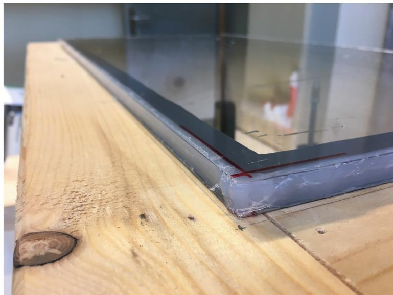
**Figure F.10:** Close-up of sealed edge of IGU panel
