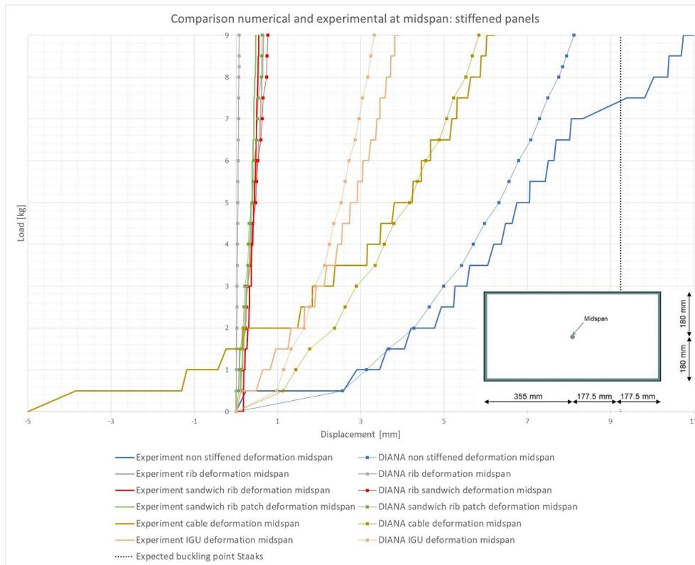
Figure 9.18: Resulting graph of the displacements at midspan for the executed stiffened panels experiments and the related FE models
