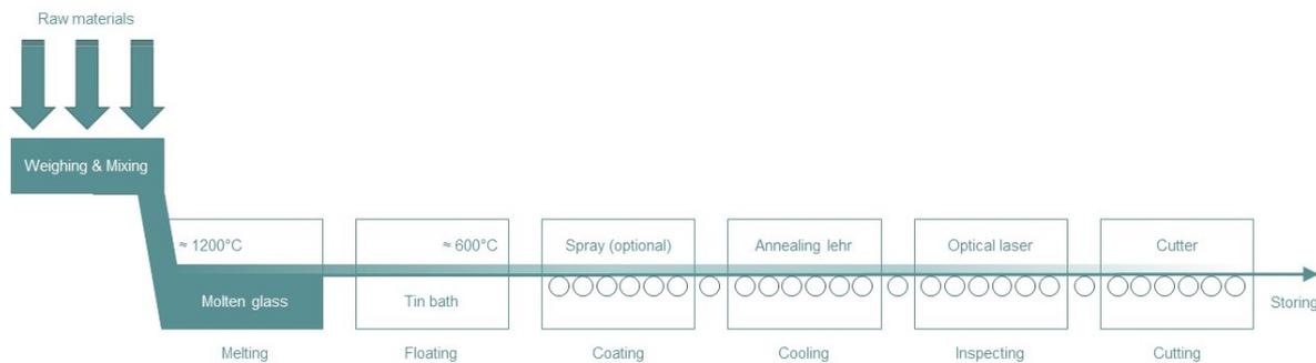
Figure 4.2: Visualisation of the Pilkington production process for float glass
