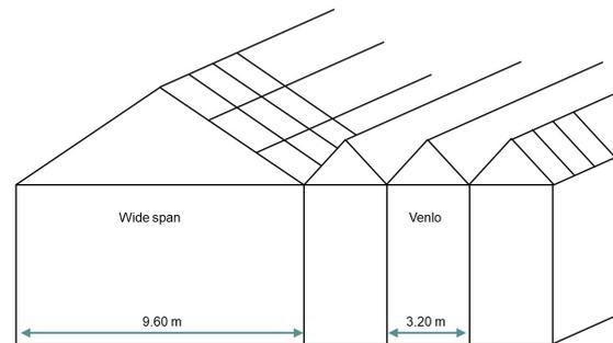
**Figure 5.6:** Comparison of the build up of a Widespan and Venlo greenhouse system
