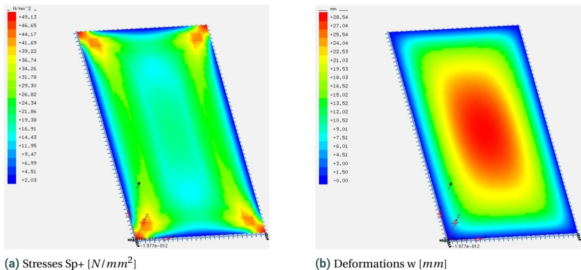
Figure B.13: Results of Mepla analysis for  $t=2.5$  mm
