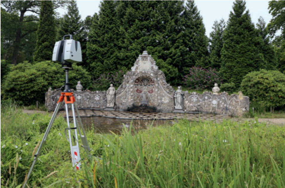
[FIG. 15] Employing a field instrument, a terrestrial laser scanner, to create a digital point cloud of the shell gallery in the park of Rosendael Castle. This technology can be used to create a detailed digital copy of architectural and natural features for study and monitoring. (Photo: Steffen Nijhuis, TU Delft)
