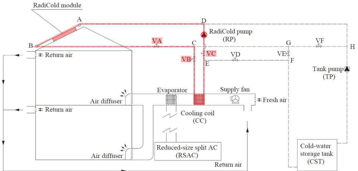
Figure 3-4. First operation mode (Direct space cooling) of the system of Zhang *et al.* (2018). Valves VA, VB and VC are open. In this mode the RSAC could be operating or not.
