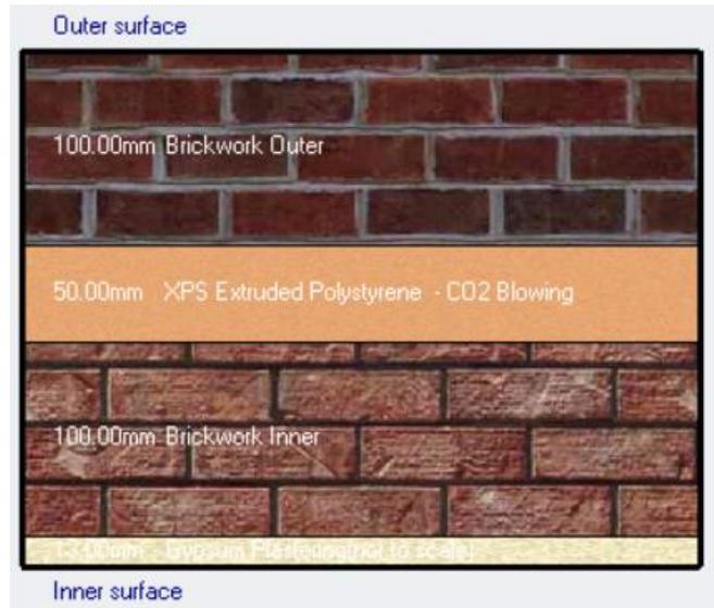
Figure 6-3. Cross-section of the external walls structure, from DesignBuilder.
