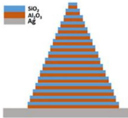
Figure 2-7. The all-dielectric micropyramid structure Introduced by Wu *et al.* (2018).
