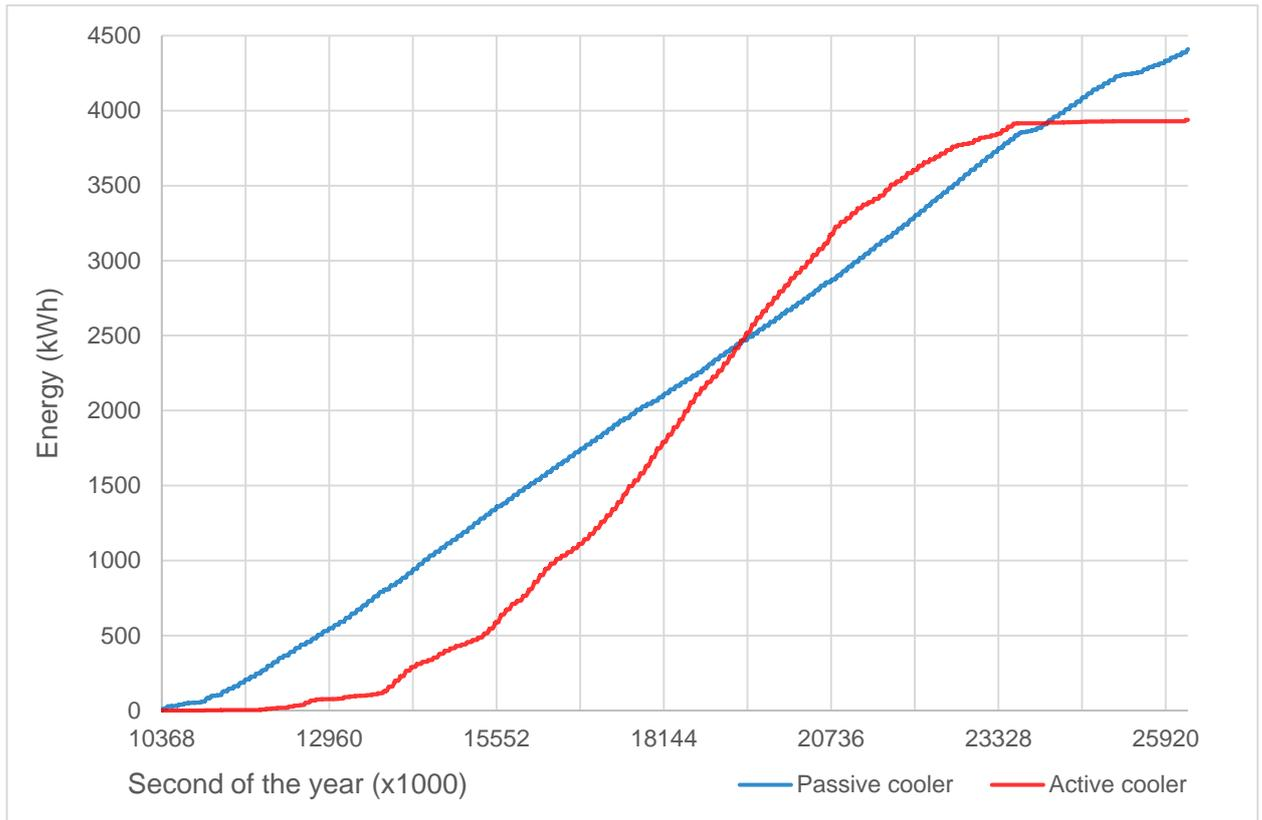
Figure 7-8. Cooling energy provided by the passive cooler and the active cooler for the six-month period for the base case scenario.
