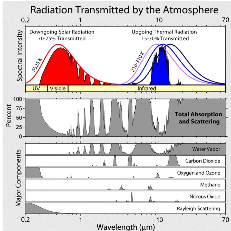
Figure 2-3. The amount of thermal radiation absorbed or scattered by the several gasses of the atmosphere between 0.2 and 70  $\mu\text{m}$ . The infrared window exists between 8 and 13  $\mu\text{m}$  (Wilson *et al.*, 2012).
