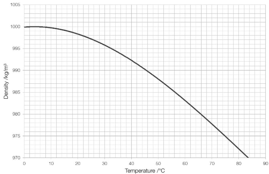
Figure 3-7. The density of water plotted against its temperature.
