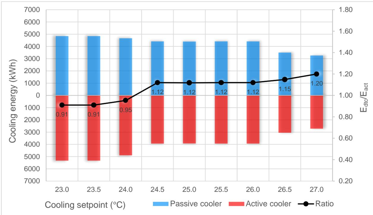
Figure 7-21. The sensitivity of the system to the cooling setpoint temperature of the dwelling.
