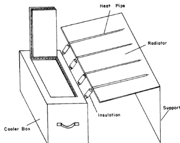
Figure 3-2. The closed loop water based system designed by Ezekwe (1990).
