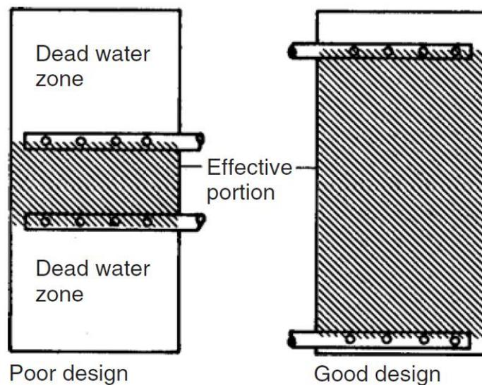
Figure 3-8. A poor and a good design of a water energy storage tank and the effective water portion in each case (Dincer and Rosen, 2011).
