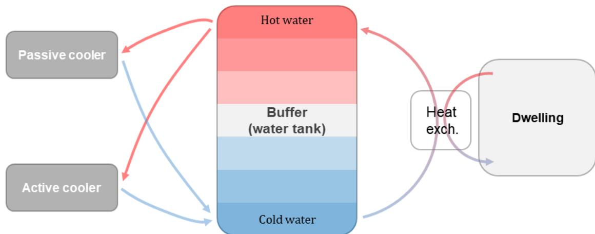
Figure 5-1. A simplified diagram of the proposed hybrid cooling system (Mode 1).
