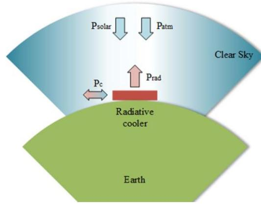
Figure 2-4. Gains and losses of a daytime radiative cooler (Zeyghami *et al.*, 2018).
