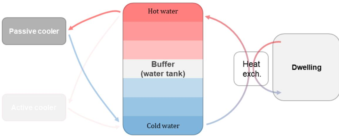
Figure 5-2. Mode 2 of the proposed system; when only the passive cooler provides cooled energy.
