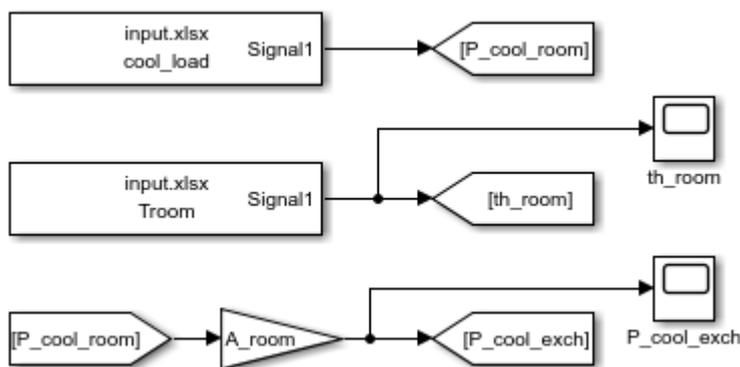
Figure B-8-2. Input of DesignBuilder simulation data from Excel file.
