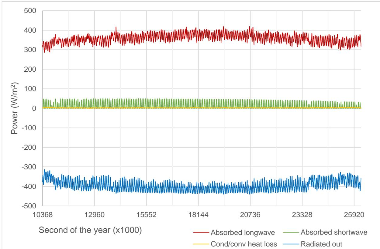
Figure 7-7. Contribution of each part to the total cooling load produced by the daytime cooler at each moment for the base-case scenario.
