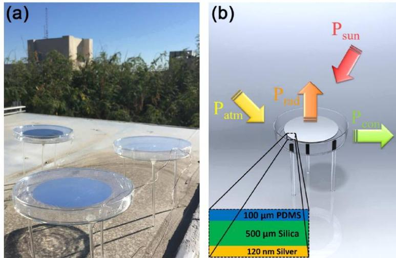
Figure 2-10. (Left) The radiative cooling samples designed by Kou *et al.* (2017); (Right) Schematic of the experiment setup.
