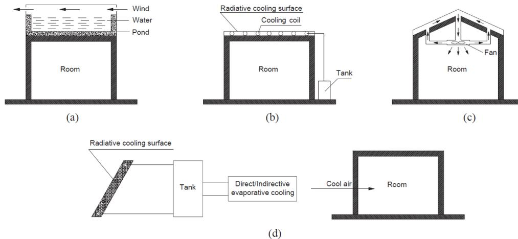
Figure 3-1. Active systems utilizing the heat gains of nocturnal radiative cooling: (a) Open loop water based system; (b) Closed loop water based system; (c) Air based system; (d) Hybrid system.
