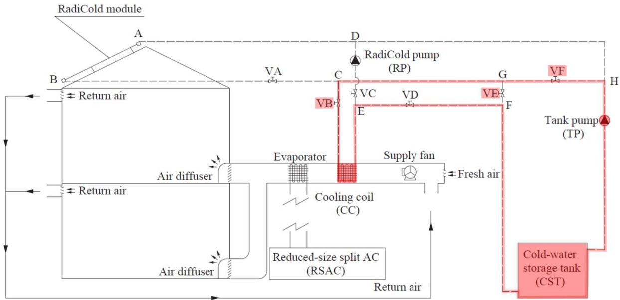
Figure 3-6. Third operation mode (Cold storage for space cooling) of the system of Zhang *et al.* (2018). Valves VB, VE and VF are open.
