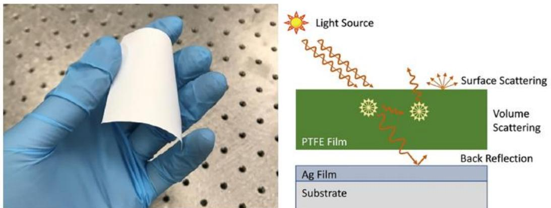
Figure 2-9. (Left) The PTFE sheet designed by Yang *et al.* (2018), without the sliver; (Right) Schematic representation of reflecting and scattering of the dual-layer structure.
