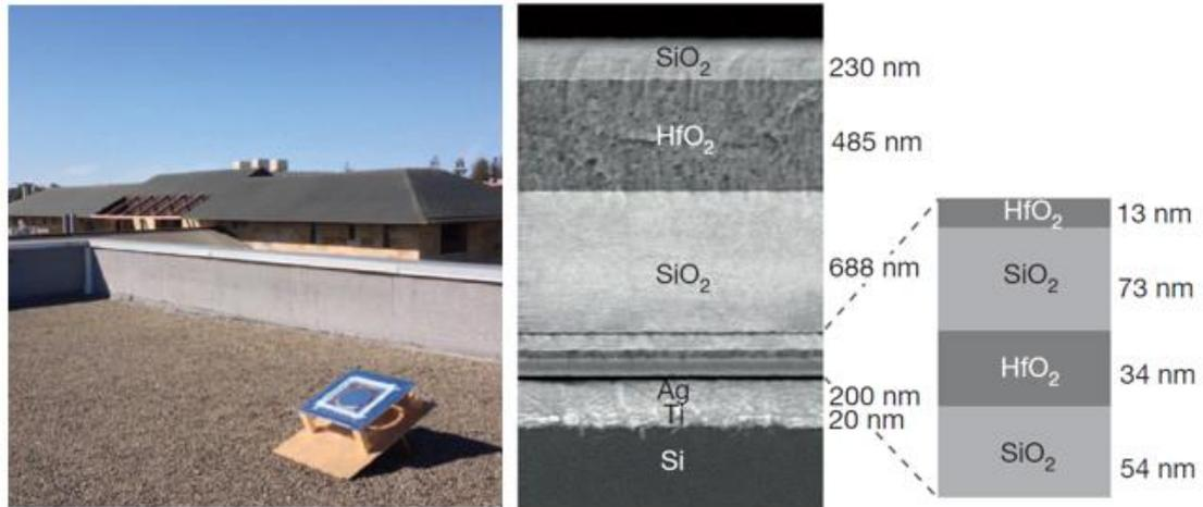
Figure 2-5. (Left) The radiative cooling structure designed by Raman *et al.* (2014); (Right) the layers of the solar reflector.
