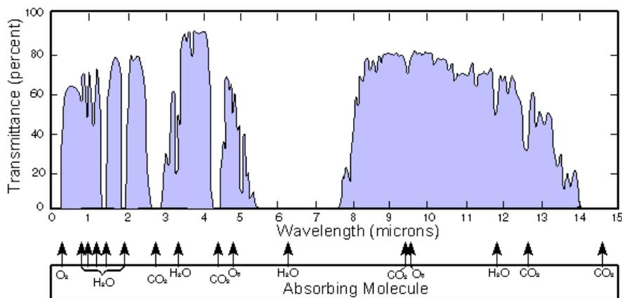
Figure 2-2. Transmittance of the atmosphere between 0 and 15  $\mu\text{m}$ . The atmospheric window can be seen between 8 and 13  $\mu\text{m}$  (Wikimedia Commons, 2014).
