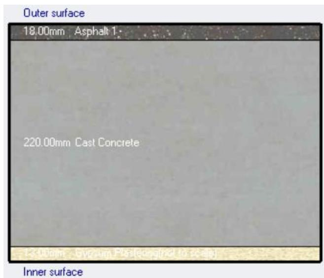
Figure 6-4. Cross-section of the flat roof structure, from DesignBuilder.
