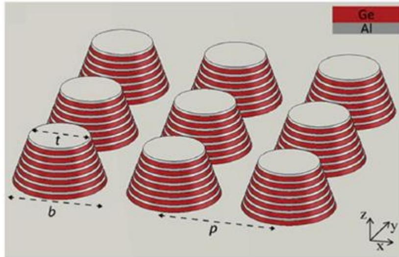
Figure 2-8. The multilayer metal-dielectric anisotropic microstructure introduced by Hossain *et al.* (2015).
