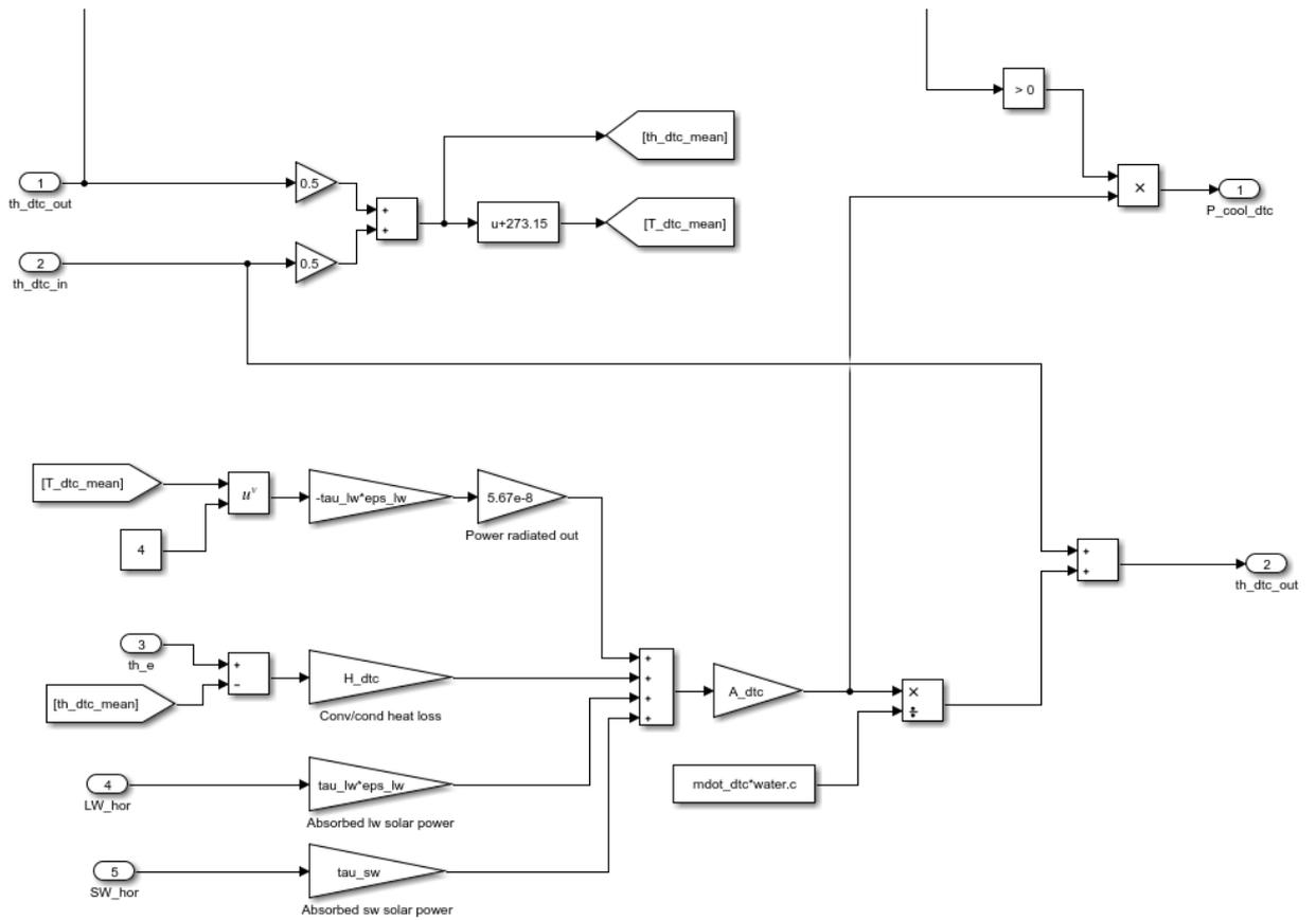
Figure B-8-6. Heat balance of the daytime radiative cooler.
