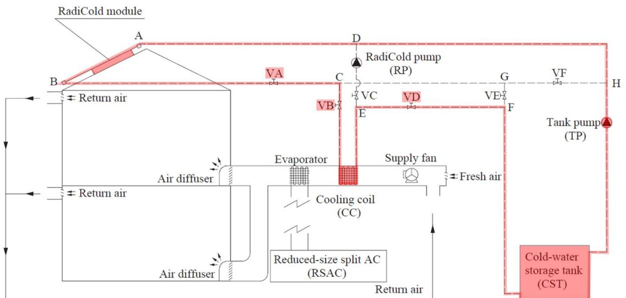
Figure 3-5. Second operation mode (Combined space cooling and cold storage charging) of the system of Zhang *et al.* (2018). Valves VA, VB and VD are open.
