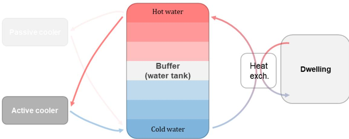
Figure 5-3. Mode 3 of the proposed system; when the active cooler covers the cooling demand.
