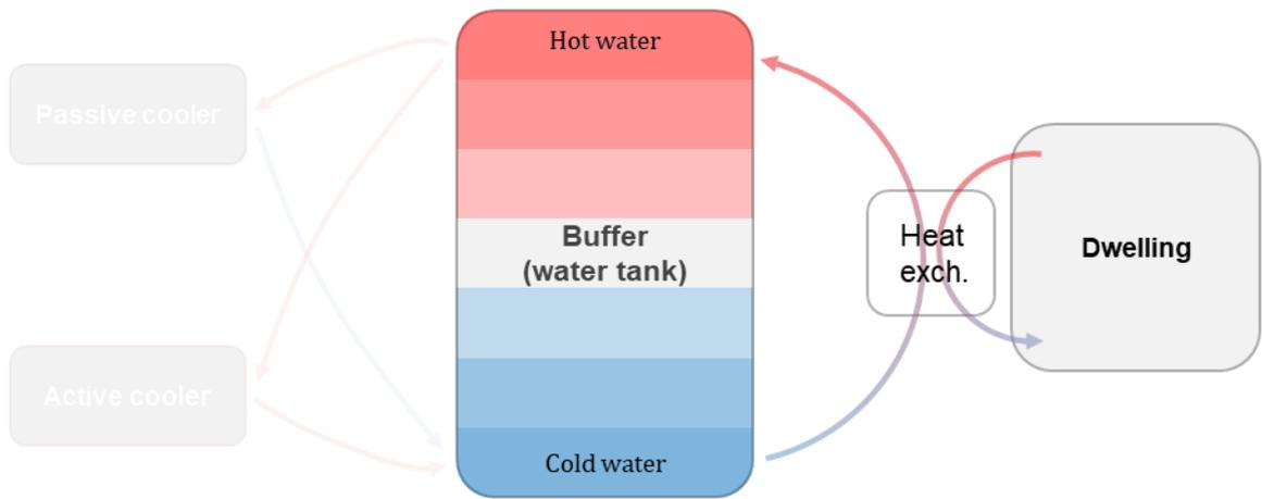
Figure 5-4. Mode 4 of the proposed system; when the energy stored in the water tank is enough to cover the dwelling cooling demand.
