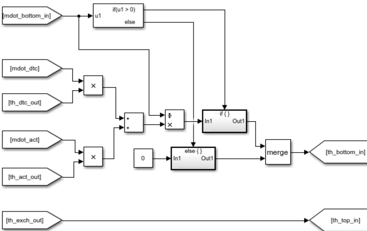
Figure B-8-5. Temperature of flows towards the buffer tank.
