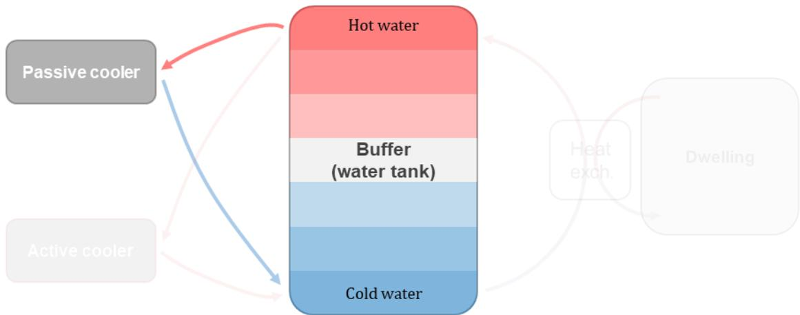
Figure 5-5. Mode 5 of the proposed system; when the energy supply from the passive cooler is used to only charge the water tank.
