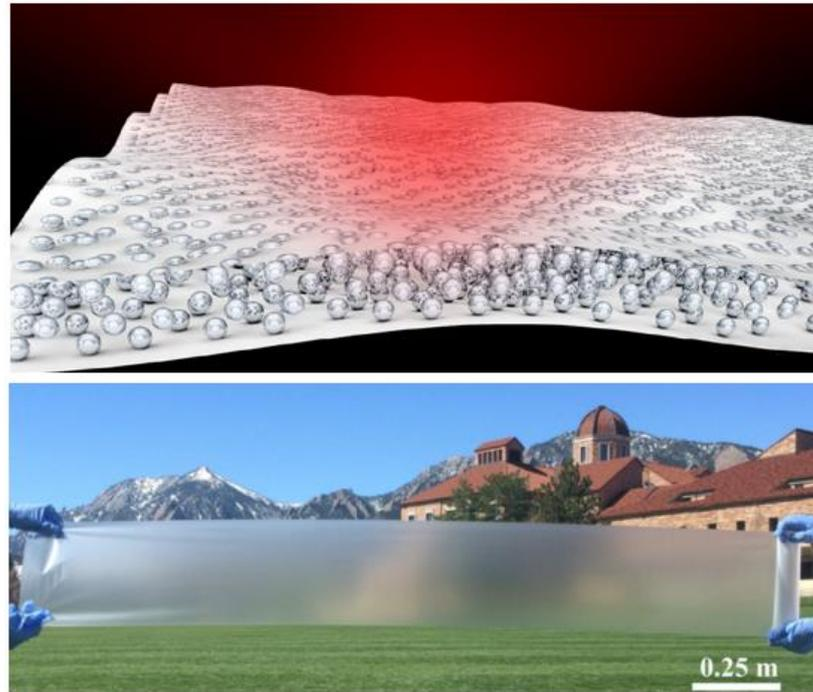
Figure 2-11. (Top) Schematic of the glass-polymer hybrid metamaterial as proposed by Zhai *et al.* (2017); (Bottom) A photo showing the metamaterial film, before being coated with silver.
