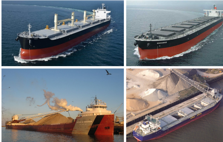
Figure E.3: Basic, gearless, lake and self-unloading bulk carrier respectively [160], [161], [162], [163]
