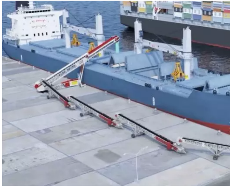
Figure 5.37: Mobile belt conveyors used for the shortcut [89]
