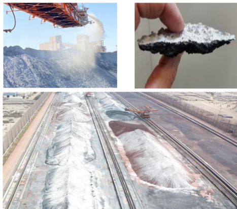
Figure 2.4: Cellulose crust on stockpile [44]
