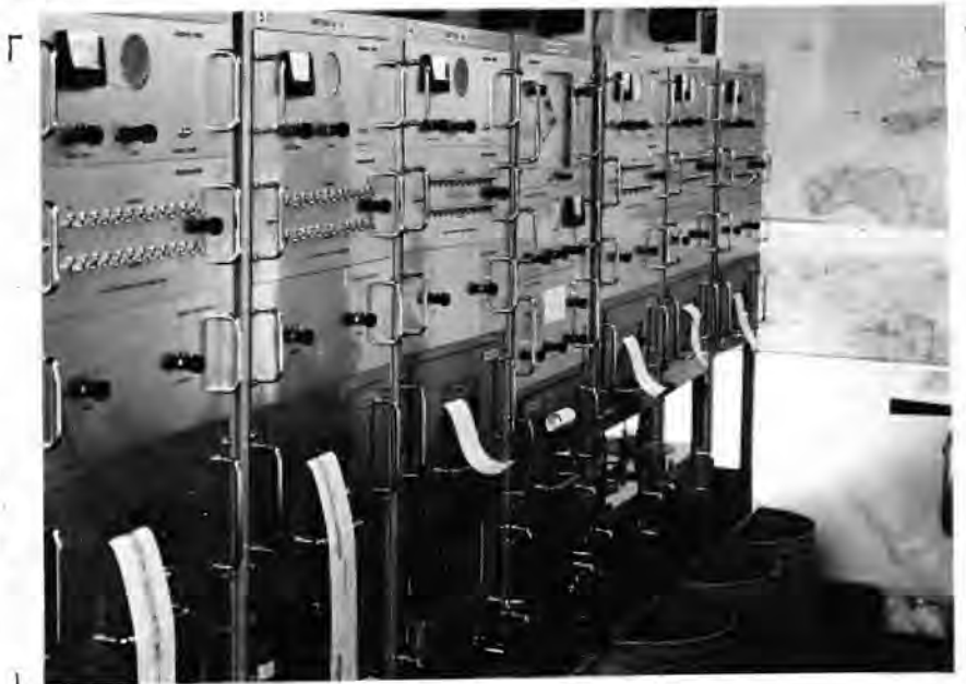
Photo 1 - Wave height registration apparatus in the central recording office at Hellevoetsluis.
