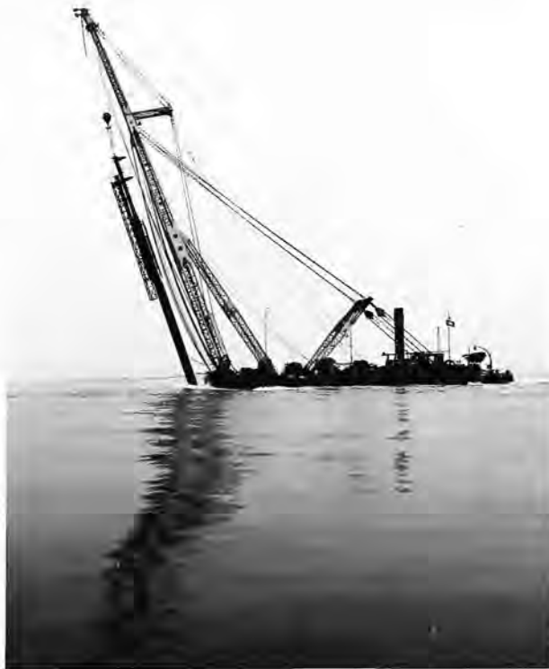
Photo 3 - Transport of staff-gauge by floating crane.
