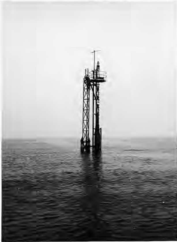
Photo 5 - The staff-gauge in place.
