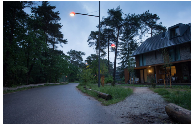
LED street lights to limit energy use and to dim for fauna
