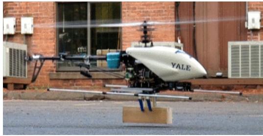
(a) Example of flying hand aerial manipulator, source: [5].
